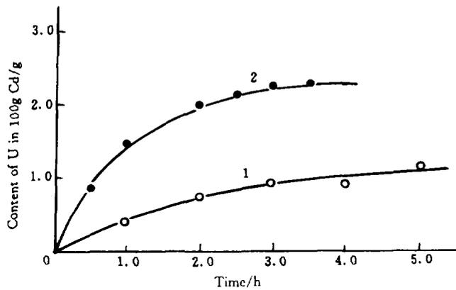
Fig. 5 Effect of stirring on dissolution of uranium (Temperature 500°C, others are same as that in Fig. 2.)
