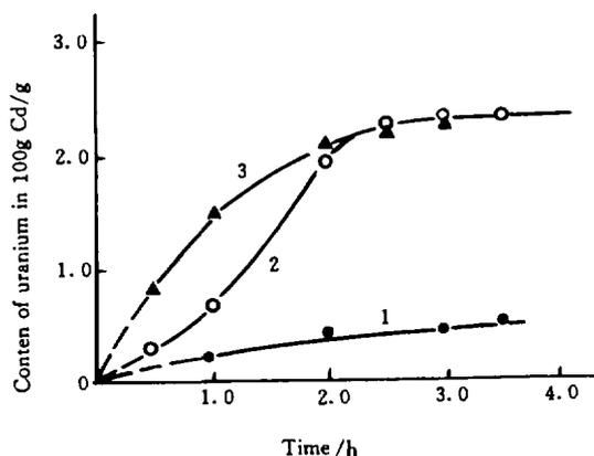
Fig. 2 Effect of time and temperature on dissolution of uranium
