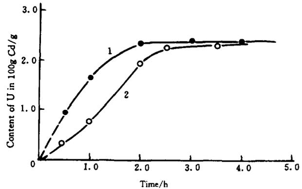
Fig. 4 Effect of total surface area of U-10Zr alloy pellet on dissolution of uranium (Temperature 475°C, others are same as that in Fig. 2.)
