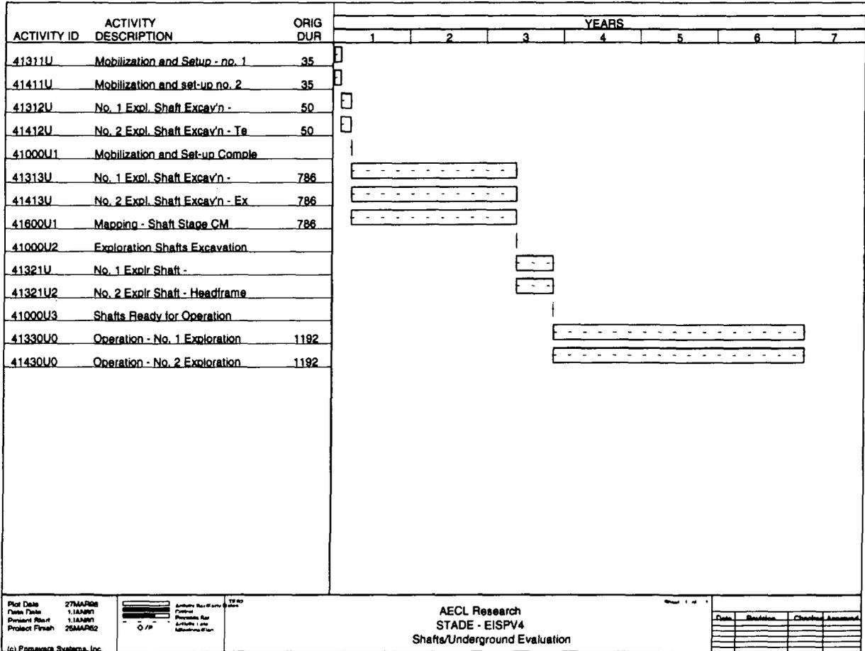
FIGURE 5: An Example Activity Gantt Chart. This figure is designed to show only the shaft-related activities during the Underground Evaluation stage. The activities are selected from the activity-based system by identifying the appropriate codes.
