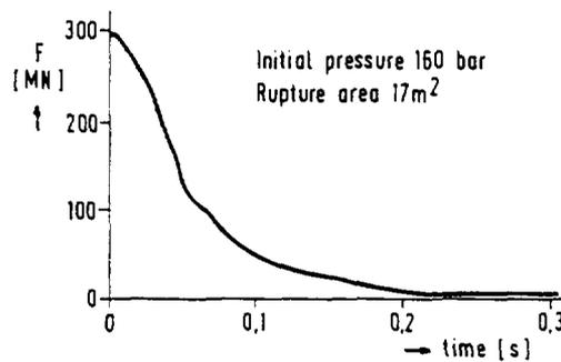
Fig. 4: Force  $F$  acting at the reactor vessel after a melt through failure under high internal pressure; figure taken from [9].
