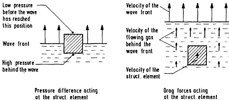
Fig. 5: Structural elements which are not properly fixed may be accelerated by passing pressure waves caused by hydrogen explosion.
