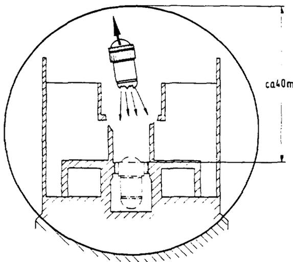
Fig. 3: The whole reactor vessel might be hurled against the containment shell as a consequence of a melt through failure under high internal pressure. This event must not occur.
