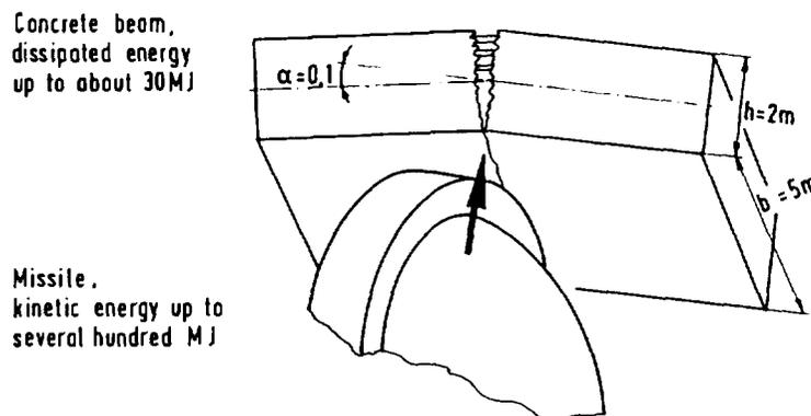
Fig. 2: The energy which can be dissipated by the protective structure is much smaller than the energy of missiles caused by a steam explosion
