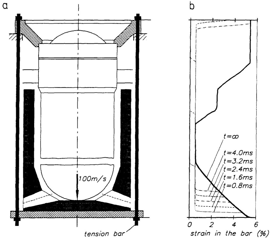
Fig. 8: The missile retention device forms a closed system
