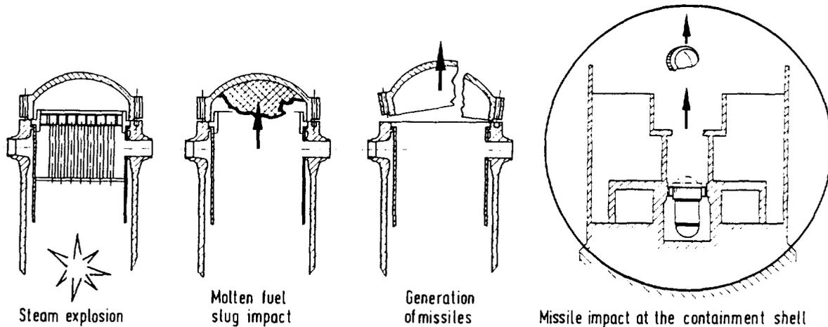
Fig. 1: Heavy fragments of the pressure vessel might be hurled against the containment shell as a consequence of a steam explosion. It must be shown that this event does not occur.
