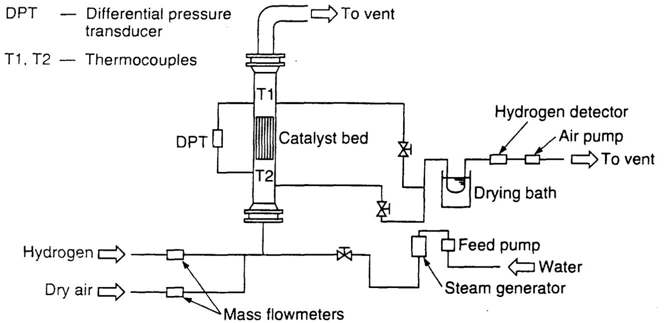
**FIGURE 1:** Schematic of an Apparatus for Testing the Performance of Cylindrical Catalyst Elements in  $H_2$ -Air-Steam Under Forced Convection
