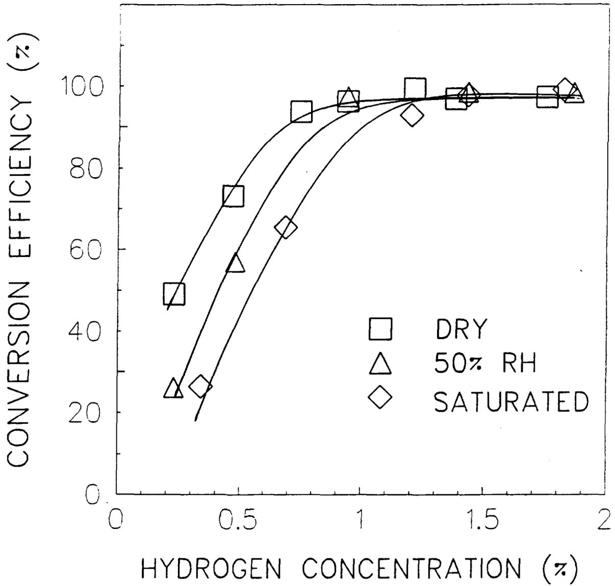
FIGURE 5: Effect of Humidity on Self-Start Under Forced Convection (200 mm-deep element with a 3 m/s flow velocity)
