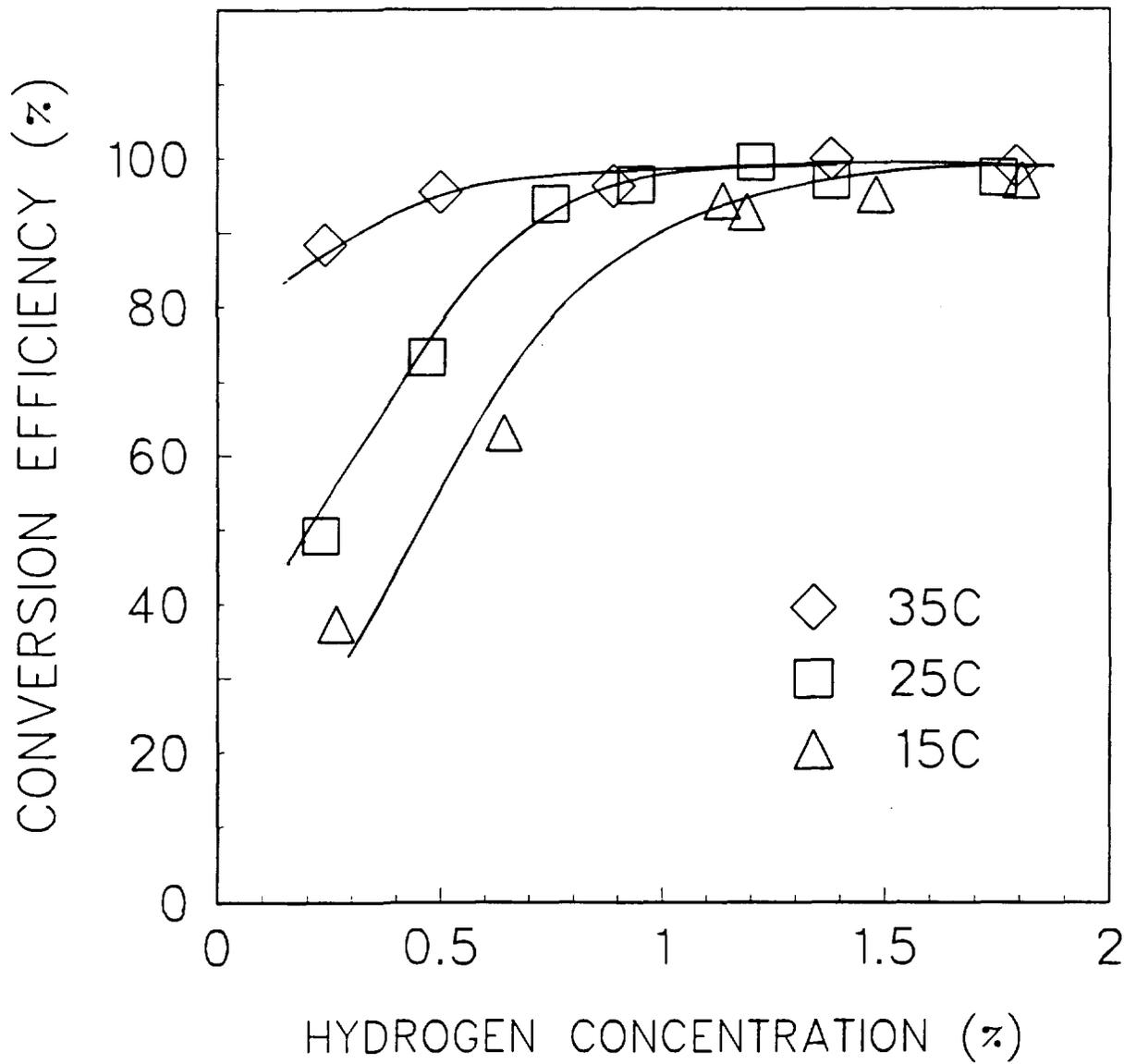
FIGURE 4: Effect of Inlet Gas Temperature on Conversion Efficiency Under Forced Convection (200 mm-deep element, 3 m/s flow velocity)
