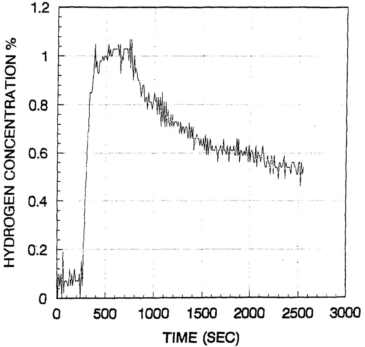
FIGURE 7: Example of Passive Self-Start of Catalytic Recombiner in 1% H<sub>2</sub> at 25°C, 100% R.H. Recombiner opened at 750 s.
