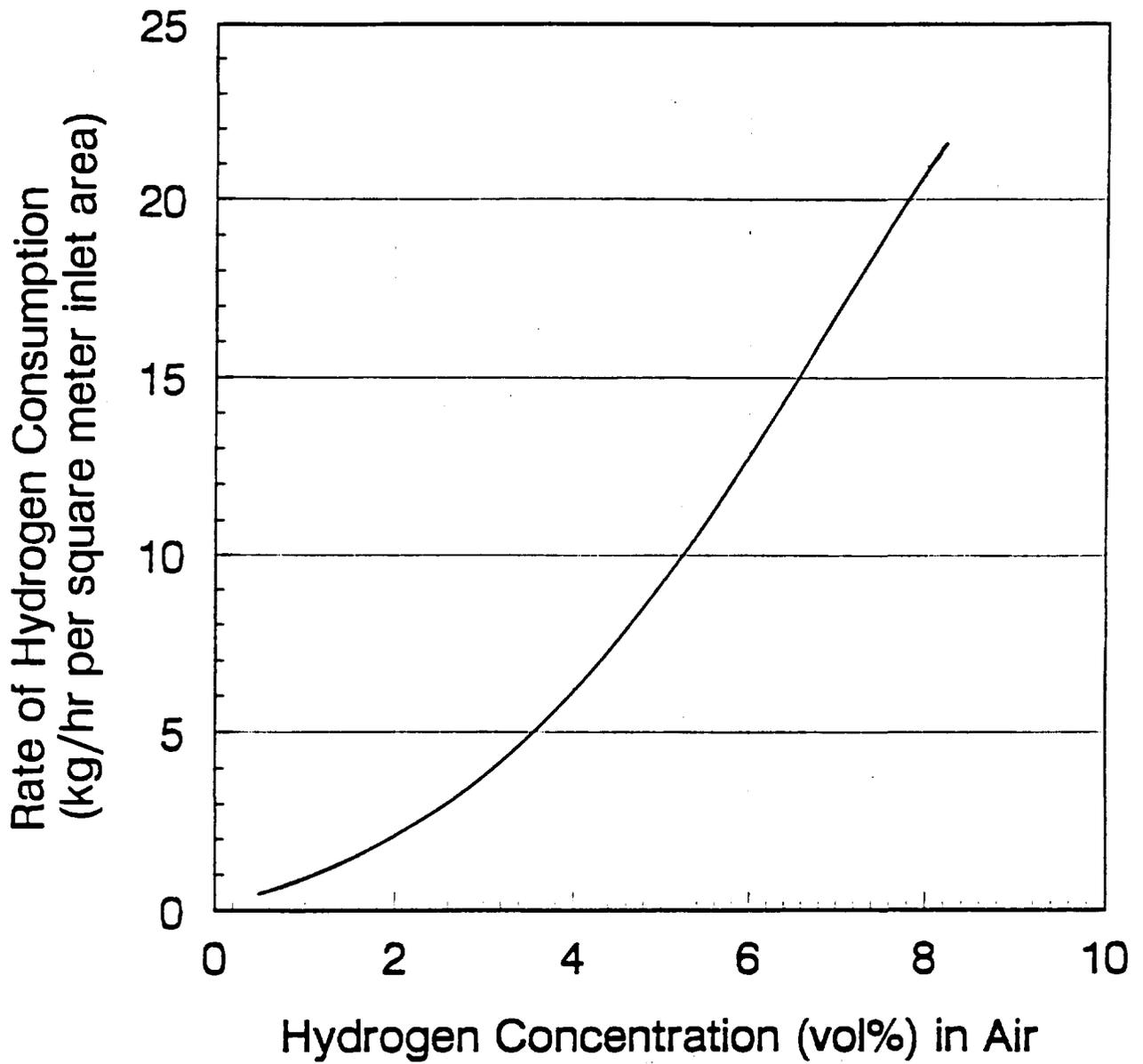
FIGURE 8: Typical Capacity of AECL Catalytic Recombiner Operating in Natural Convection (passive) Mode. Inlet conditions 100 kPa (abs), 25°C, 100% R.H.
