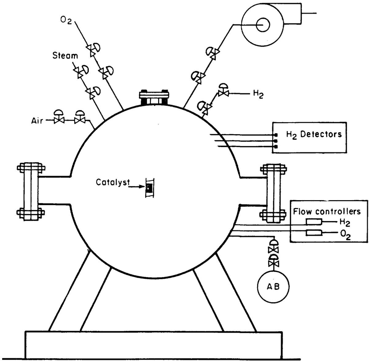
FIGURE 6: The 6.6 m<sup>3</sup> Containment Test Facility (CTF), Configured for Hydrogen Recombiner Tests
