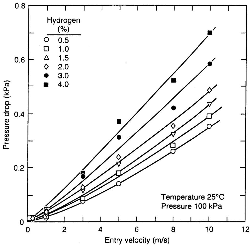
FIGURE 3: Pressure Drop with Forced Convection Across a Catalyst Element with 80% Efficiency for Hydrogen Removal
