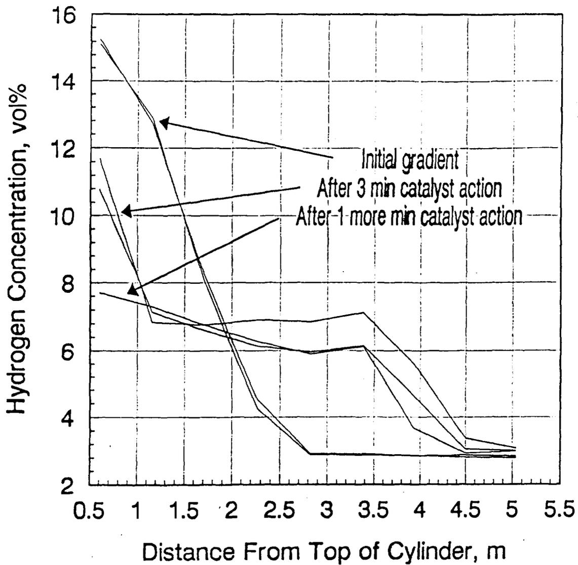
FIGURE 10: Typical Mixing Behaviour in Stratified Mixtures with Catalytic Recombiner Arranged Approximately 1 m from the Bottom as Shown in Figure 9
