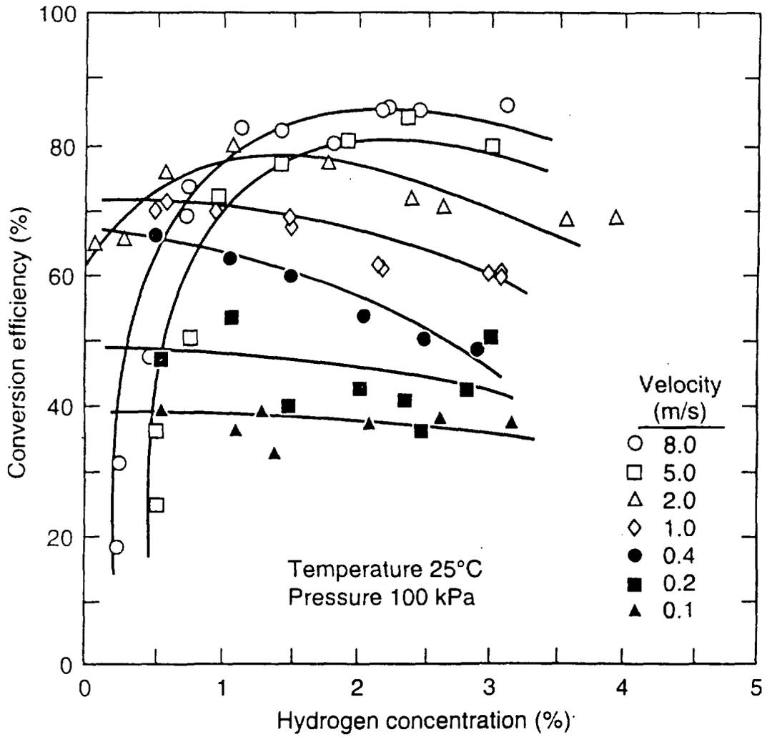
FIGURE 2: Hydrogen Recombination Efficiency of a 100 mm-Deep Catalyst Element Under Forced Convection
