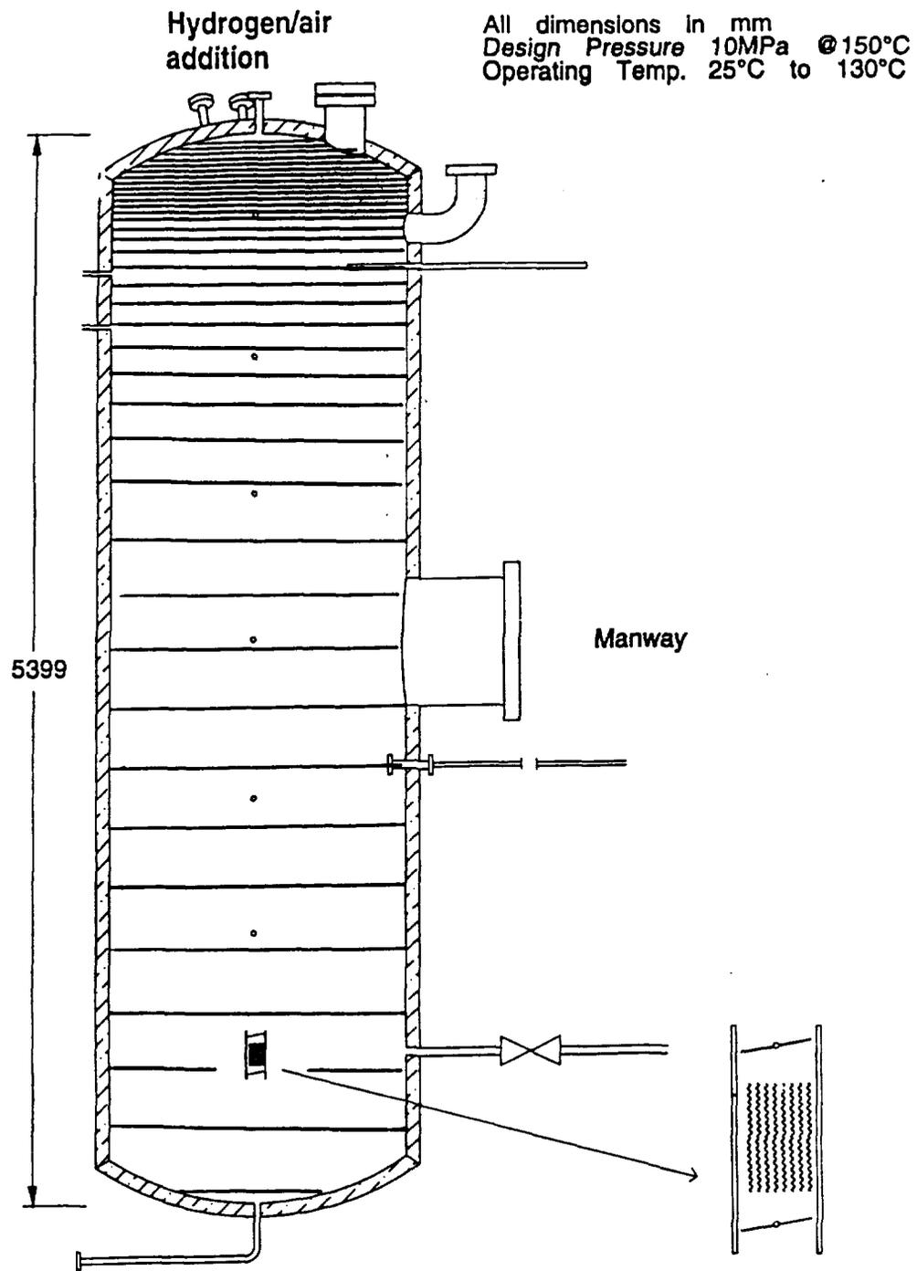
**FIGURE 9:** The 10.7 m<sup>3</sup> CTF Cylinder Configured for Testing Catalytic Recombiner Performance in Stratified Mixtures
