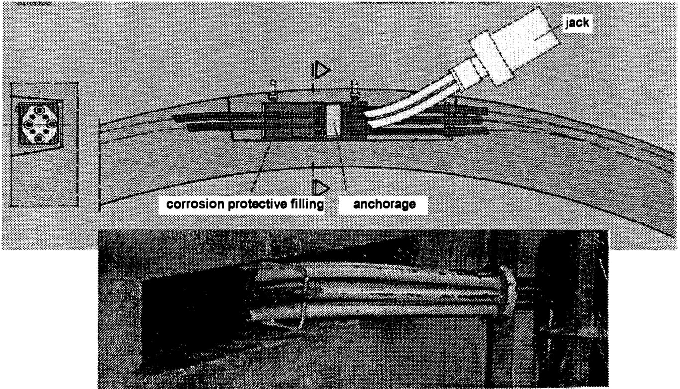
Fig. 8 Monostrand post-tensioning system of DYWIDAG
