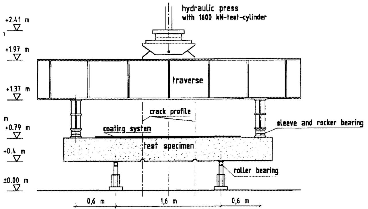
**Fig. 3 Composite liner test installation**
