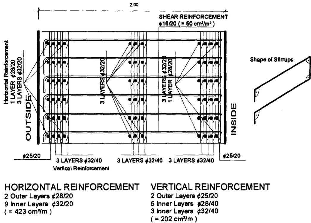
**Fig. 2 Typical arrangement of reinforcement at the cylindrical part**
