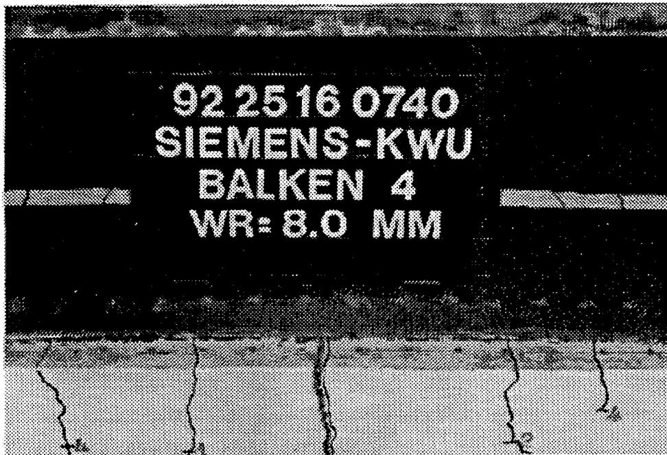
**Fig. 5 Composite liner during test - crack width of 8 mm without failure**
