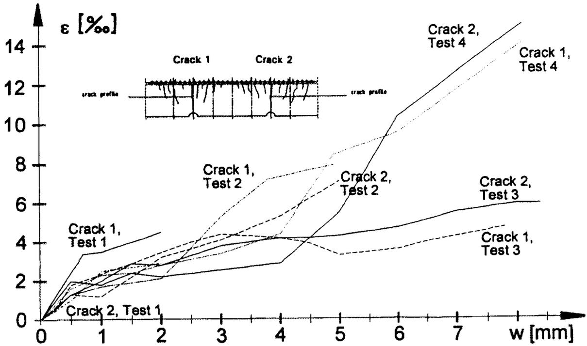
Fig. 7 Strain in the composite liner as a function of crack width
