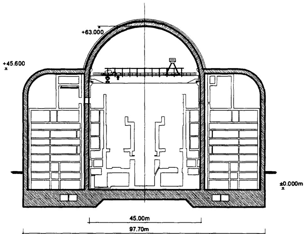
**Fig. 1 Arrangement of the combined reinforced concrete containment**
