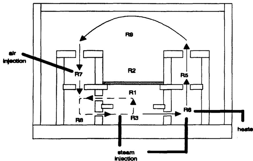
Fig. 2: Natural circulation flows during FIPLOC F2 test.
