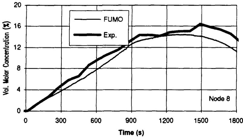
Fig. 10: Hydrogen concentration in the blow-down node.
