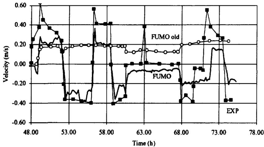
Fig. 3: Natural circulation velocity through junction from R6 to R3.
