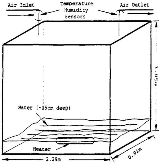
Figure 5. Test Geometry for Evaporative Heat Transfer Tests.
