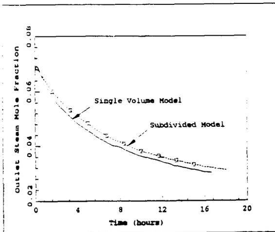
Figure 10. Lumped Versus Subdivided Results for Outlet Steam Mole Fraction.
