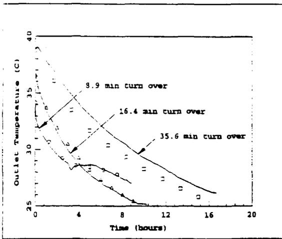
Figure 6. Grout Mold Outlet Temperatures.
