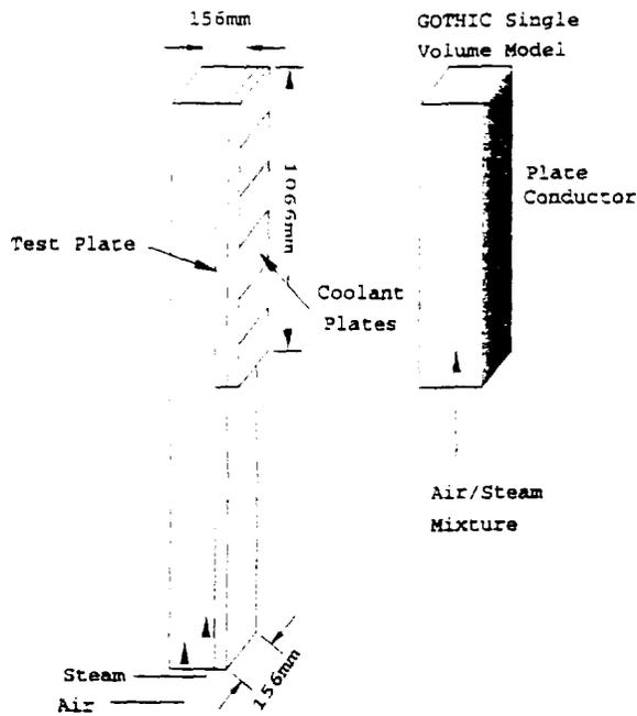
Figure 1. Test Section and GOTHIC Model for Condensation Tests.
