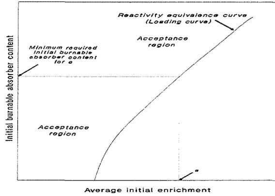
FIG. 2. Reactivity equivalence concept applied to wet storage of BWR fuel assemblies having attained their maximum reactivity.
