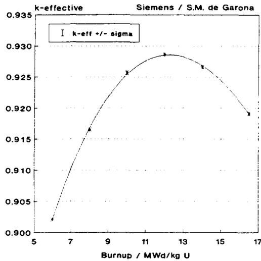
FIG. 4. Illustration of estimating the neutron multiplication as a function of the initial burnable absorber content: The maximum of the curve representing the neutron multiplication as a function of burnup provides one of the  $k_{eff} \pm \sigma$  bars shown in Fig. 3.
