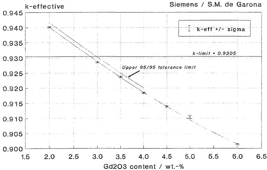
FIG. 3. Illustration of estimating the loading curve shown in Figure 2: The intersection of the upper 95%/95% tolerance limit of the neutron multiplication as a function of the initial burnable absorber content with the maximum permissible neutron multiplication  $k_{\text{limit}}$  provides one point of the loading curve Fig. 2.
