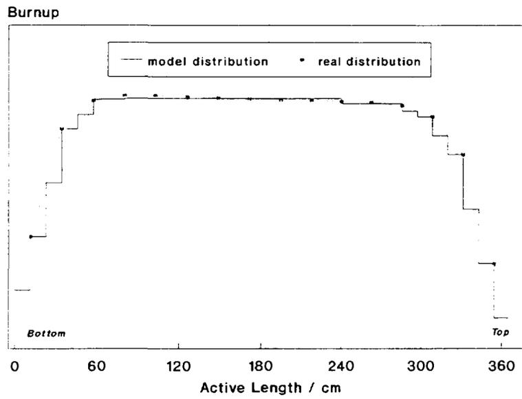
FIG. 5. Typical PWR axial burnup distribution
