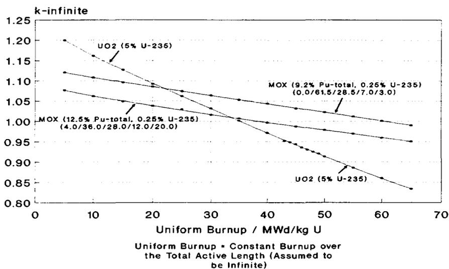
FIG. 1. Neutron multiplication of a wet storage system for loadings with spent PWR UO<sub>2</sub> fuel assemblies having an initial enrichment of 5 wt.% <sup>235</sup>U and loadings with spent PWR MOX fuel assemblies having different total plutonium contents and different isotopic vectors.
