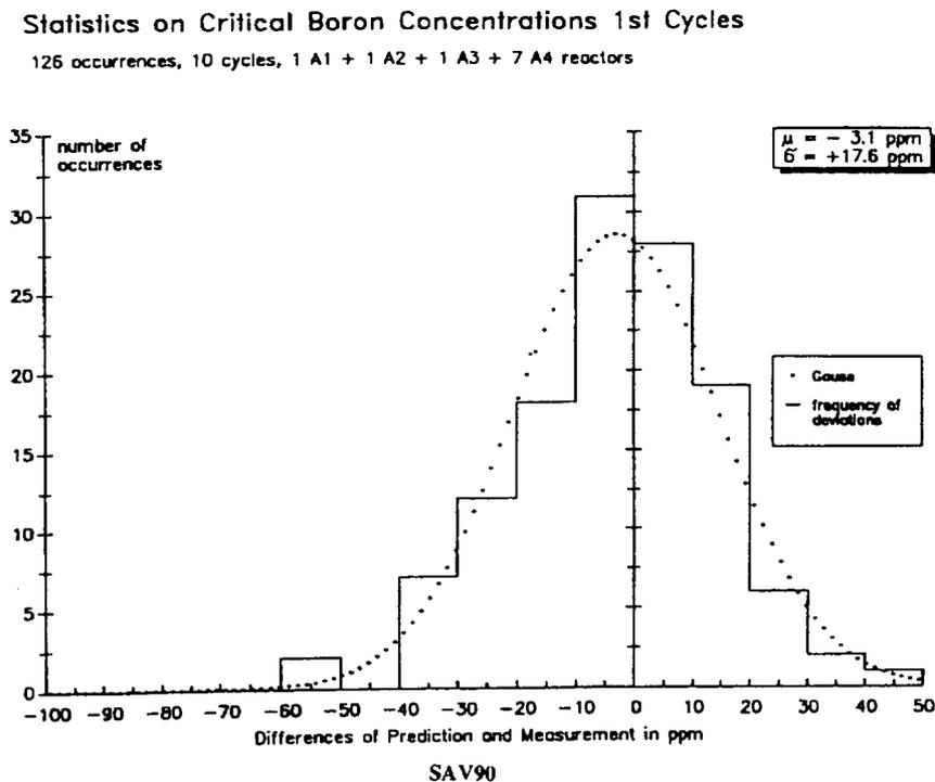
FIG. 8. SAV90 statistics on critical boron concentrations.
