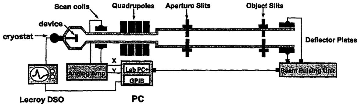
Figure 1: A schematic of the complete Transient-IBIC analysis system.
