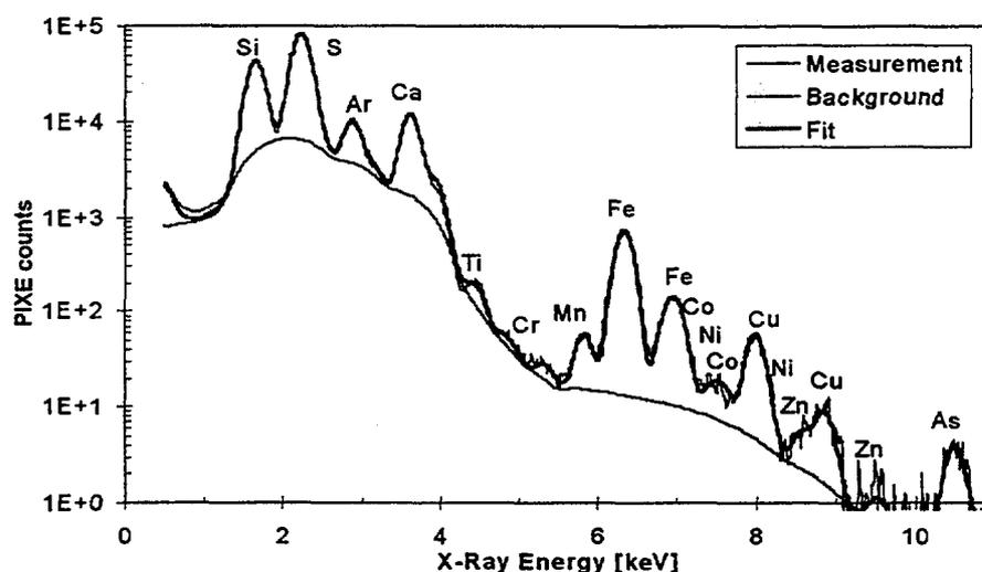
**Figure 3:** The high amount of Fe visible in the external PIXE spectrum of the blue Egyptian glass is the source for the blue colour of this Egyptian glass sample
