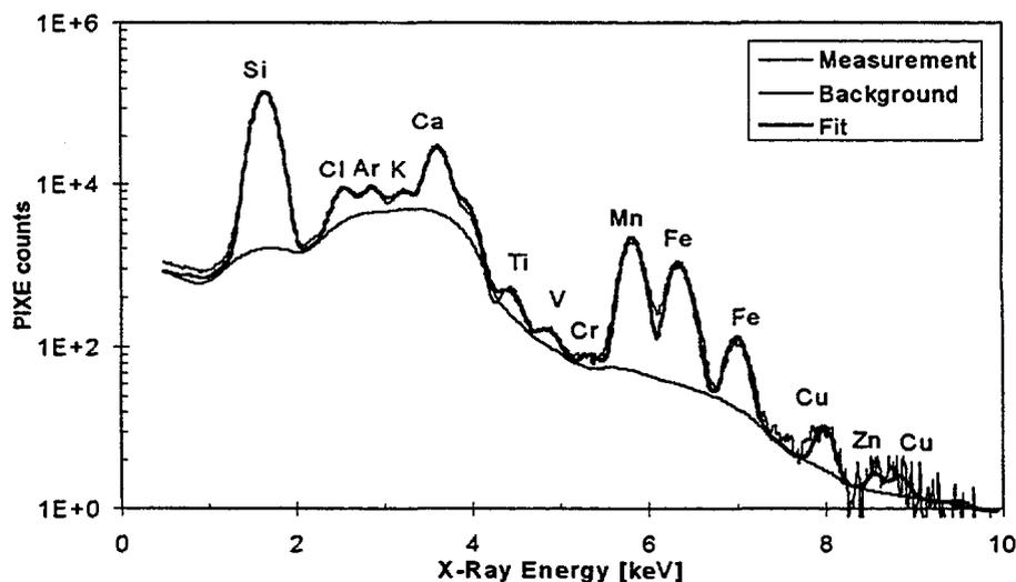
Figure 2: External PIXE spectrum of the red Egyptian glass displaying the high concentration of Mn and Fe causing the light red colour.
