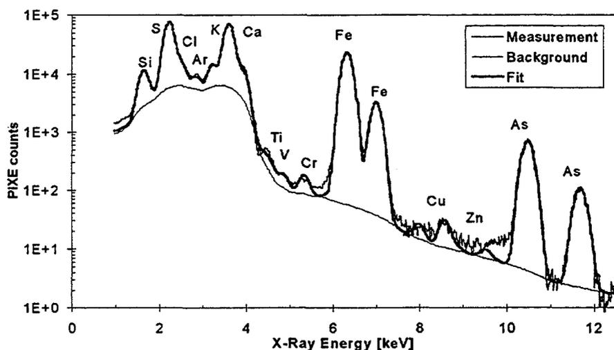
Figure 1: External PIXE spectrum from the wall paint with clearly visible As peaks.
