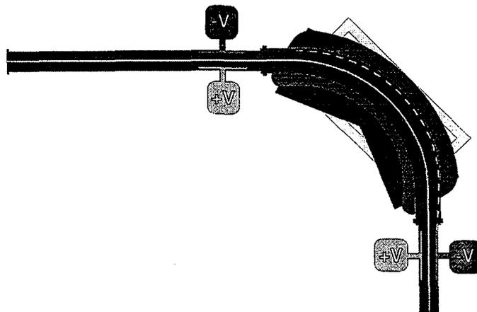
Figure 1. The fast bouncing system at the high energy end consists of pairs of deflector plates at the entrance and at the exit of the high energy magnet, deflecting the beam in the plane of orbit. The voltages are identical for the two sets of plates.
