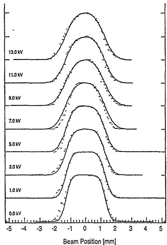
Figure 3. The beam profile remains flat over a significant range of deflection and deteriorates at higher deflection, accompanied by a decrease in transmission.
