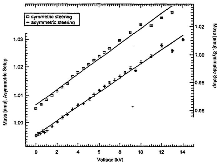
Figure 2. Test of the deflector plates with 3 MeV protons. The proton beam energy variation has been translated into the equivalent mass for a 3 MeV beam. Both the symmetric mode, where the voltages on the pair of plates are equal but opposite, and the anti-symmetric mode, where one of the plates is grounded, give linear response.
