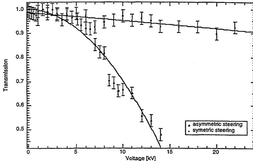
Figure 4. The transmission efficiency for the symmetric mode remains flat for a significant range of deflection voltage. The more rapid drop in the asymmetric mode reflects the lens effect.
