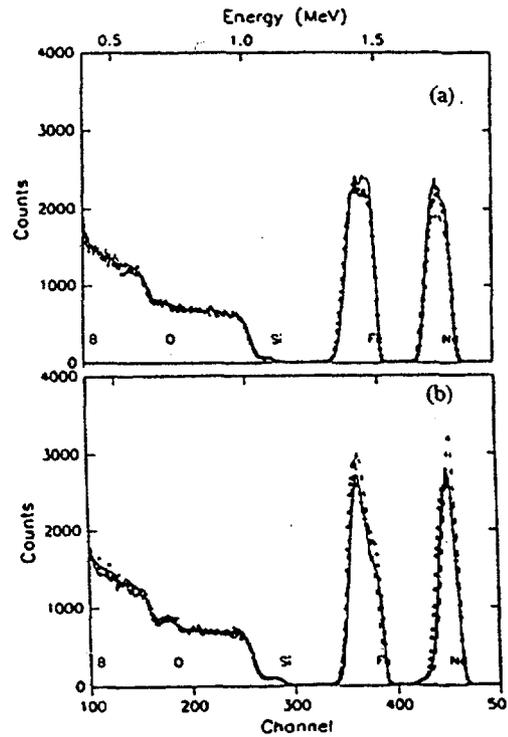
Fig.3. RBS spectra of films deposited on silicon with SiO<sub>2</sub> barrier layer at R.T (—), 360°C (·), 440°C (--) and annealed at (a) 600°C and (b) 800°C
