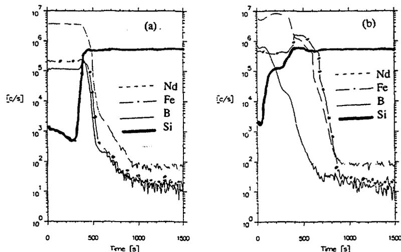
Fig.1. SIMS spectra of films deposited at (a) R.T (b) 440°C
