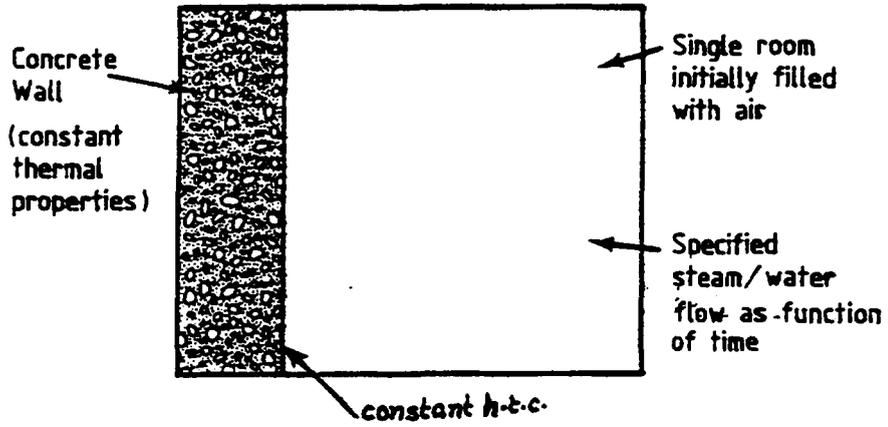
Fig. 6: CSNI Numerical Benchmark Test Model
