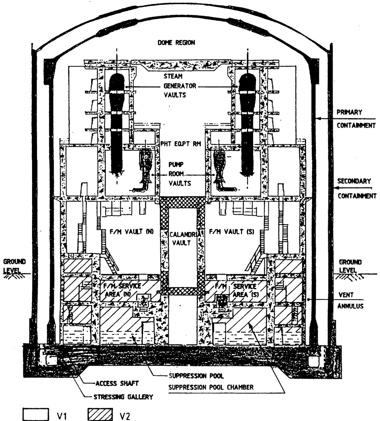
Fig.1: Typical Cross-Section of 220 MWe Indian PHWR Containment Building
