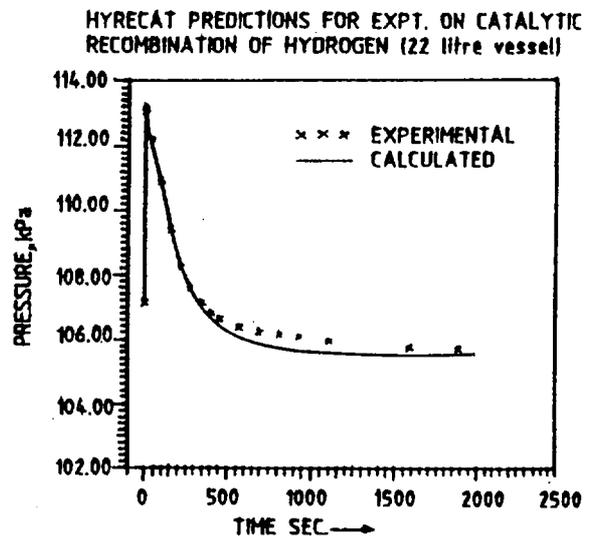
Fig. 10: Comparison of HYRECAT Predictions with experimental data on Laboratory Scale Test.
