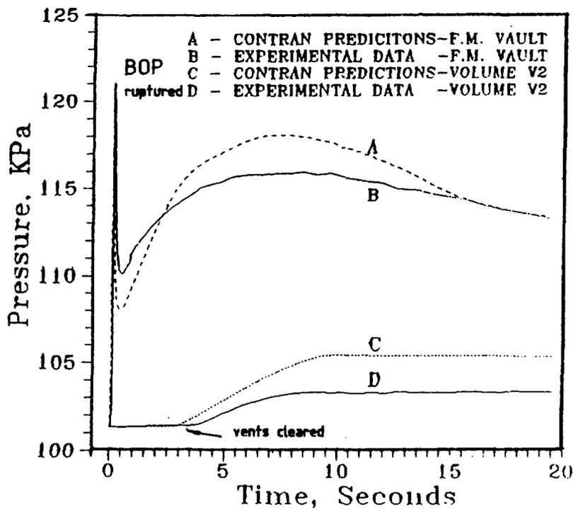
Fig. 3: Pressure Transients in V1 and V2 for Test M4L0 in One-Tenth Scale Vapour Suppression pool Containment Experimental Facility
