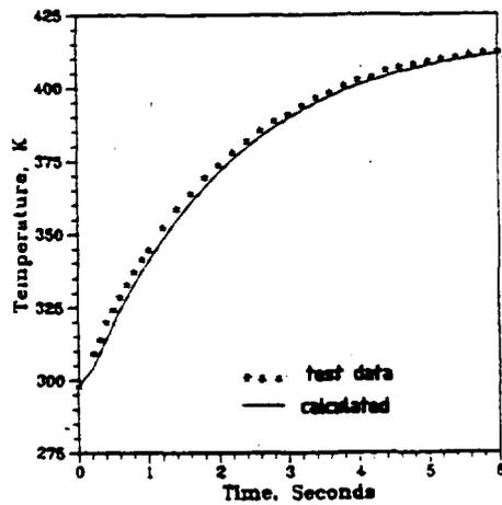
Fig. 7c: Wall Surface Temperature of Containment of CSNI Benchmark Test Model
