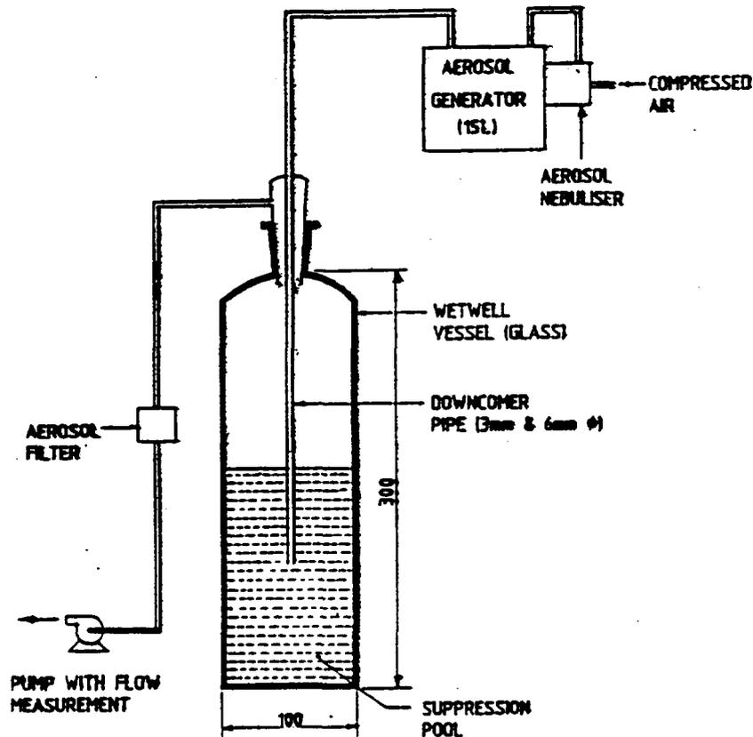
Fig. 14: Suppression pool Aerosol Scrubbing Test Facility (schematic)
