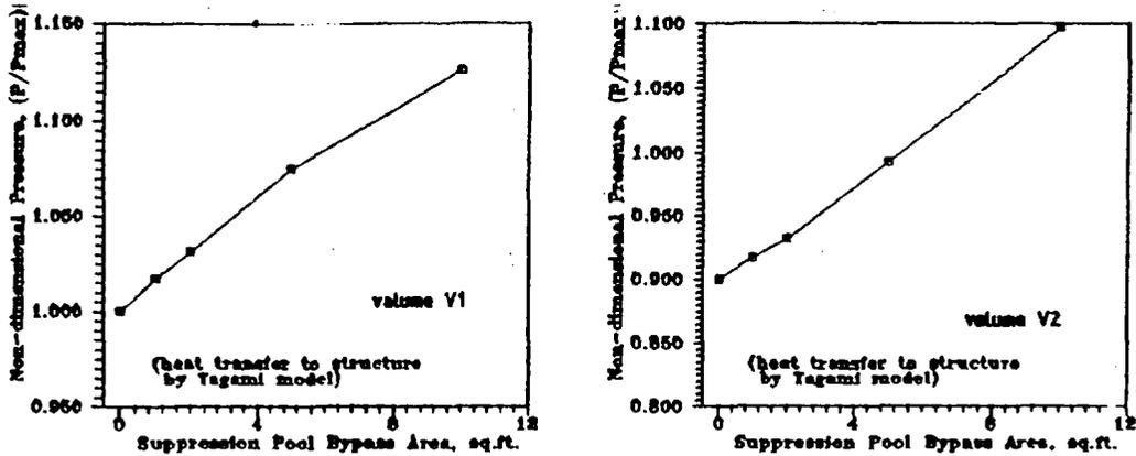
Fig. 8a: Variation of Containment Peak Pressure with Suppression Pool Bypass Area following MSLBA in 220 MWe Indian PHWR
