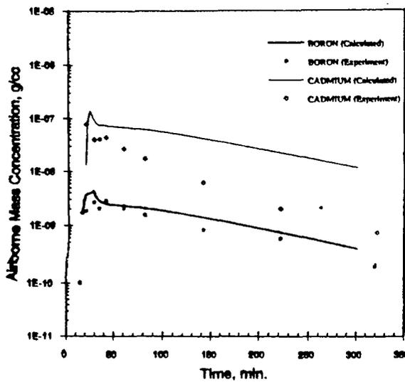
Fig. 13a: Boron and Cadmium airborne mass concentrations in containment
