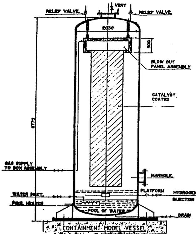
Fig. 9: Experimental Setup for Hydrogen Mitigation Studies using catalytic Recombination
