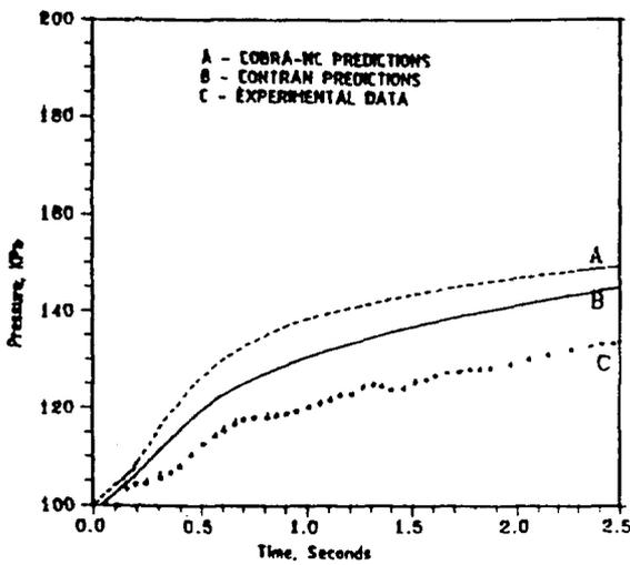
Fig. 5d: Pressure Transients in Room R4 for BFC Test D-15.
