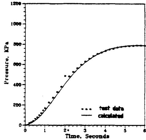
Fig. 7b: Steam Pressure in Containment of CSNI Benchmark Test Model
