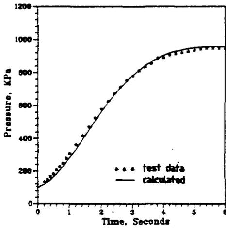
Fig. 7a: Total Pressure in Containment of CSNI Benchmark Test Model
