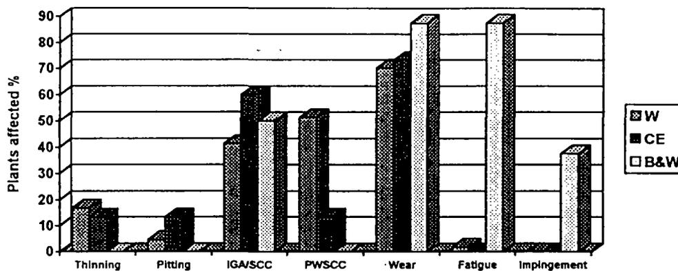
Figure 2. Tube degradation in PWR steam generators
