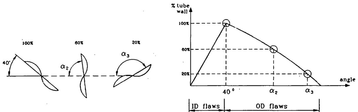
Figure 3. Determining the depth of detected indication
