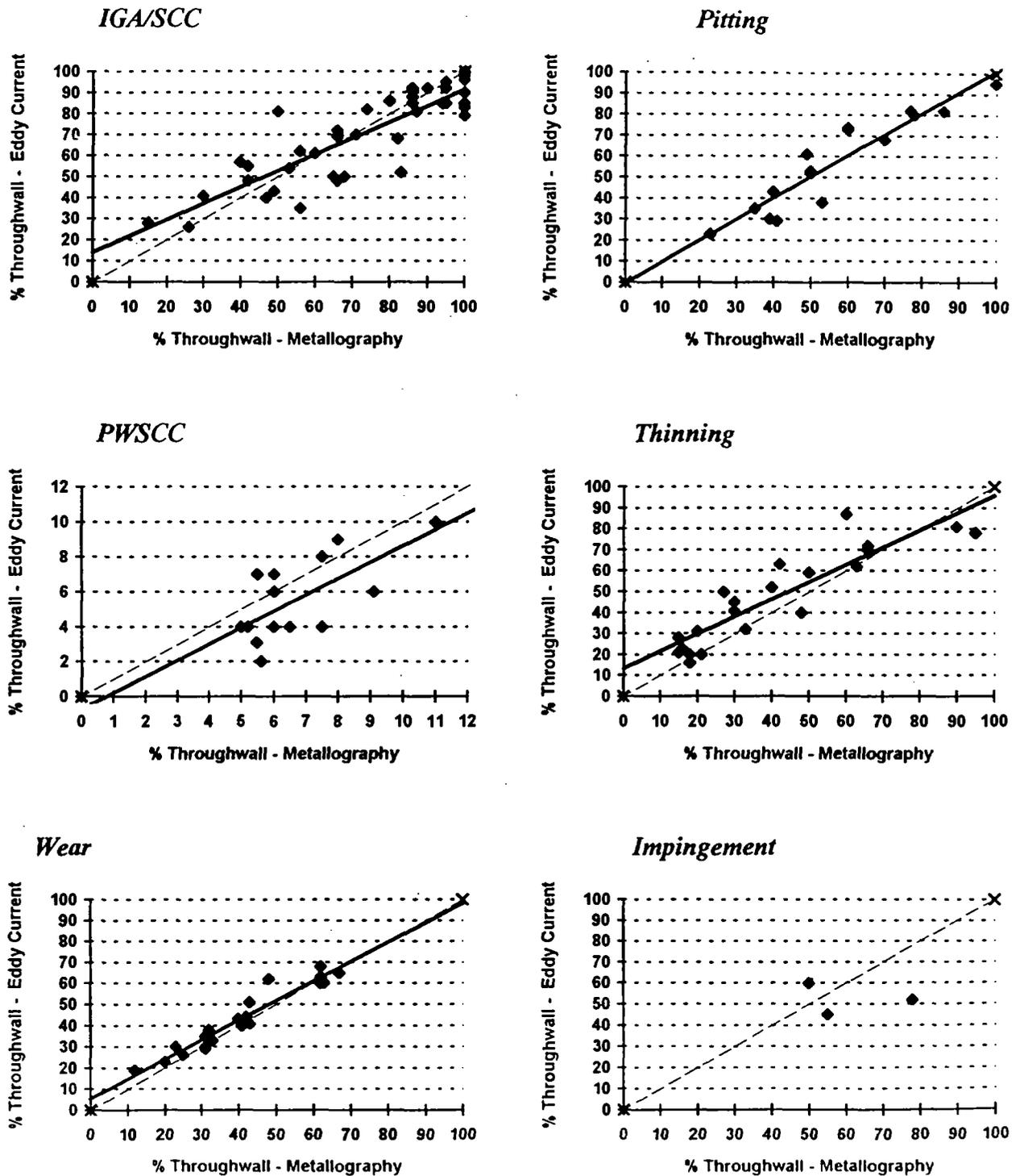
Figure 4 Eddy current accuracy for different degradation mechanisms
