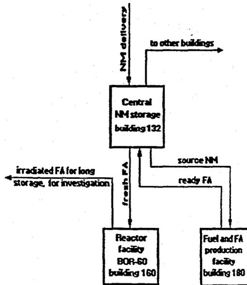
Fig. 2. Movement of Nuclear Material in RIAR Fast Reactor Fuel Cycle
