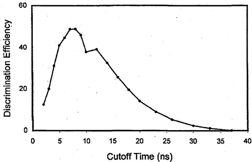
**Figure 3.2.** Graph Showing the Algorithmic Efficiency of the “Early Area” Method as a Function of the Cutoff Time Used. The optimum cutoff time is found to be 8.0 ns.
