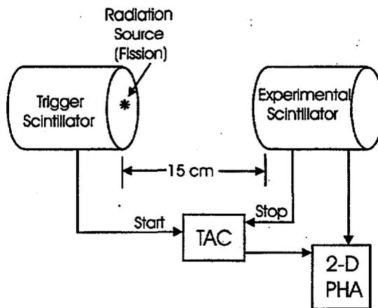
**Figure 4.1.** Schematic Drawing Showing the Time-of-Flight Technique Used To Label Pulses As Neutron or Gamma Ray Pulses Before Interaction in the Scintillator. This method allows assessment of the performance of a direct fast-neutron detector.
