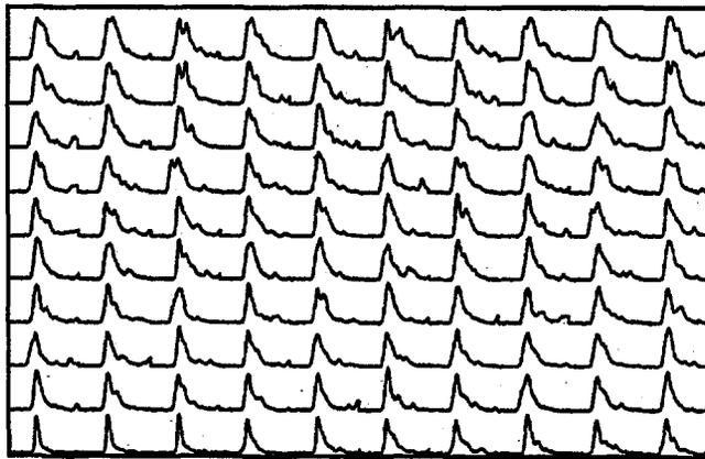
**Figure 4.4.** Plot Showing 100 Experimentally Acquired Gamma Ray Pulses. The average width for this set is roughly 3.3 ns.
