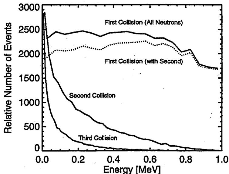
**Figure 2.1.** Histogram of the Distribution of Neutron-Recoil Energy Loss for Four Different Sets of Neutron Recoil Events Arising During the Interaction of 50,000 Neutrons. The sets are comprised of all first collisions, all second collisions, all third collisions, and those first collisions that are followed by a second collision. The second and third collision curves are vertically scaled to fit the plot, but the two sets of first collision data can be quantitatively compared.
