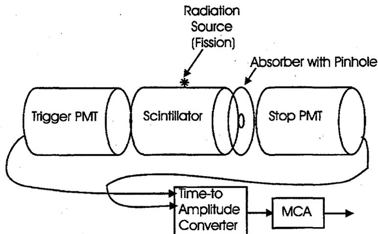
Figure 6.1. Schematic Diagram Showing the Technique Used To Acquire "Single Photon Test" Data
