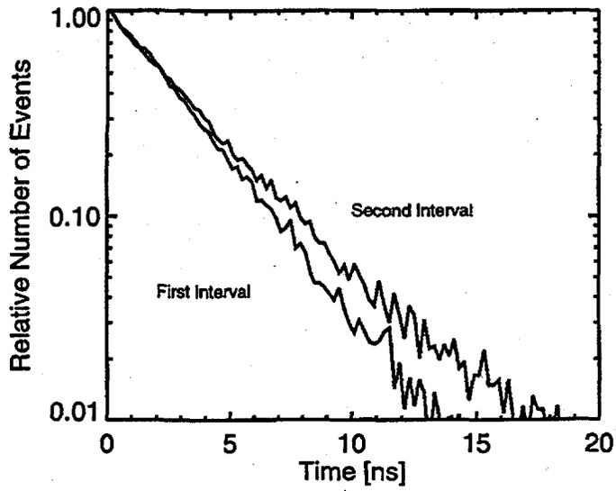
**Figure 2.2.** Histogram Showing the Distribution of Time Intervals Between the First and Second Recoils and Between the Second and Third Recoils
