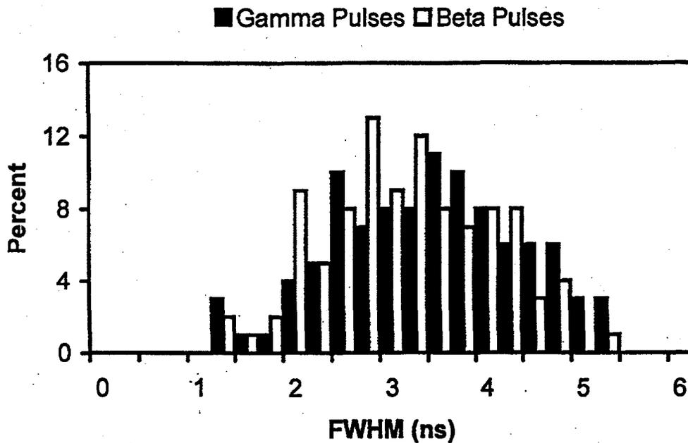
Figure 4.9. Plot Showing Width Spectra for Sets of Pulses Acquired Using Beta and Gamma Radiation, Respectively
