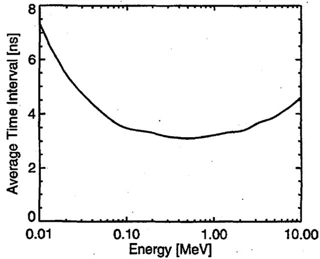
**Figure 2.3.** Plot Showing the Theoretically Expected Average Time Interval Between Hydrogen Recoils As a Function of Neutron Energy
