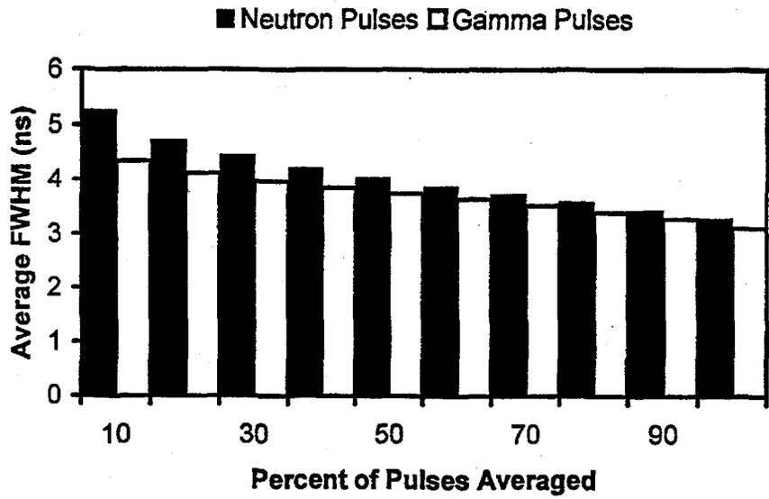
**Figure 4.3.** Plot comparing the averaged width of various subsets of Experimentally Acquired Sets of 100 Neutron and 100 Gamma Ray Pulses. The pulses were sorted by width before selecting the fractional subsets. For example, the first data point shows the average width of the widest 10% of the neutron and gamma ray pulses.
