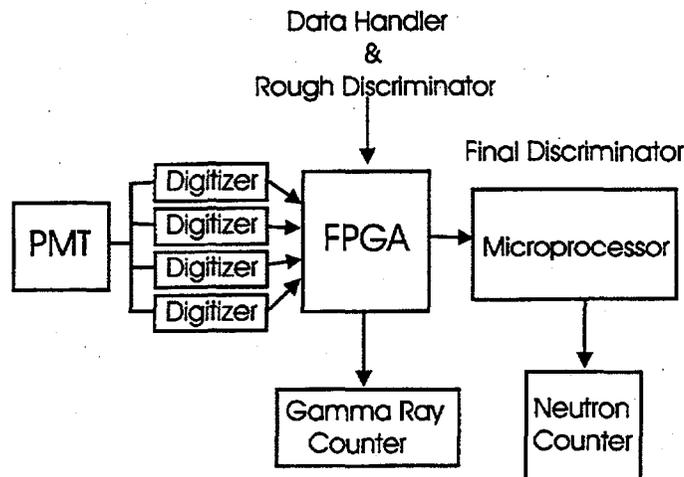
**Figure 5.1.** Schematic Representation of the Proposed Electronic Implementation of a DFND System
