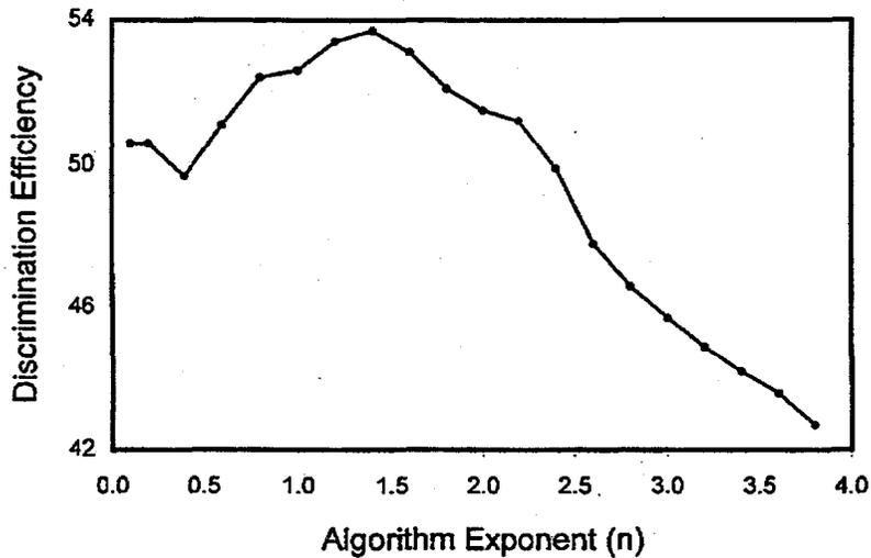
**Figure 3.4.** Graph Showing the Algorithmic Efficiency of the “Pulse Width” Method as a Function of the Exponent Used for Calculation of the Pulse Width. The optimum exponent was found to be 1.4.
