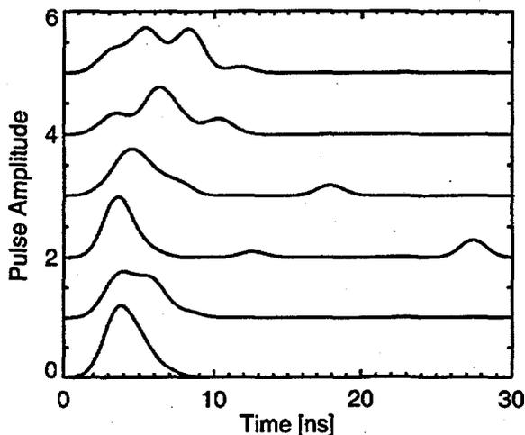
**Figure 1.1.** Six Numerically Calculated Neutron-Interaction Pulse Shapes. These six pulse shapes are typical and are calculated under the assumptions that fast but commercially available scintillators, PMTs, and data acquisition electronics are used.
