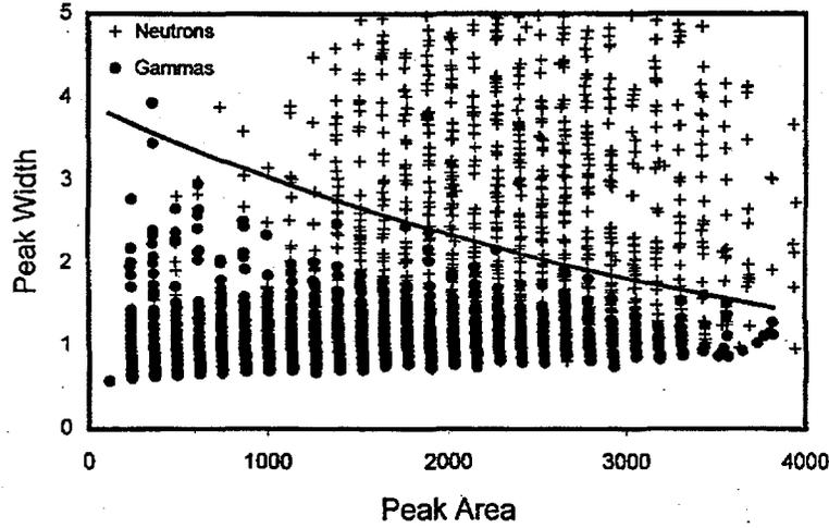
**Figure 3.3.** Plot of the Pulse Width vs. Pulse Area for Numerically Generated Sets of 2000 Neutron and 2000 Gamma Ray Pulses. The line represents the bounding curve that most effectively separates the neutron and gamma ray pulses. The exponent used for the width calculation was 1.4.
