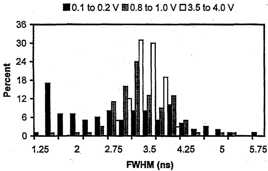
Figure 4.6. Plot Showing Width Spectra for Sets of Pulses with Different Pulse Heights
