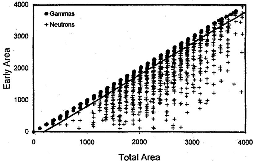
**Figure 3.1.** Plot of Early Area vs. Total Peak Area for Numerically Generated Sets of 2000 Neutron Pulses and 2000 Gamma Ray Pulses. The line represents the bounding curve that most effectively separates the neutron and gamma ray pulses. The cutoff time for this example is 8.0 ns.
