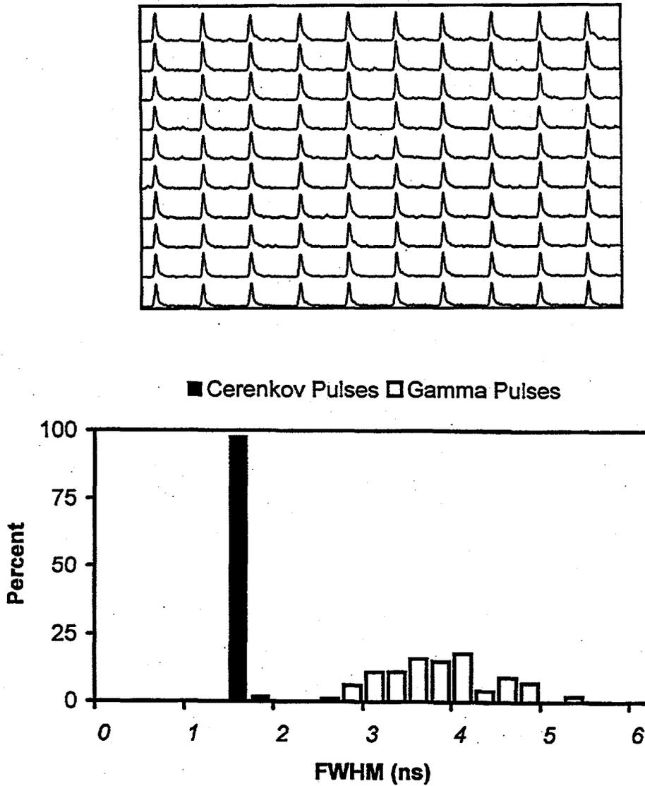
Figure 4.5. Plot Showing 100 Experimentally Acquired Cherenkov Pulses and the Associated Width Spectrum. The average width for this set is roughly 1.4 ns. The width spectrum for a typical set of gamma ray pulses is also shown.
