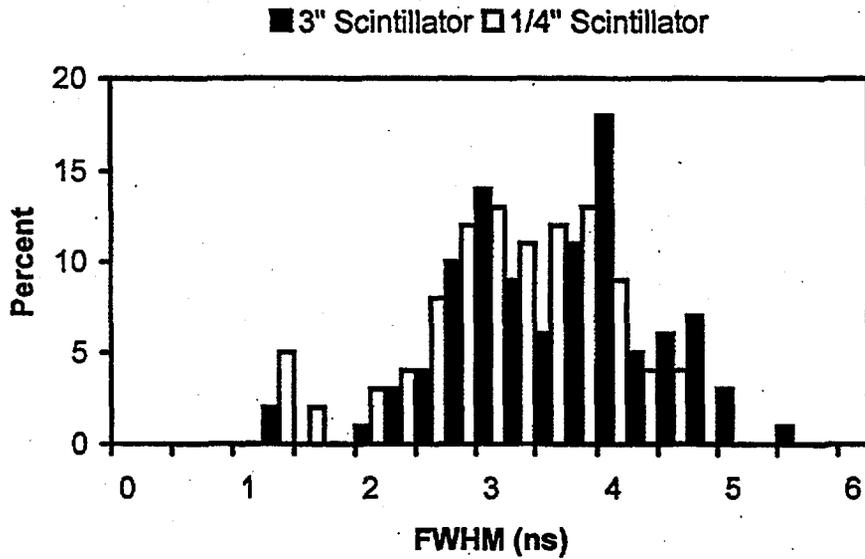
Figure 4.7. Plot Showing Width Spectra for Sets of Pulses Acquired Using Scintillators with Different Sizes
