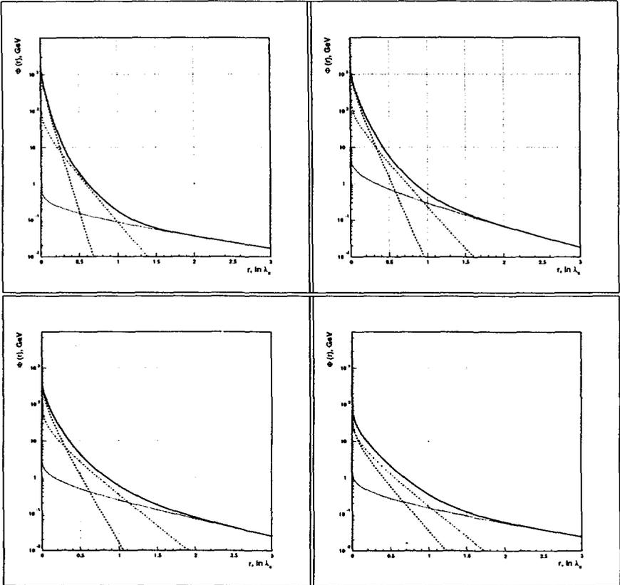
Figure 8: The radial energy density,  $\Phi(r)$ , as a function of  $r$  for TILECAL for various depths: solid lines — the energy densities  $\Phi(r)$ , dashed lines — the contribution from the first term, dash-dotted lines — the contribution from the second term, dotted lines — the contribution from the third term. Depth 1 — up left, depth 2 — up right, depth 3 — down left, depth 4 — down right.
