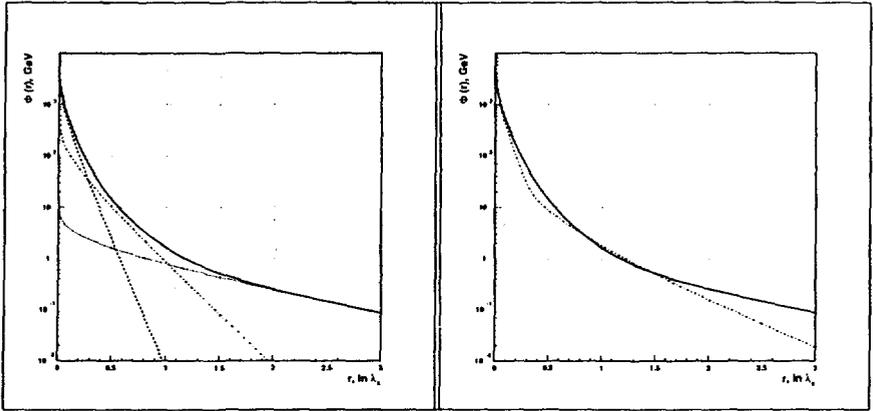
Figure 9: Left: The radial energy density as a function of  $r$  (in units of  $\lambda_f$ ) for TILECAL (solid line), the contribution to  $\Phi(r)$  from the first term (dashed line), the contribution to  $\Phi(r)$  from the second term (dash-dotted line), the contribution to  $\Phi(r)$  from the third term (dotted line). Right: The comparison of the radial energy densities as a function of  $r$  (in units of  $\lambda_f$ ) for TILECAL (solid line) and SPACAL (dash-dotted line).
