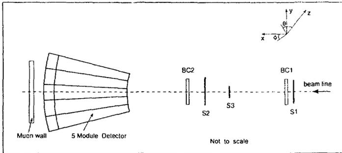
Figure 2: Setup of the tile hadronic calorimeter prototype.
