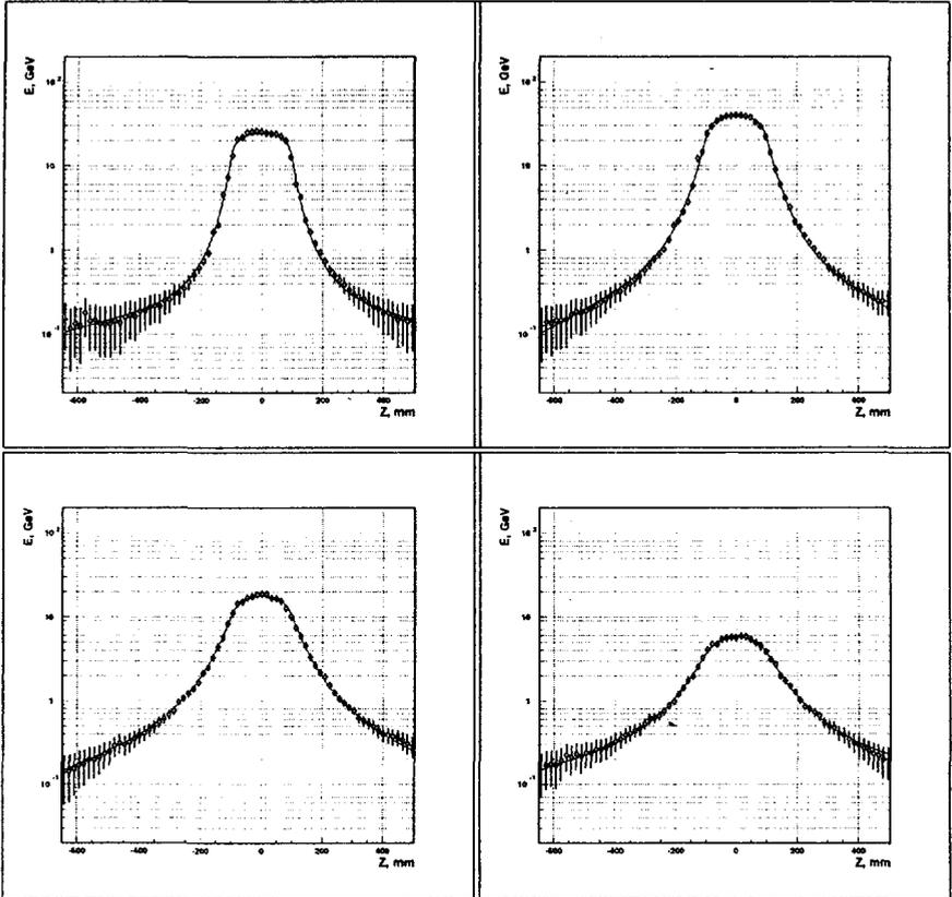
Figure 3: The energy depositions in towers of  $1 \div 4$  depths as a function of  $Z$  coordinate. Depth 1 — up left, depth 2 — up right, depth 3 — down left, depth 4 — down right. Curves are fits of equation (14) and (15) to the data.
