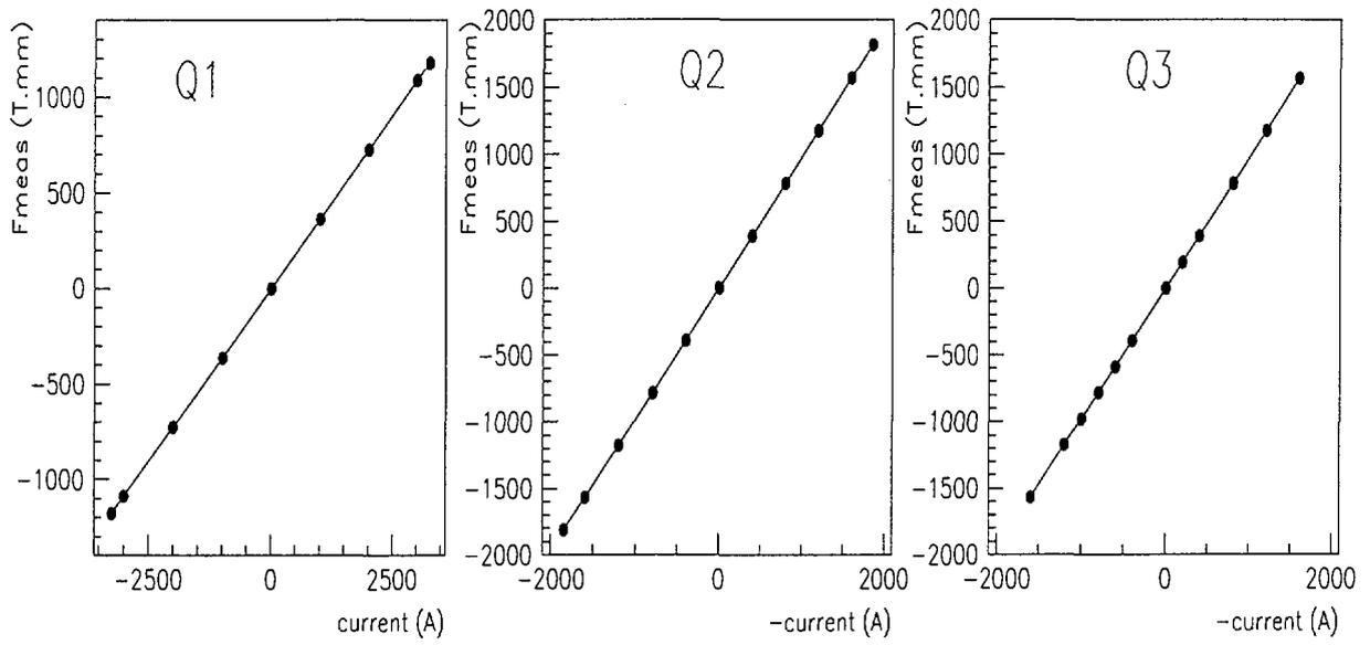
Figure 3: Hysteresis loop in terms of field integrals  $F$  for the HRS quads.
