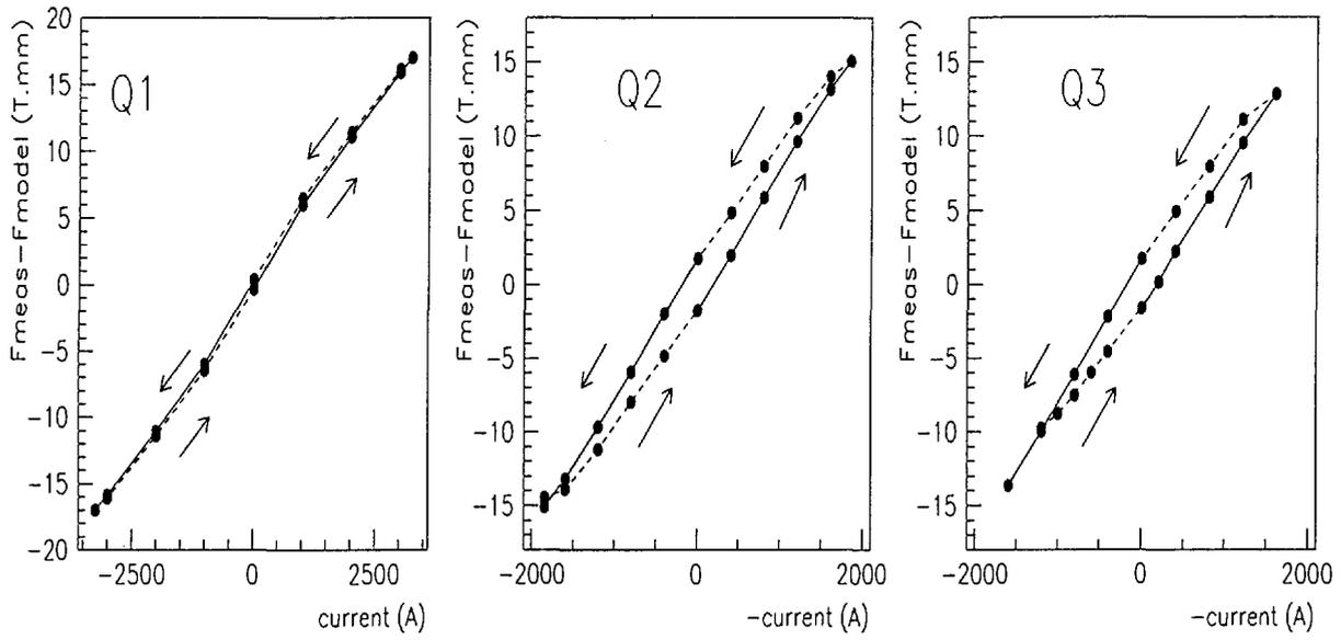
Figure 4: Hysteresis loop in terms of differential variable  $y = F_{meas} - F_{model}$  for the HRS quads. The loop has been measured starting at  $I = -3250/+1850/+1200$  A for Q1/Q2/Q3 and following the arrows.
