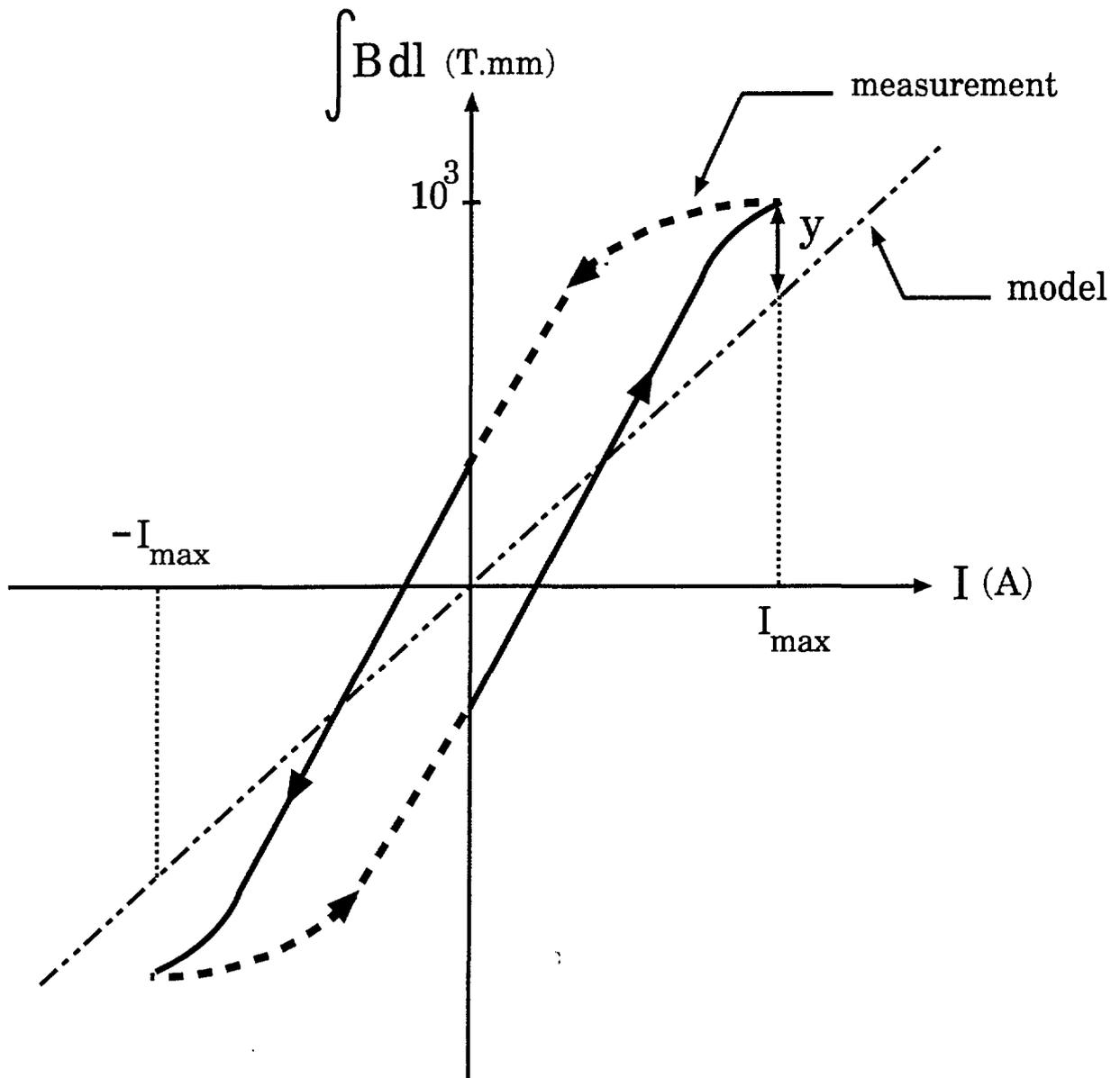
Figure 1: Hysteresis loop (schematic) in terms of field integrals  $F$ .
