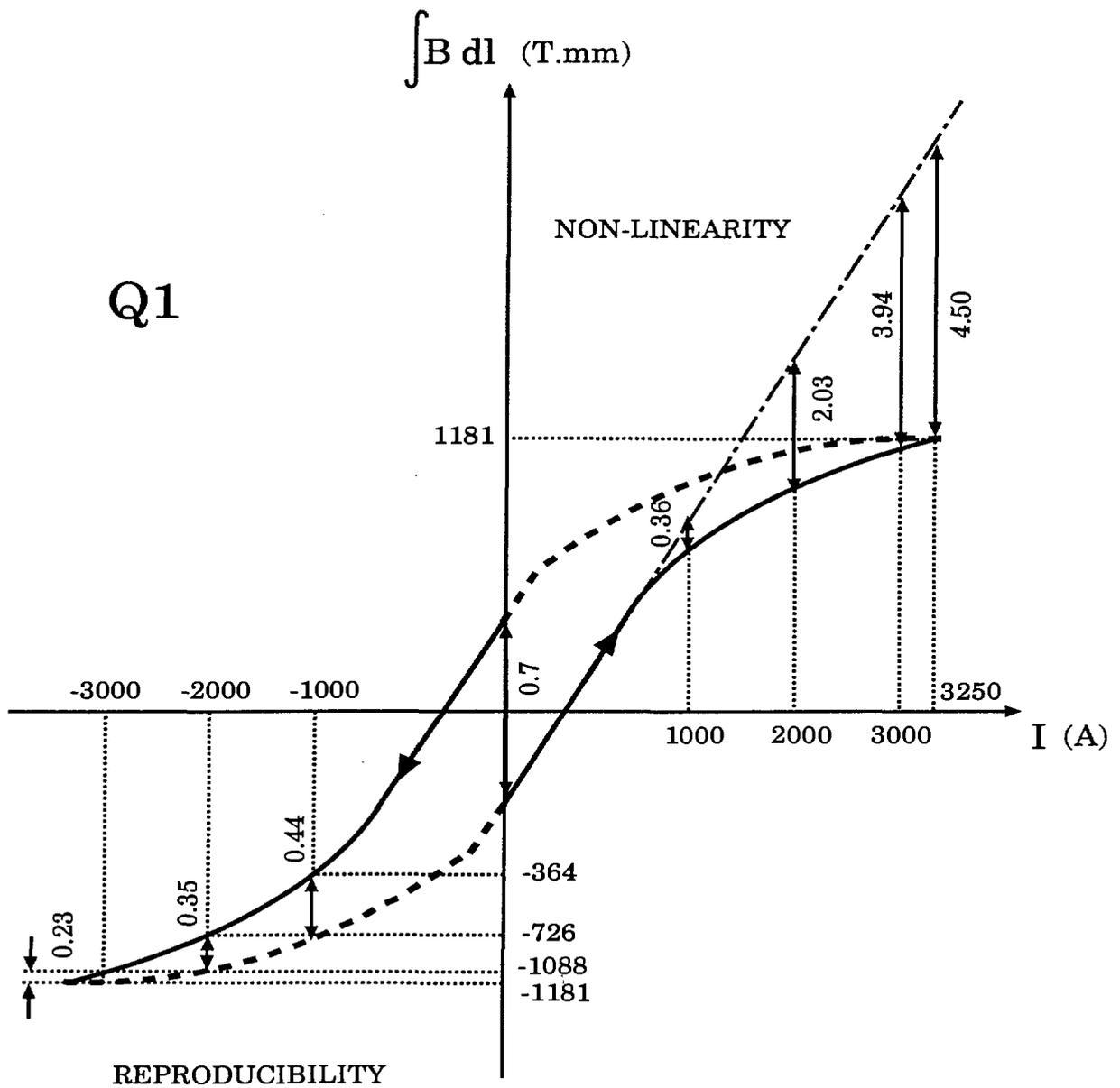
Figure 6: Hysteresis loop (schematic) with results on linearity and reproducibility for Q1. Numbers on the plot are in T.mm.
