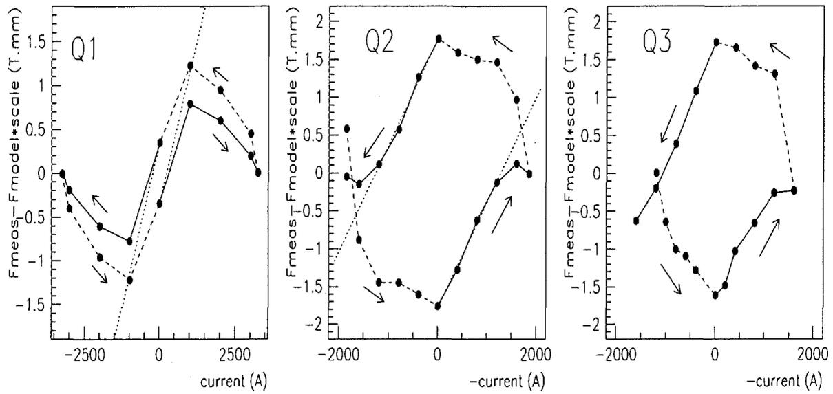
Figure 5: Hysteresis loop in terms of differential variable  $y_1 = F_{meas} - F_{model} \times (1 + \alpha)$  for the HRS quads. The variable  $y_1$  is chosen such that  $y_1(\pm I_{max}) \simeq 0$ . The loop has been measured starting at  $I = -3250/+1850/+1200$  A for Q1/Q2/Q3 and following the arrows.
