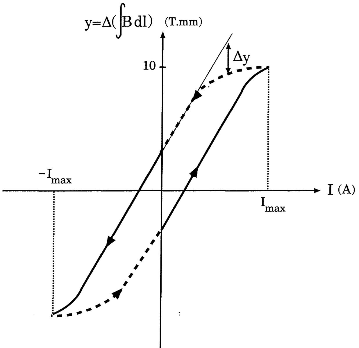
Figure 2: Hysteresis loop (schematic) in terms of differential variable  $y = F_{meas} - F_{model}$ .
