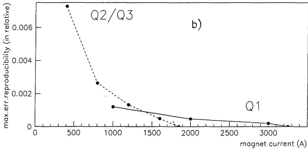
Figure 8: Summary of results on field linearity and setting reproducibility for Q1 and Q2/Q3.
