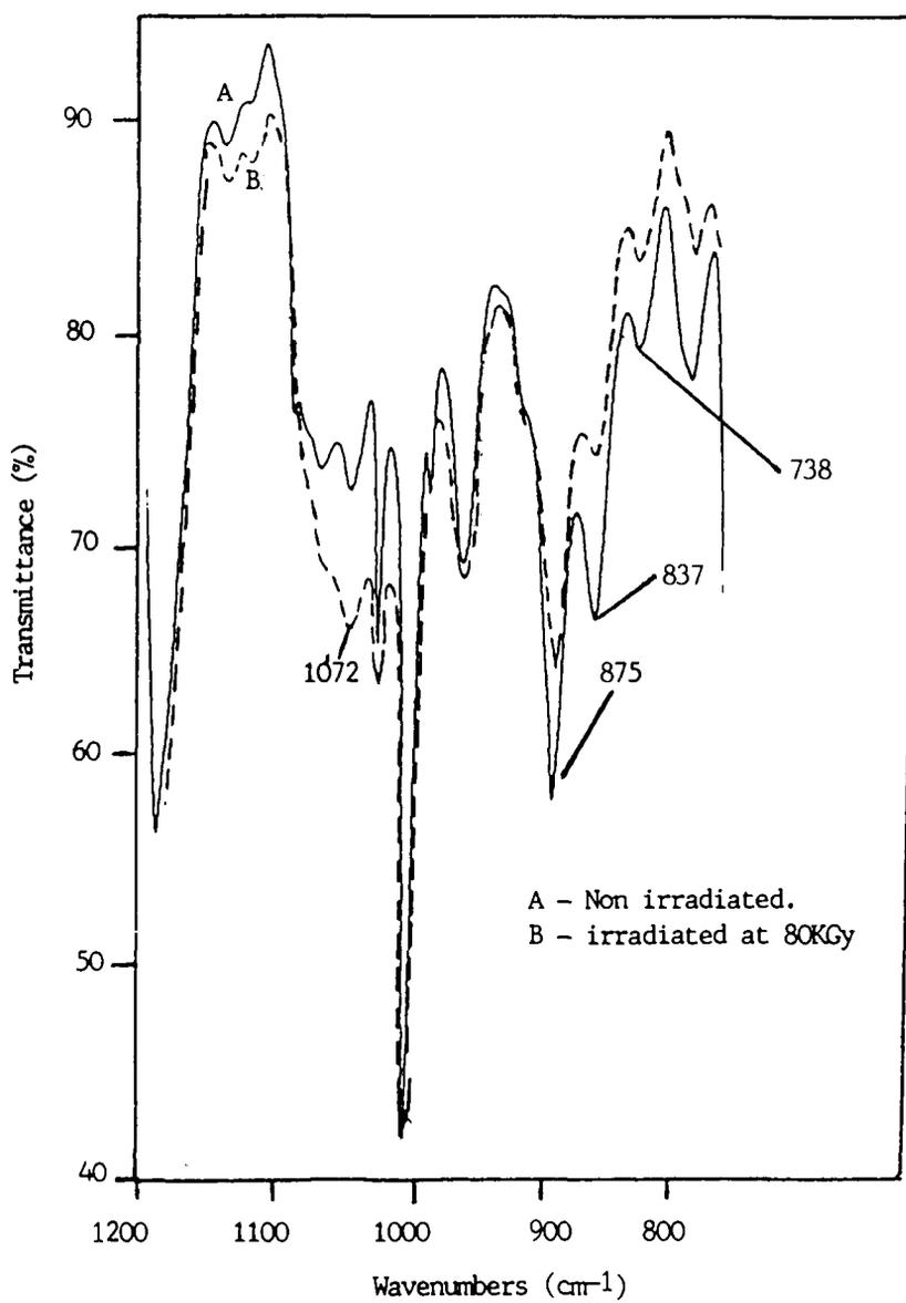
Figure 5. IR Spectra of 50% PVC blend
