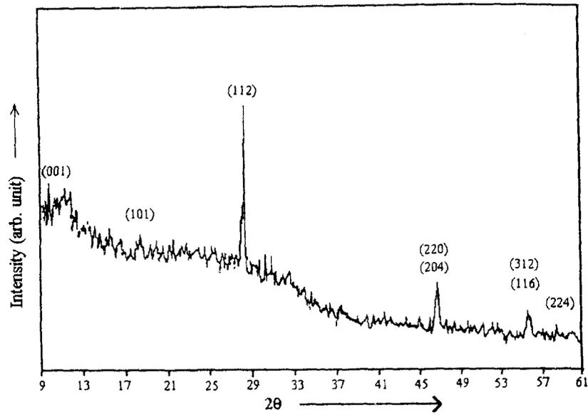
**FIGURE 2:** X-Ray Diffraction Spectra of CuInS<sub>2</sub> Thin Film (449.5 nm)
