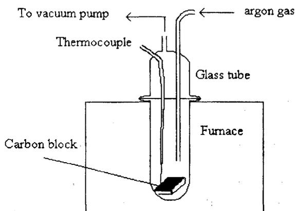
**FIGURE 1:** Annealing Sample in Carbon Block
