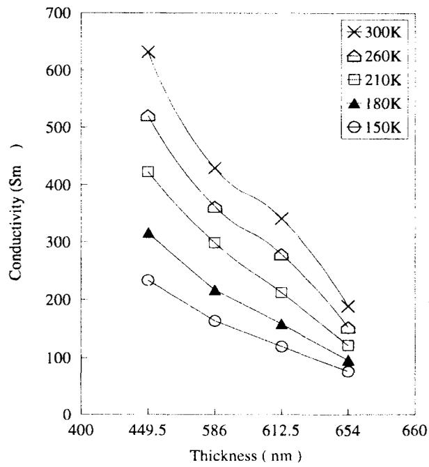
**FIGURE 6:** The Variation of Conductivity against Thickness for  $\text{CuInS}_2$  Thin Films
