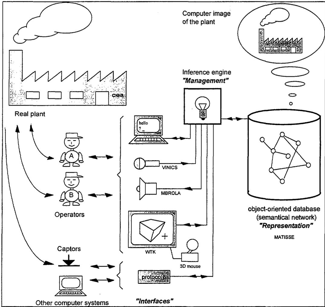
Figure 1. Overview of ImagIn system's components .
