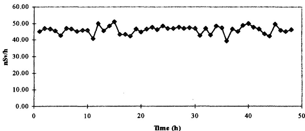
Fig 3: Gamma dose rate from telemetric station in N. Philadelphia (Athens area).
