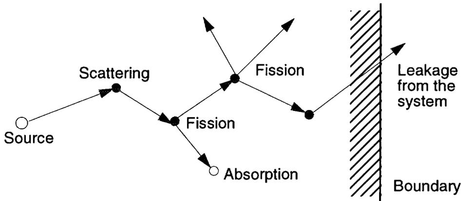
Fig. 2. A schematic view of neutron transport
