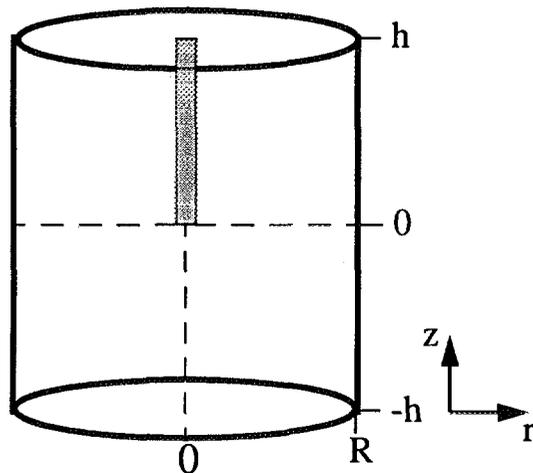
*Fig. 1. The cylindrical reactor model with an absorber rod present from the top to the mid-plane of the reactor.*
