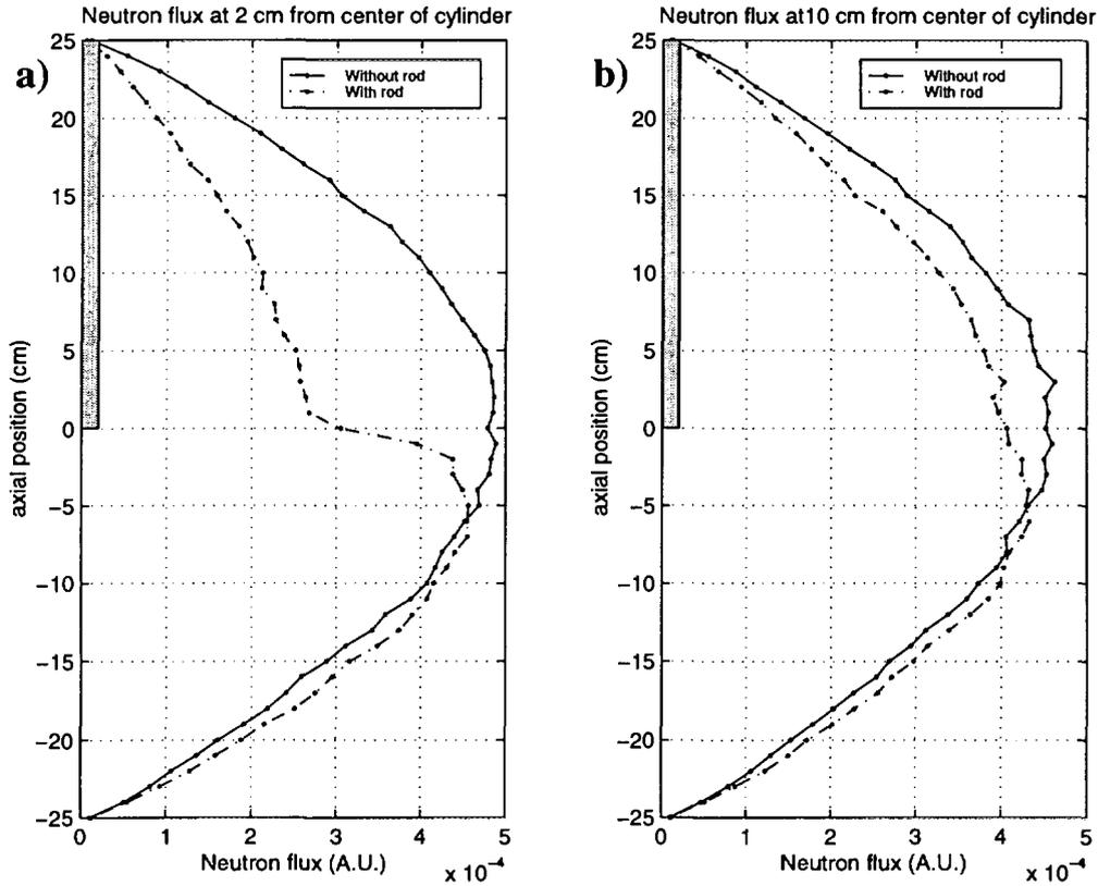
Fig. 5. The figure shows the flux as a function of axial elevation for the case with the rod present (dash-dotted line) and without the rod present (solid line) and also for two distances from the centre of the reactor, i.e. a) 2 cm and b) 10 cm.
