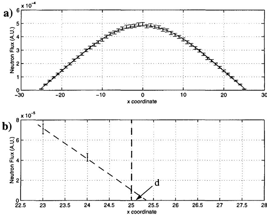
*Fig. 3. Figure a) shows the neutron flux with error bars along the diameter (called the x-coordinate [cm]) at the axial centre of the reactor. Figure b) shows three values of the flux close to the boundary connected with a line, which indicates the extrapolation distance.*
