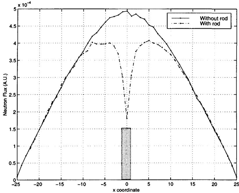
Fig. 4. The neutron flux along the diameter of the reactor for the two cases with the rod present (dash-dotted line) and without the rod present (solid line).
