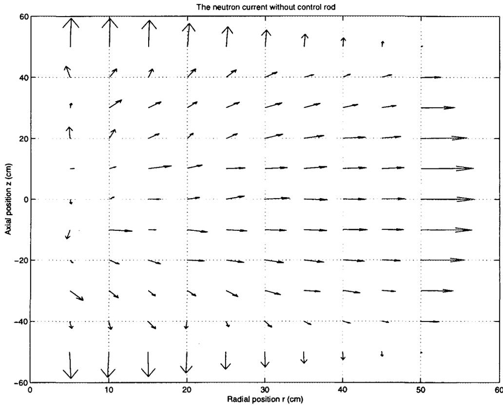
Fig. 8. The neutron current as a function of position in  $r, z$  geometry. The arrows show both the relative magnitude and the direction of the current vector as a function of position.
