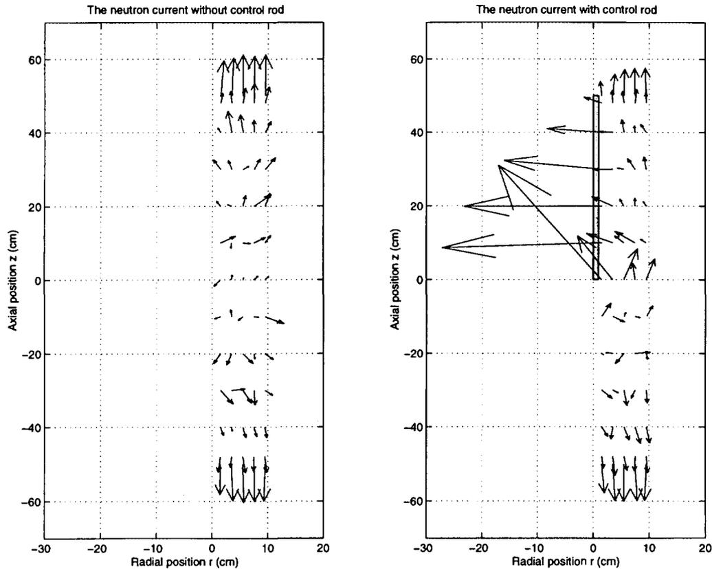
Fig. 9. The neutron current vector as a function of position for a) the unperturbed reactor and b) the reactor with the rod present.
