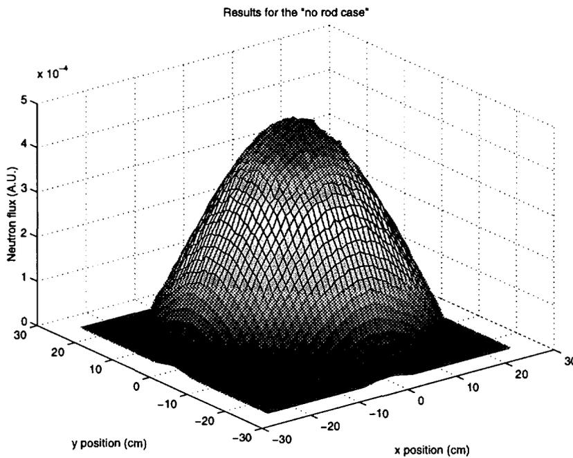
Fig. 6. The 2-D neutron flux for the unperturbed system.
