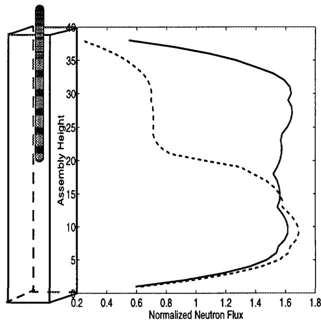
*Fig. 7. The axial neutron flux inside a fuel element. The solid curve is the neutron flux without the rod present. The dashed curve shows the distortion of the neutron flux caused by the presence of the rod.*
