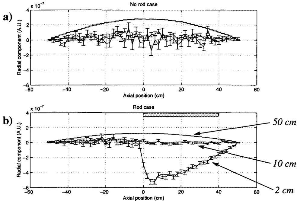
*Fig. 10. The neutron current with error bars as a function of axial position, for three different radial positions from the centre of the reactor and for a) the unperturbed reactor and b) the reactor with the rod present.*
