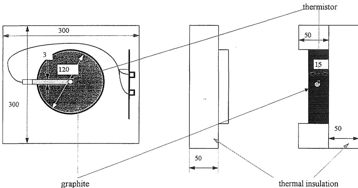
Fig.3. The graphite calorimeter
