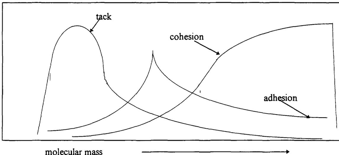
Fig.2. Relationship between the properties of self adhesive glue and the polymer molecular mass for wide range of change of molecular masses
