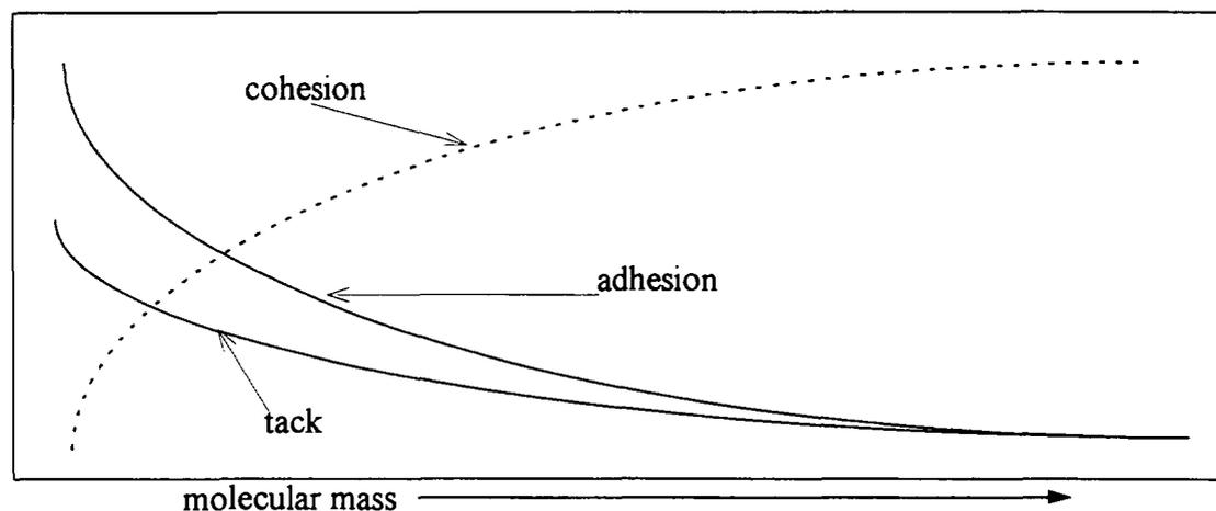
*Fig.1. The main properties of pressure sensitive adhesive vs. molecular mass of used polymer, after [ 2]*
