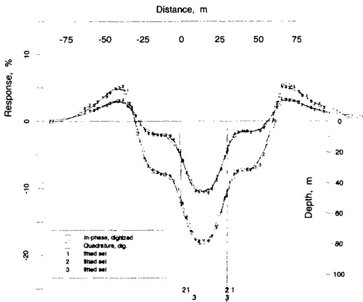
**Figure 2.** Digitized small scale experiments of Ketola and the results of interpretation.
