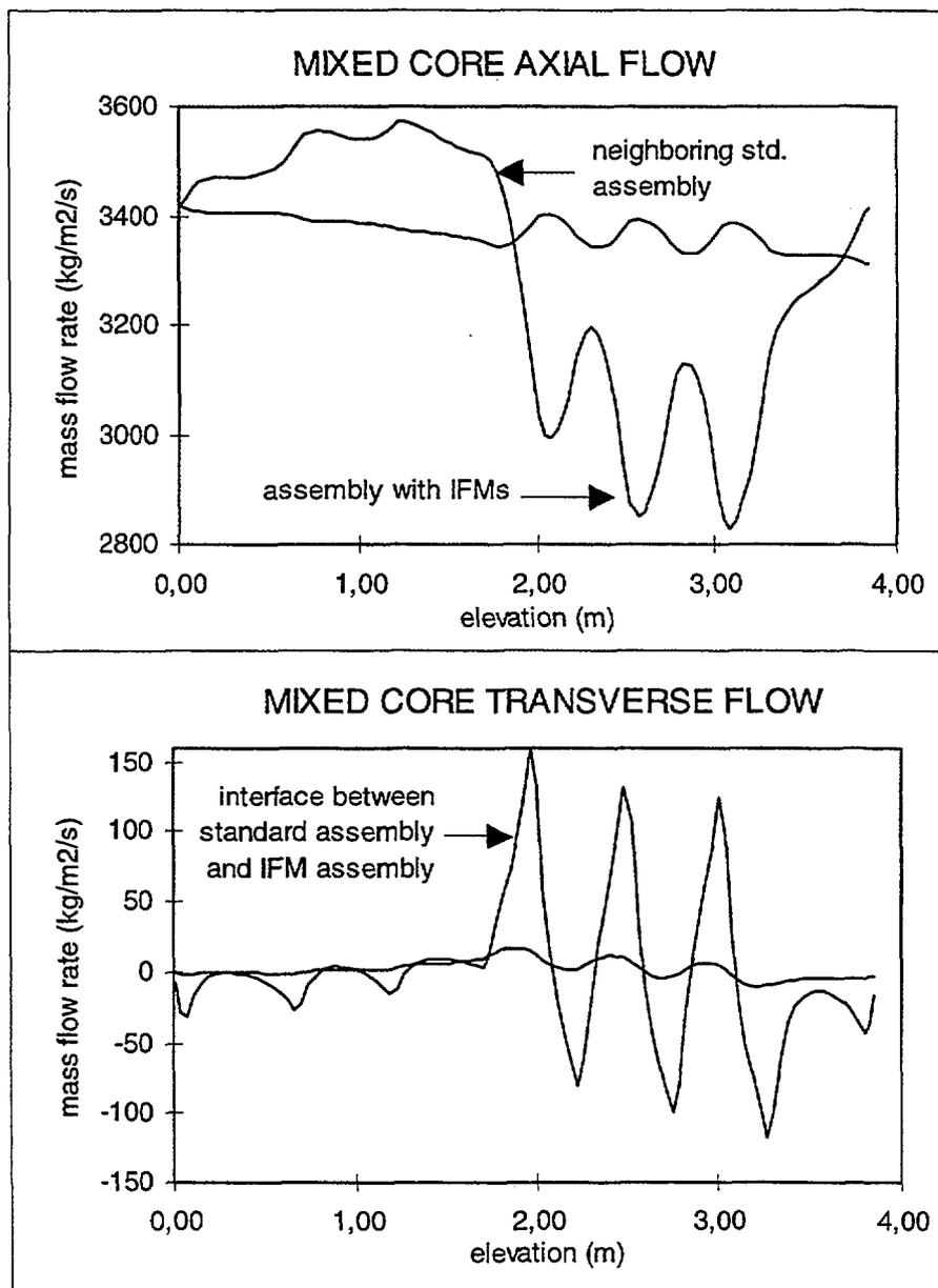
Figure 4: Axial and transverse mass flow rate profiles for a mixed core with one assembly with IFMs.
