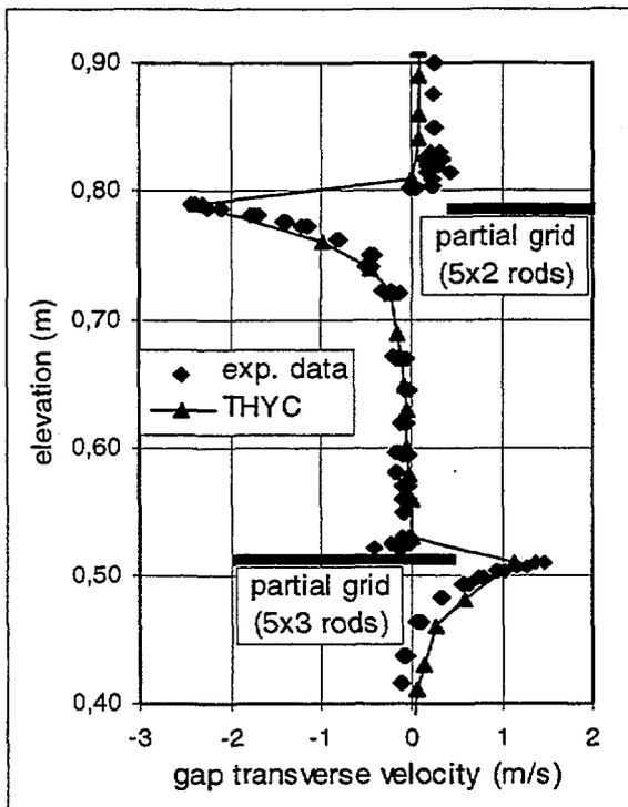
Figure 1: Measured vs. predicted transverse velocity, AGATE test section with partial grids.
