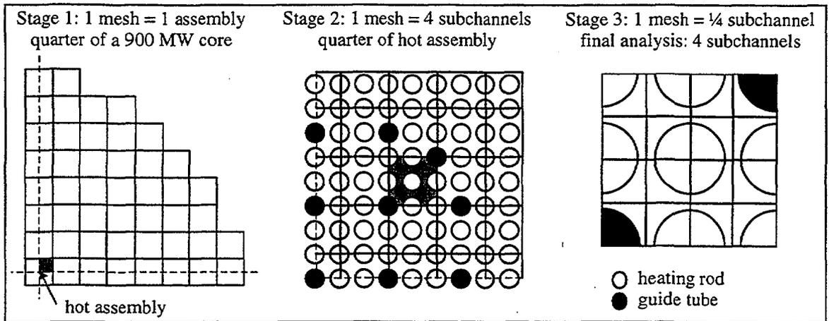
Figure 3: THYC three-stage core analysis.
