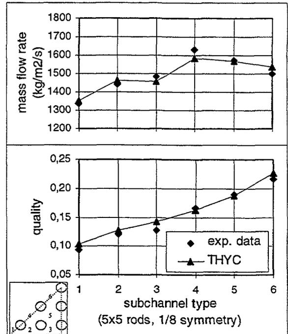
Figure 2: Measured vs. predicted subchannel mean values of mass flow rate and quality, GRAZIELLA-P test section.
