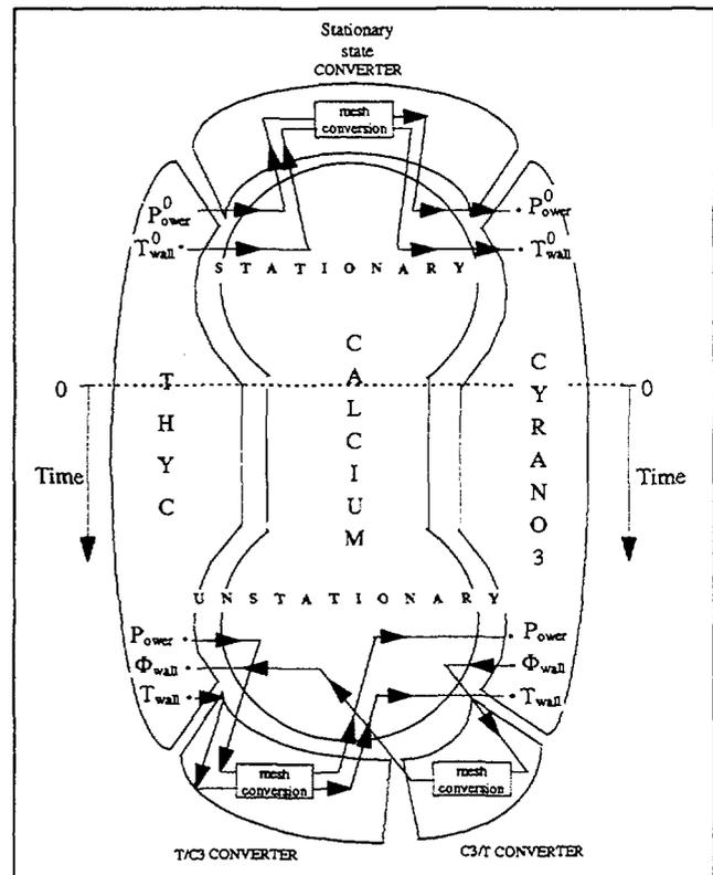
Figure 2: Logic diagram exchanged variables in the coupling THYC/CYRANO3
