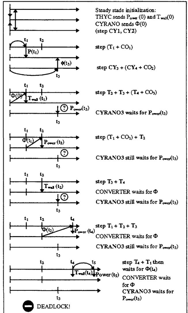
Figure 7: Deadlock using only one converter
