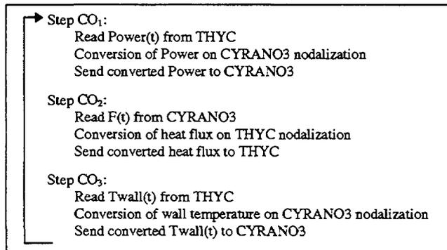
Figure 4: Logic diagram of one converter
