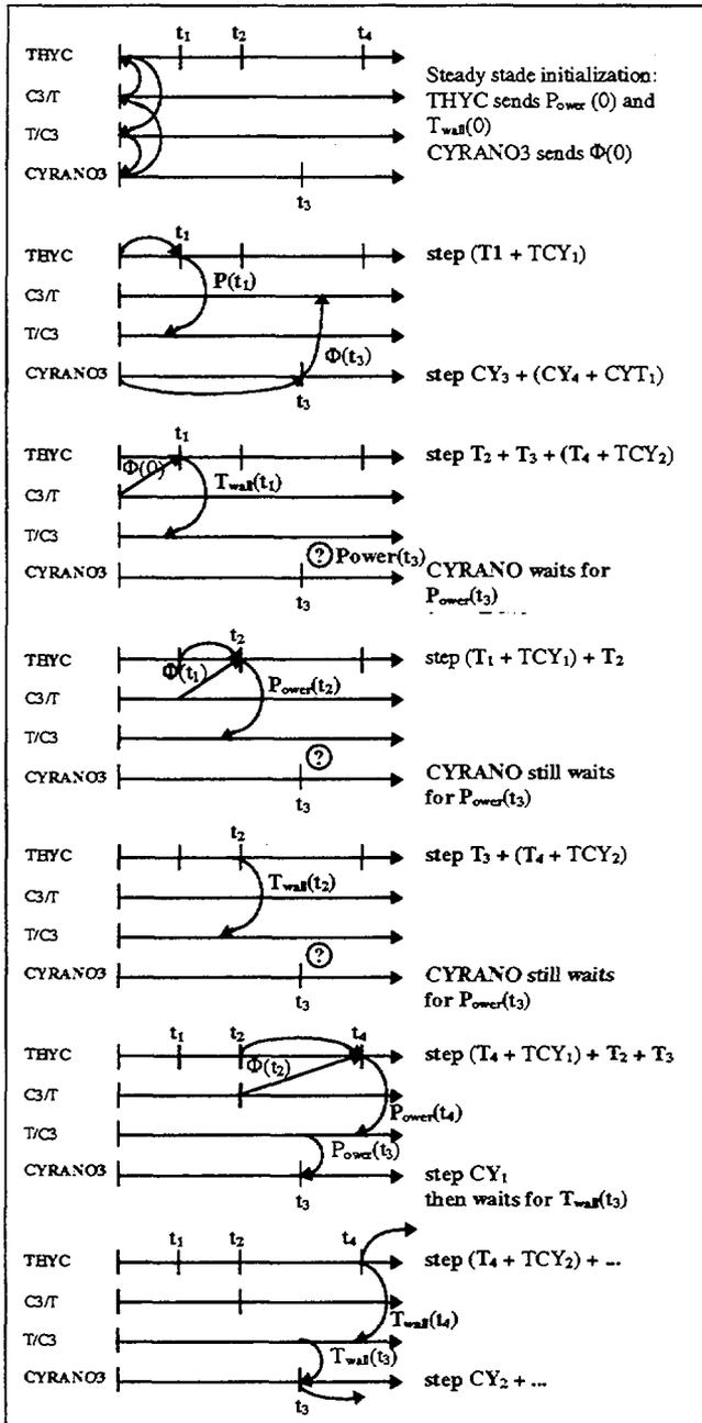
Figure 8: Timing of the T/C3 coupling with two unstationary converters
