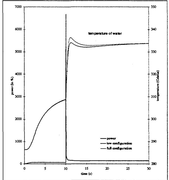
Figure 14: Rod ejection power transient
