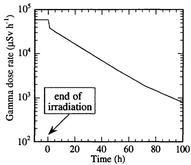
Figure 4: Gamma dose rate after 15 days of irradiation at 47 cm from the target for  $^{36}\text{S}$  (77MeV/A,  $1 \cdot 10^{13}$ pps)->  $^{12}\text{C}$
