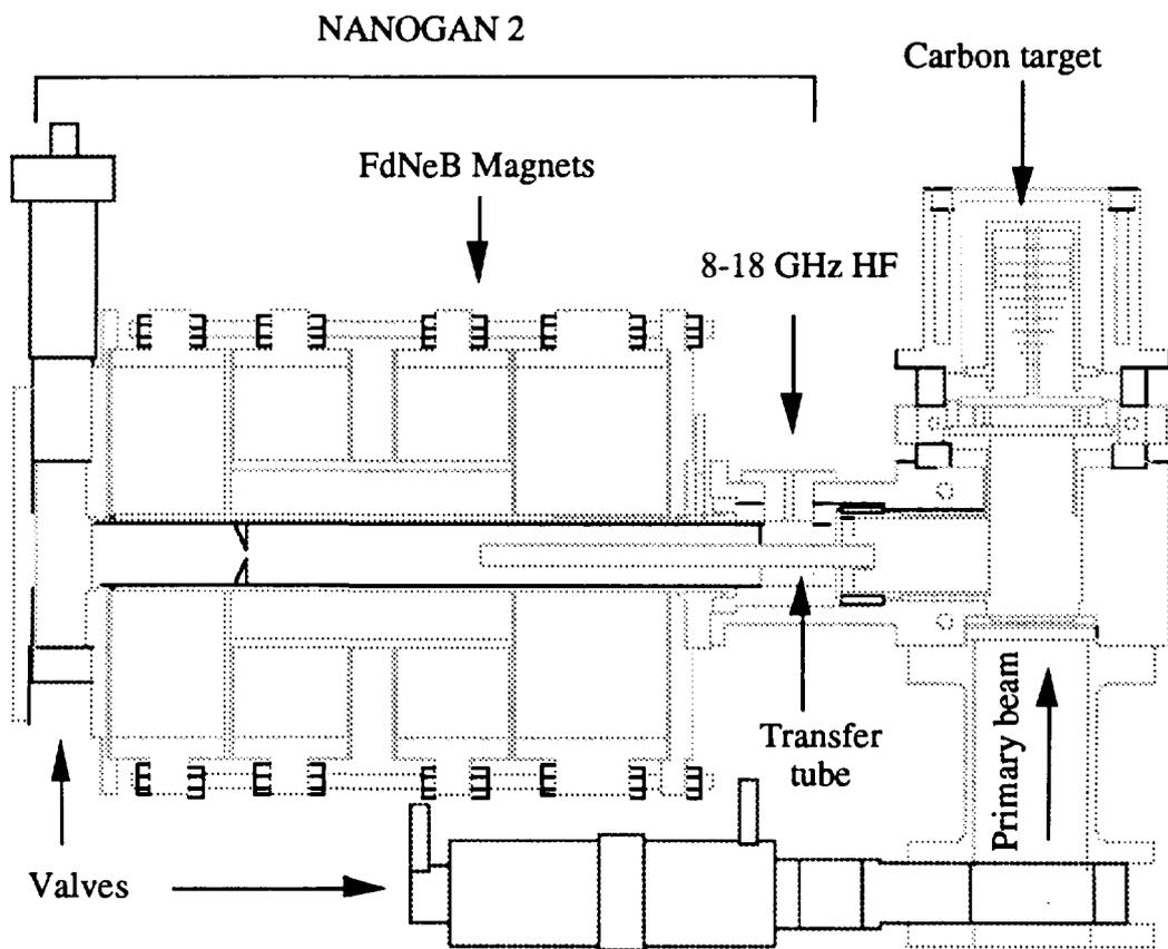
Figure 1: the target ion source system (TISS)
