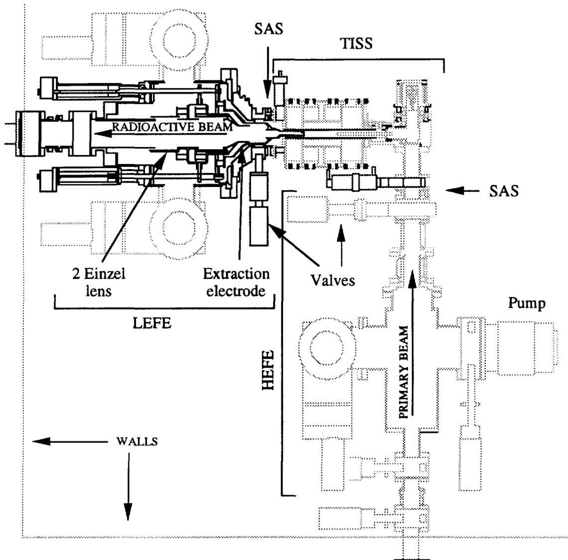
Figure 2: The elements located inside the production cave.
