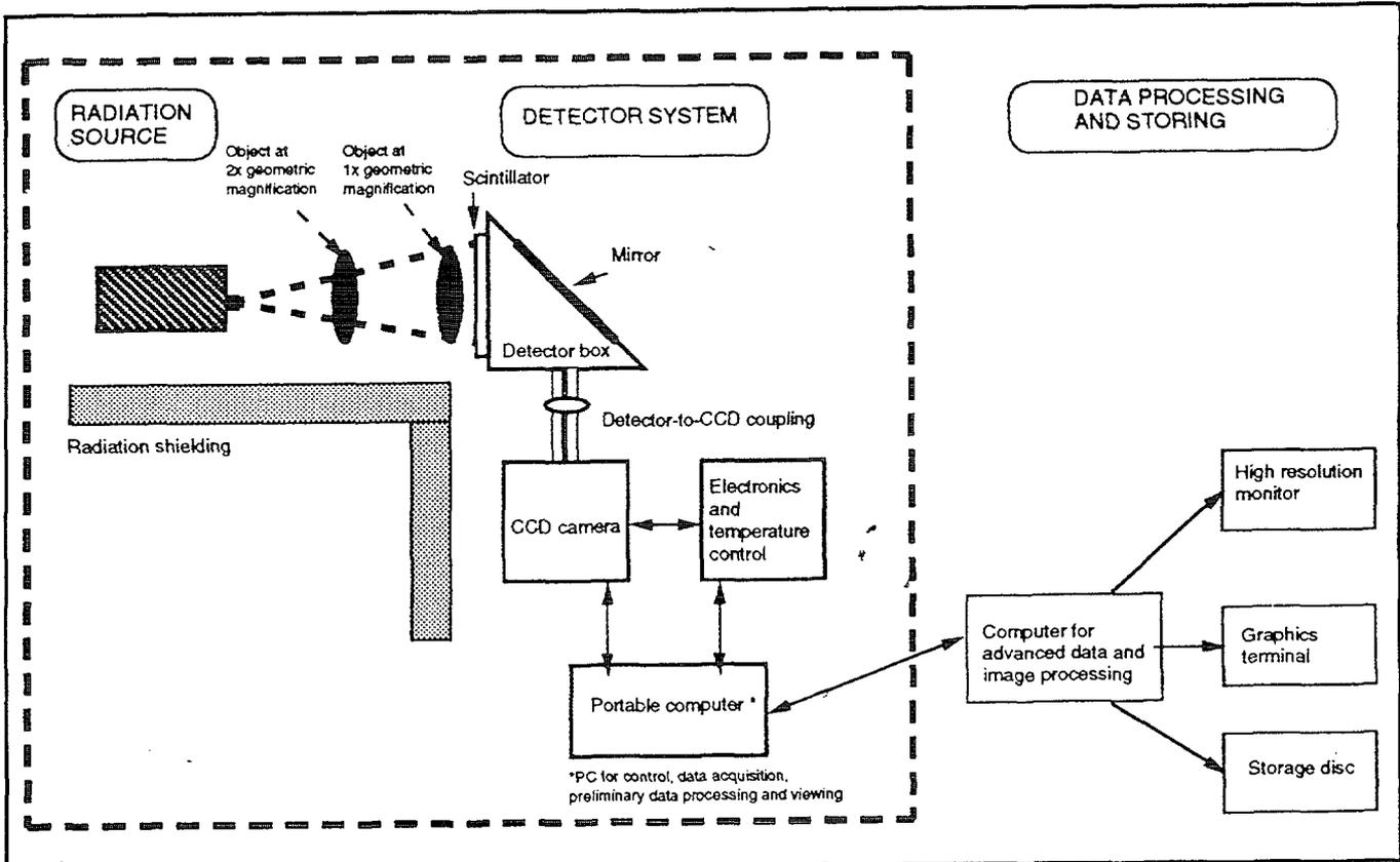
Figure 1: Block diagram of the SSI system
