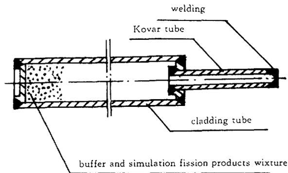
FIG.1 Profile of the prepared cladding tube specimen
