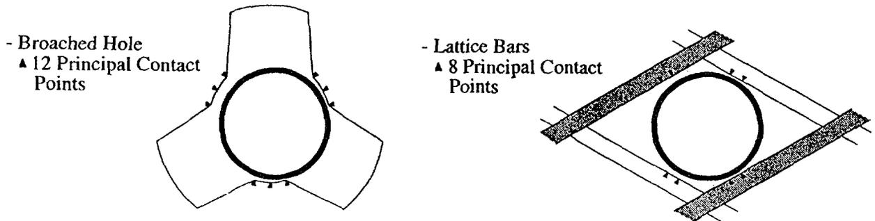
Figure 4: Complex Tube-Support Geometry: Possible Contact Points
