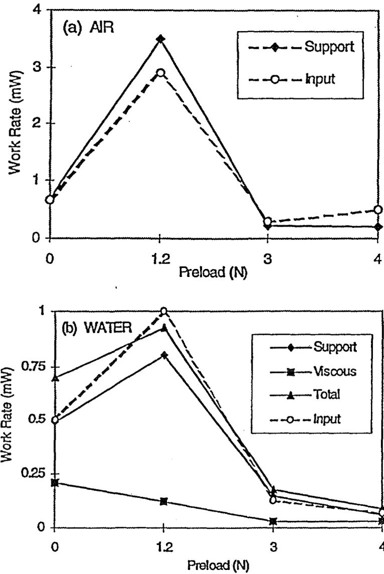
Figure 9: Input and Dissipated Work-Rates for Multispan Heat Exchanger Tube Tests
