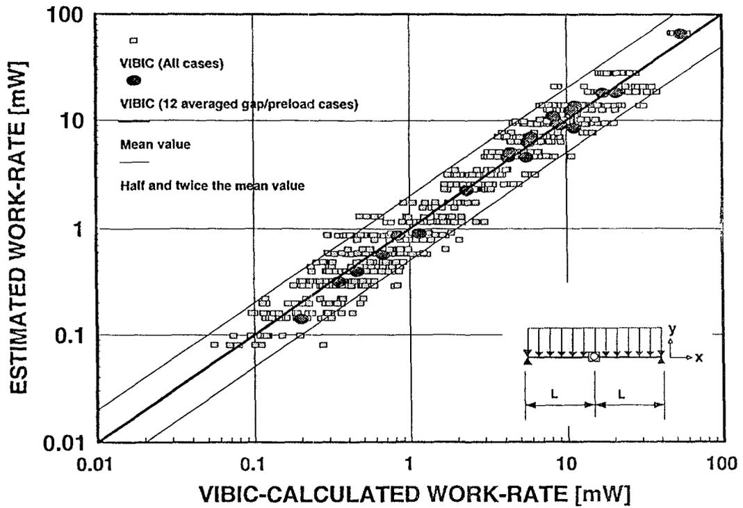
Figure 10a: Estimated and VIBIC-Calculated Work-Rates for all Two-Span Simulations. (Total number of simulations is 1144. Only 27 (3%) data points are outside the factor-of-two bounds.)
