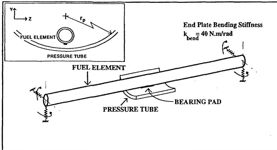
Figure 6: Model of Fuel Element Bearing Pad and Fuel Channel Contact
