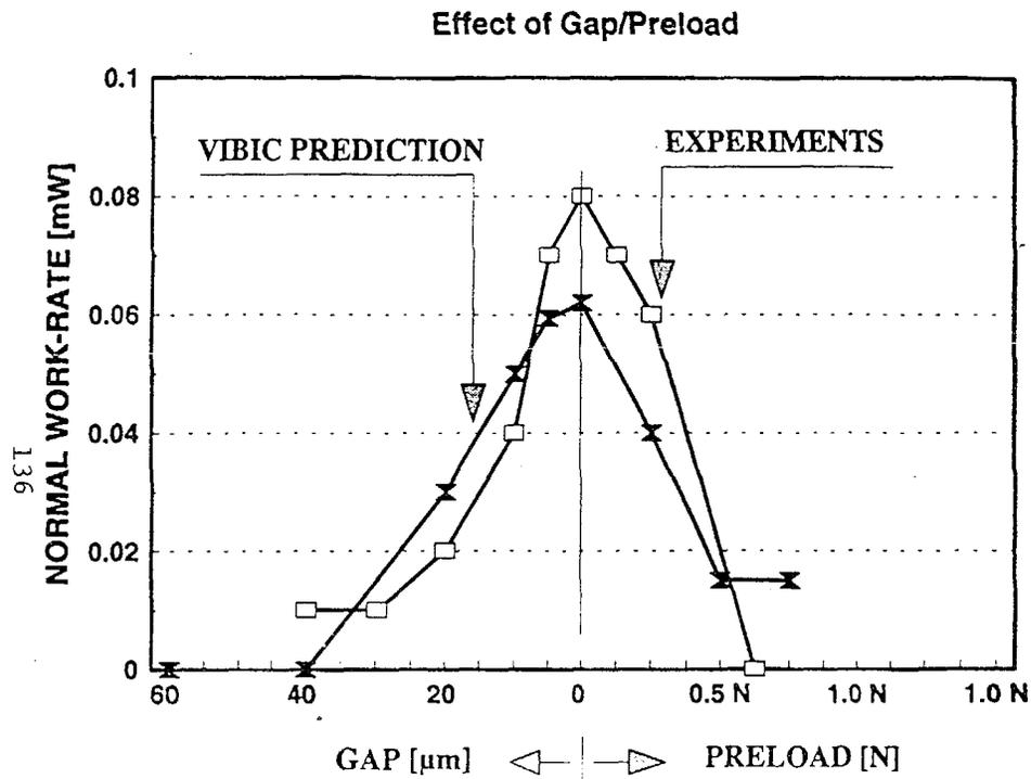
Figure 7: Work-Rate Versus Gap/Preload for a Fuel Element Vibration Response of 25 μm RMS
