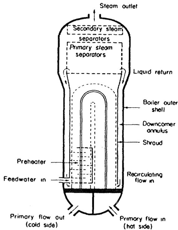
Figure 1: Typical Nuclear Steam Generator
