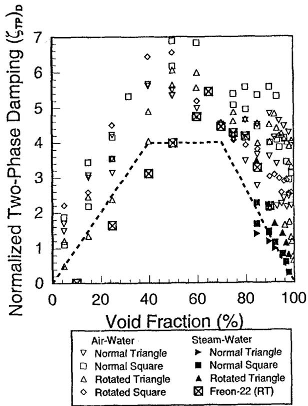
Figure 3: Available Damping Data in the form of Normalized Two-Phase Damping Ratios Showing the Effect of Void Fraction
