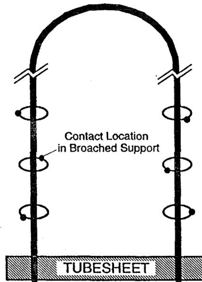
Figure 5: Steam Generator Tube and Support Contact Combinations
