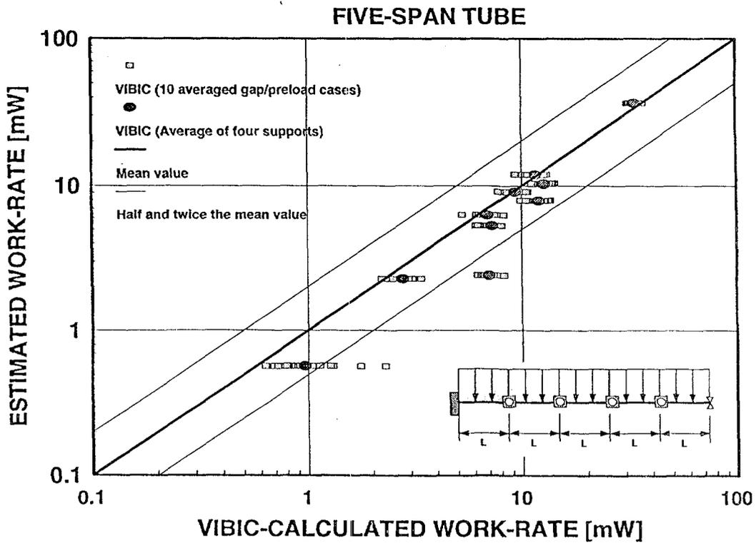
Figure 10b: Estimated and VIBIC-Calculated Work-Rates for all Five-Span Simulations. (Total number of simulations is 275. Twenty nine (10.5%) data points are outside the factor-of-two bounds.)
