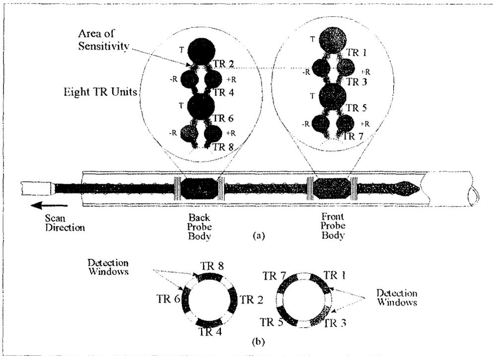
Figure 7. C3 probe showing T/R coil configuration and detection windows.
