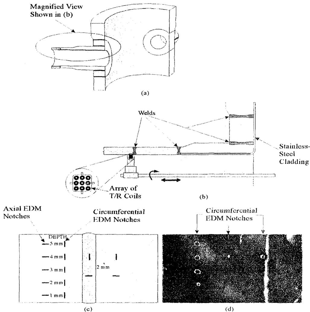
Figure 5. Eddy current detection of surface cracks in stainless-steel clad PWR pressure vessel.
