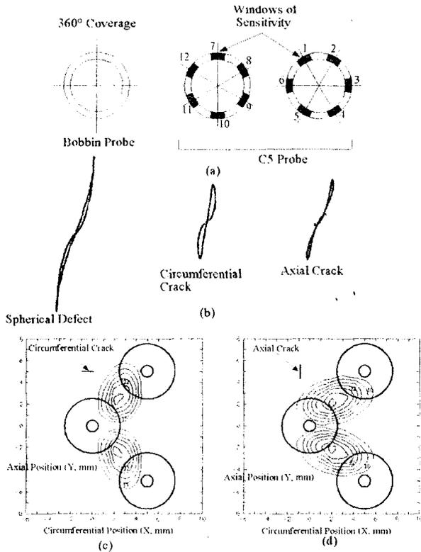
Figure 9. (a) Cross section view of the C5 probe. (b) Computed-predicted response to various defects. (c) Computer-predicted areas of sensitivity for the C5 probe to short circumferential cracks. (d) Computer-predicted areas of sensitivity for the C5 probe to short axial cracks.
