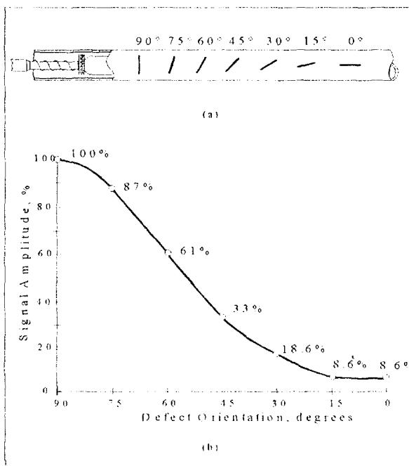
Figure 3. Plot of signal amplitude versus defect orientation for a differential C3 probe at 250 kHz from EDM notches 100% deep by 10 mm long in an Inconel 600 calibration tube.
