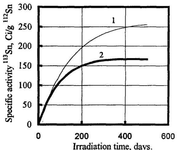
Fig.1 Specific activity <sup>113</sup>Sn vs irradiation time. 1- without consideration of <sup>113</sup>Sn "burn-up", 2- with consideration of <sup>113</sup>Sn "burn-up"
