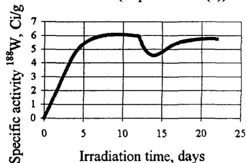
Fig.3 Specific activity  $^{188}\text{W}$  vs irradiation time during real reactor schedule.
