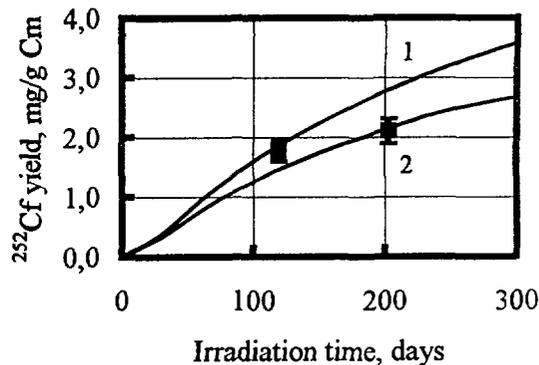
Fig.2 Comparison of  $^{252}\text{Cf}$  yield during the heavy curium irradiation on neutron trap SM reactor. 1-after neutron trap reconstruction, 2- before reconstruction, ■ - experiment
