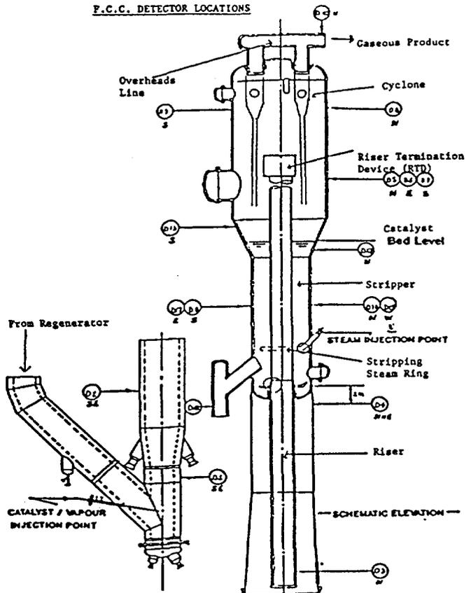
FIGURE 1. Equipment Layout for Radioactive Tracer Studies.
