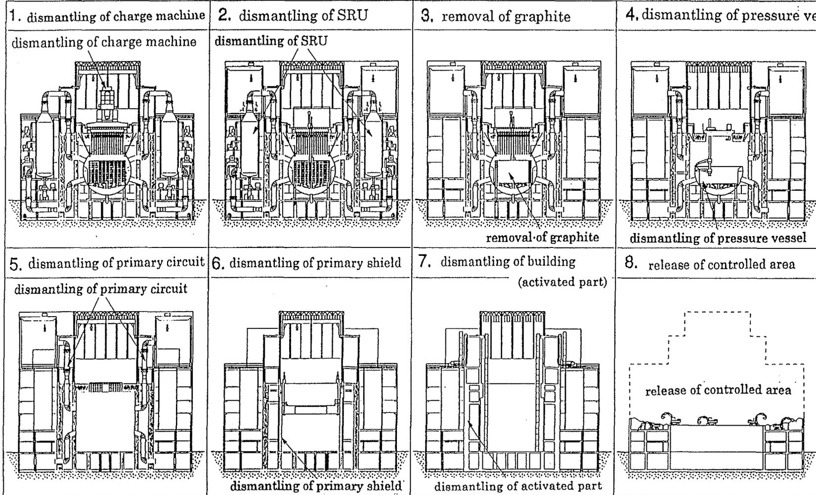
Fig.4 Outline of dismantling process of Tokai Power Plant
