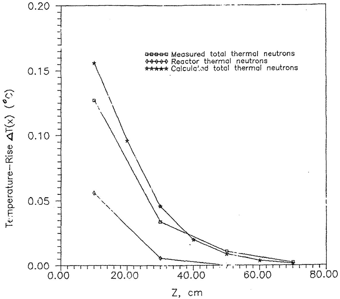
Figure 4 Temperature-rise distribution of gamma-rays due to capture of thermal neutrons in ordinary concrete
