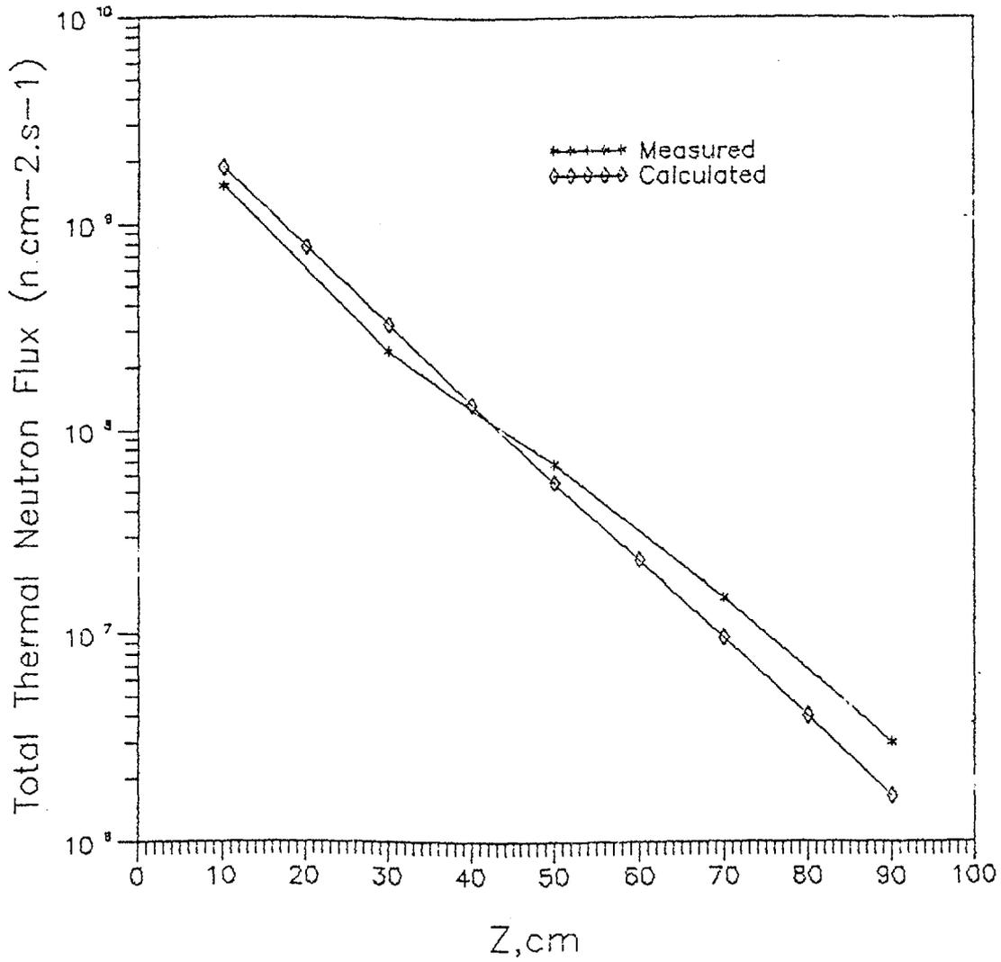
Figure 1 Measured and calculated total thermal neutron fluxes in ordinary concrete.
