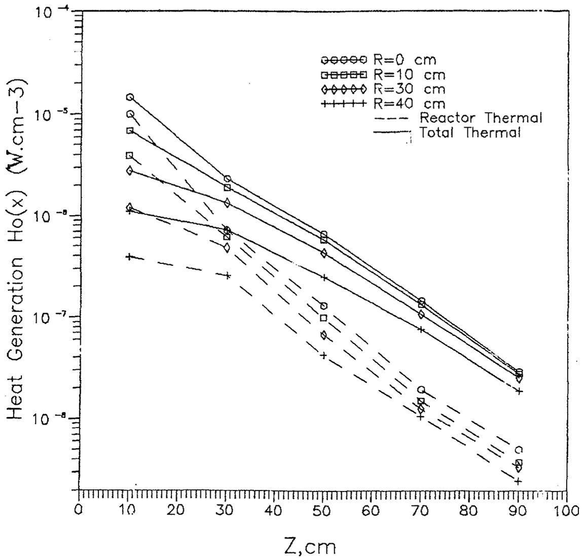
Figure 3 Heat generation in ordinary concrete evaluated using measured total and reactor thermal neutron fluxes
