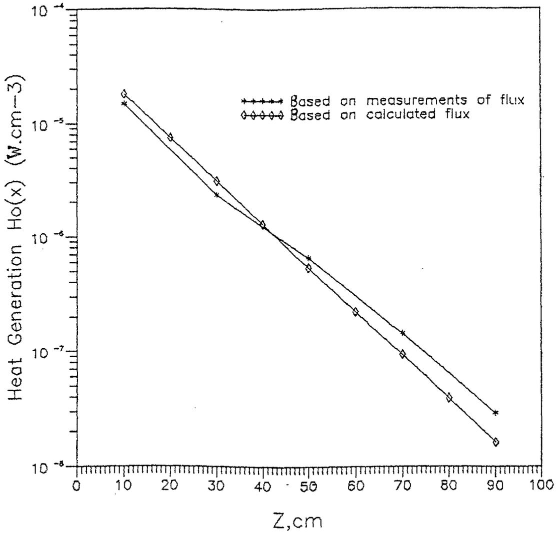
Figure 2 Heat generation in ordinary concrete evaluated using measured and calculated total thermal neutron fluxes
