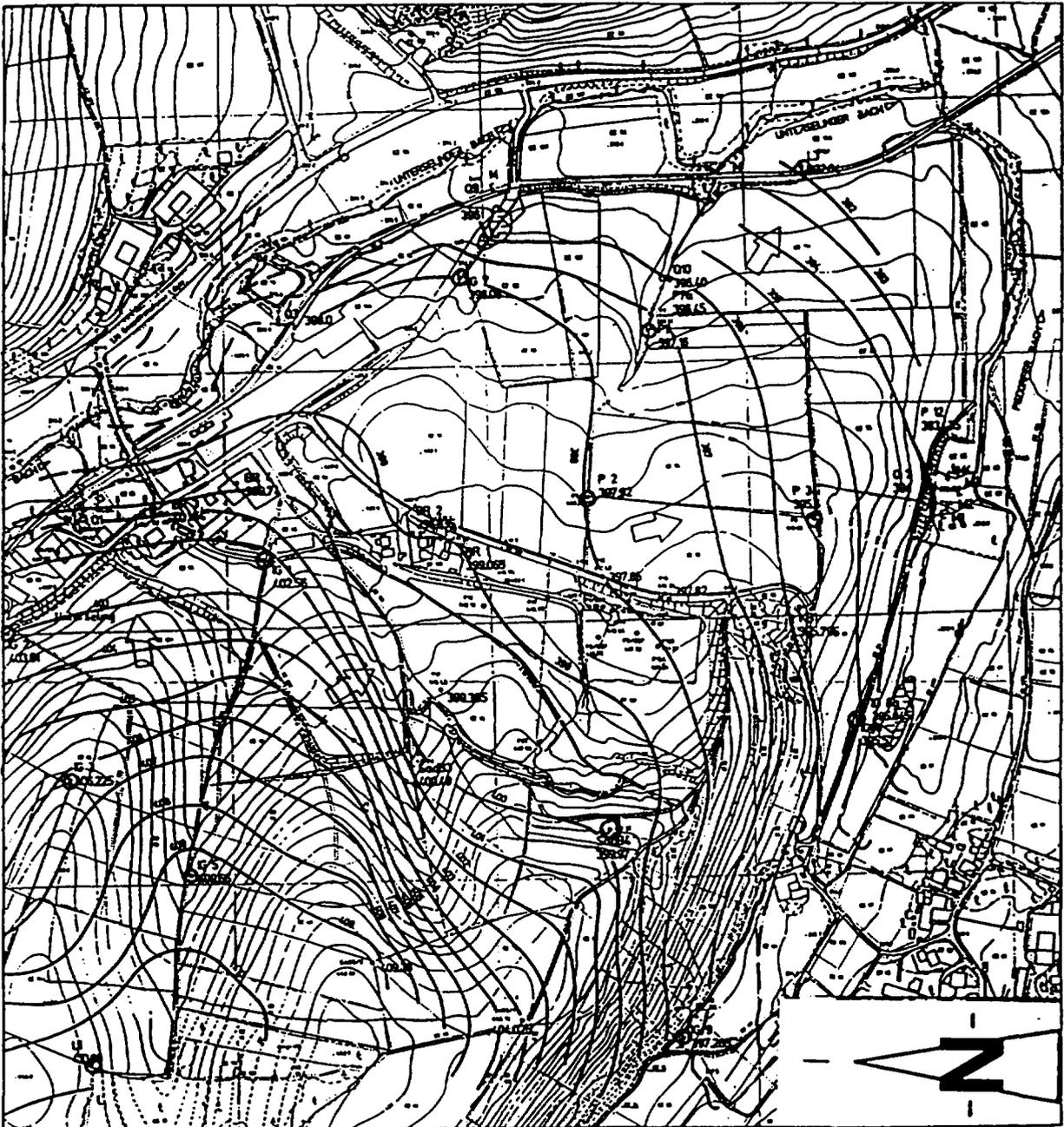
**Figure 1. Location map of boreholes and groundwater contours.**
