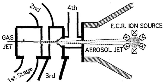
FIGURE 2. Skimming system for injecting aerosols into the ECR ion source.
