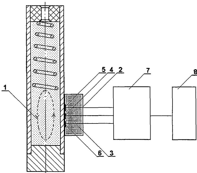
FIG. 1. Structural scheme of rod gas pressure measuring device.
