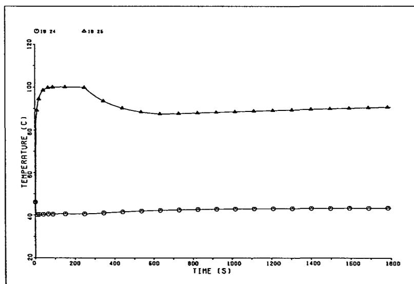
**Figure 6. Temperature in rooms IB24 and IB25 after MFLB in IB25**
