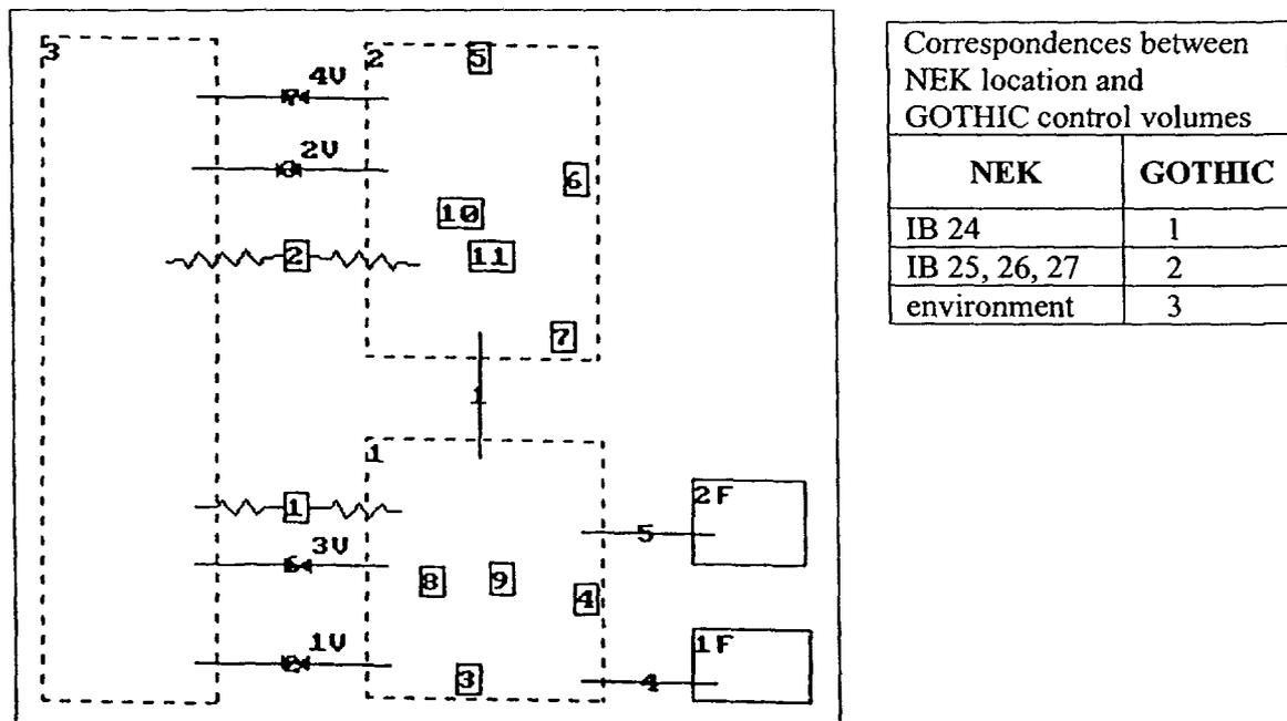
Figure 2. GOTHIC model for NEK IB at elevation 107.62
