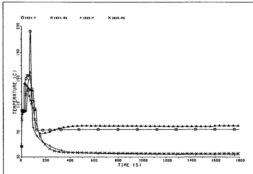
**Figure 5. Temperature in rooms IB24 and IB25 after MSLB in IB24; FSAR (-F) and RELAP5/mod2 (-R5) mass and energy source**
