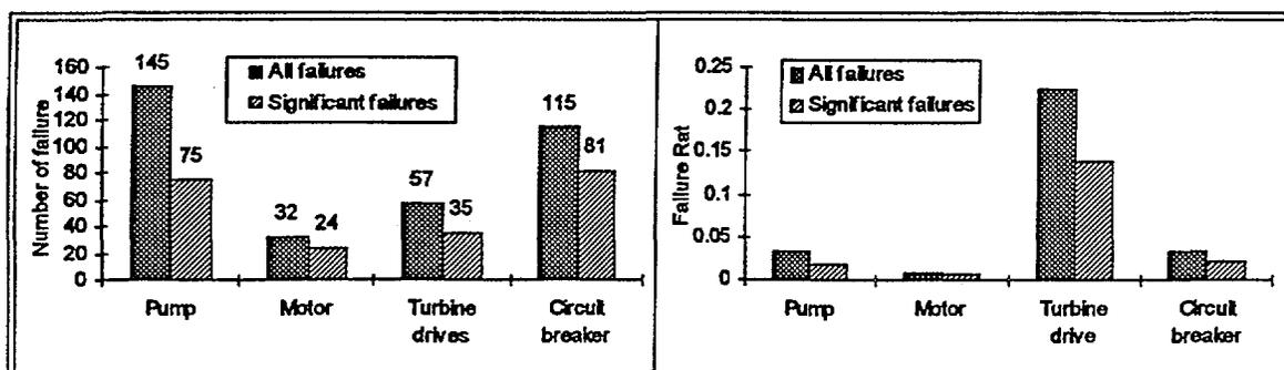
Fig. 1 Failure counts/rates for pumps, motors, turbine drives, and circuit breakers
