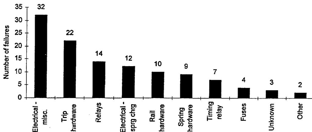
Fig. 3 Circuit breaker failures by affected area
