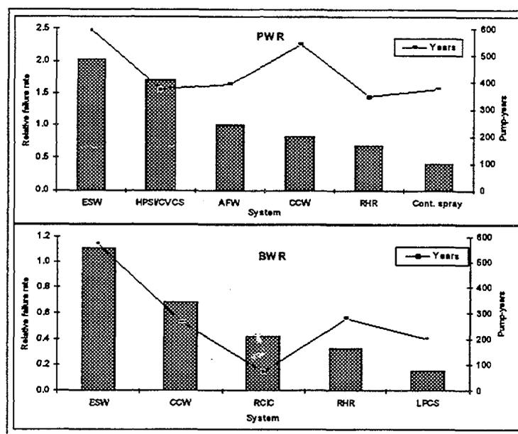
*Fig. 2 Distribution of failures by System - PWR & BWR*
