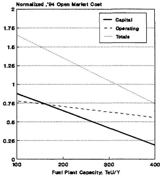
**FIGURE 2: FUEL MANUFACTURING COSTS TREND FULLY INTEGRATED FUEL PLANT (Dep. 16 Years, 10% Interest Rate)**
