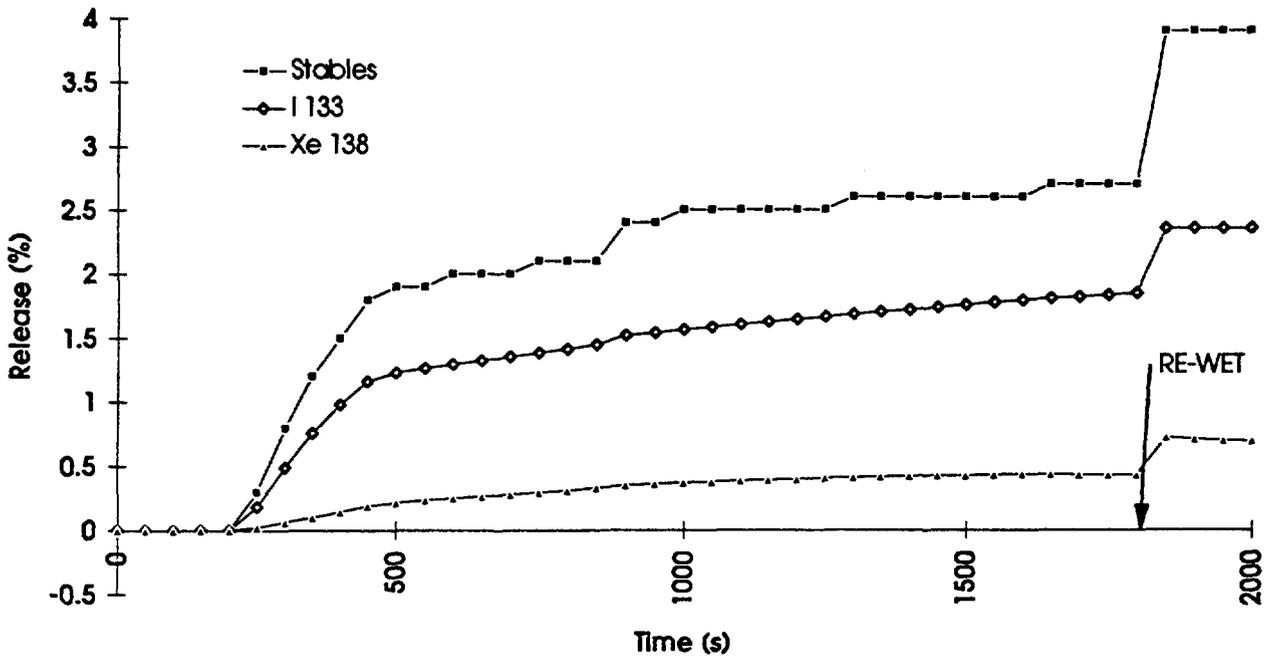
FIGURE 2 CALCULATED FP RELEASE DURING THIRD TRANSIENT
