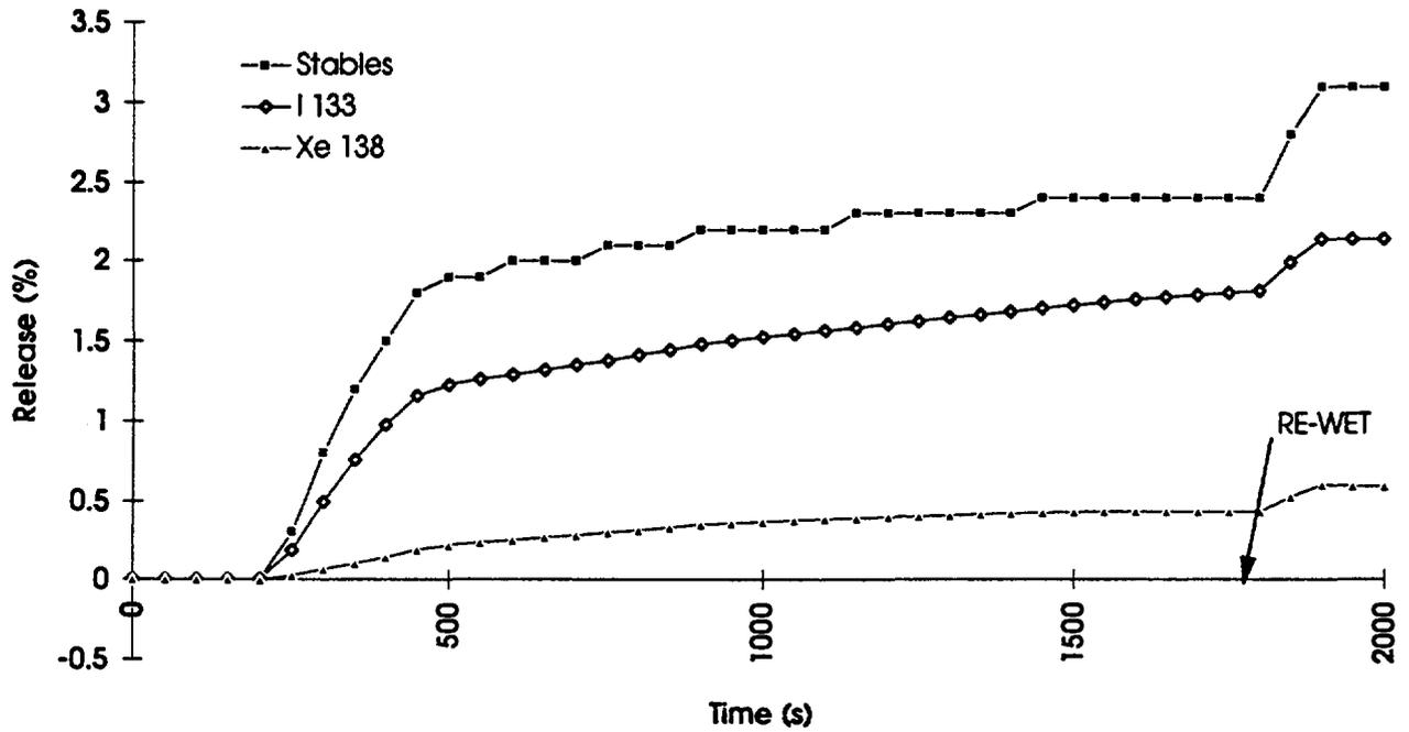
FIGURE 4 CALCULATED FP RELEASE DURING THIRD TRANSIENT WITH THERMAL STRESSES SUPPRESSED
