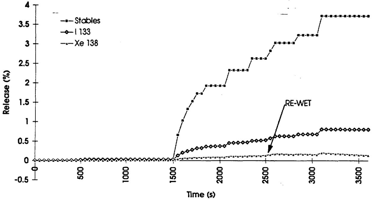
FIGURE 1 CALCULATED FP RELEASE DURING SECOND TRANSIENT
