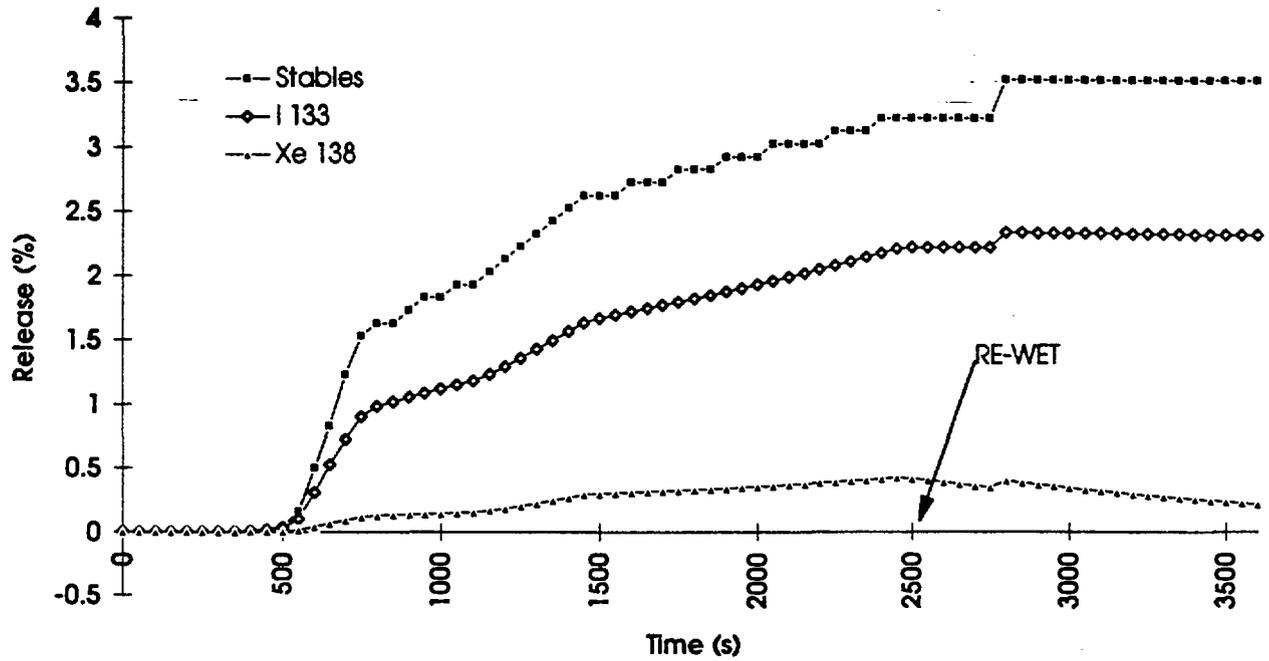
FIGURE 3 CALCULATED FP RELEASE DURING SECOND TRANSIENT WITH THERMAL STRESSES SUPPRESSED
