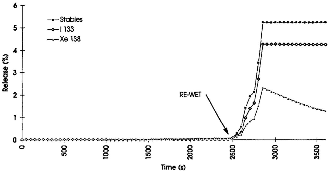
FIGURE 6 CALCULATED FP RELEASE DURING SECOND TRANSIENT, WITH INTERFACE PRESSURE TO PELLET CENTER AND RELOCATED BRIDGING ANNULUS
