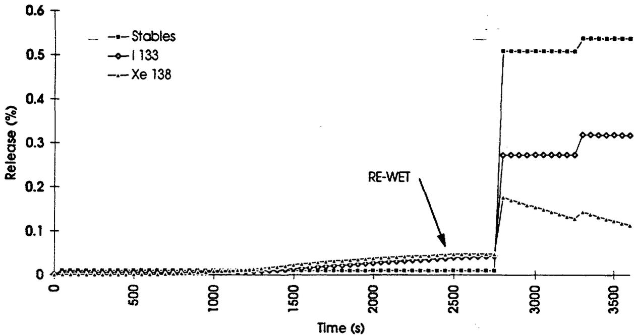
FIGURE 5 CALCULATED FP RELEASE DURING SECOND TRANSIENT, WITH INTERFACE PRESSURE TO PELLET CENTER
