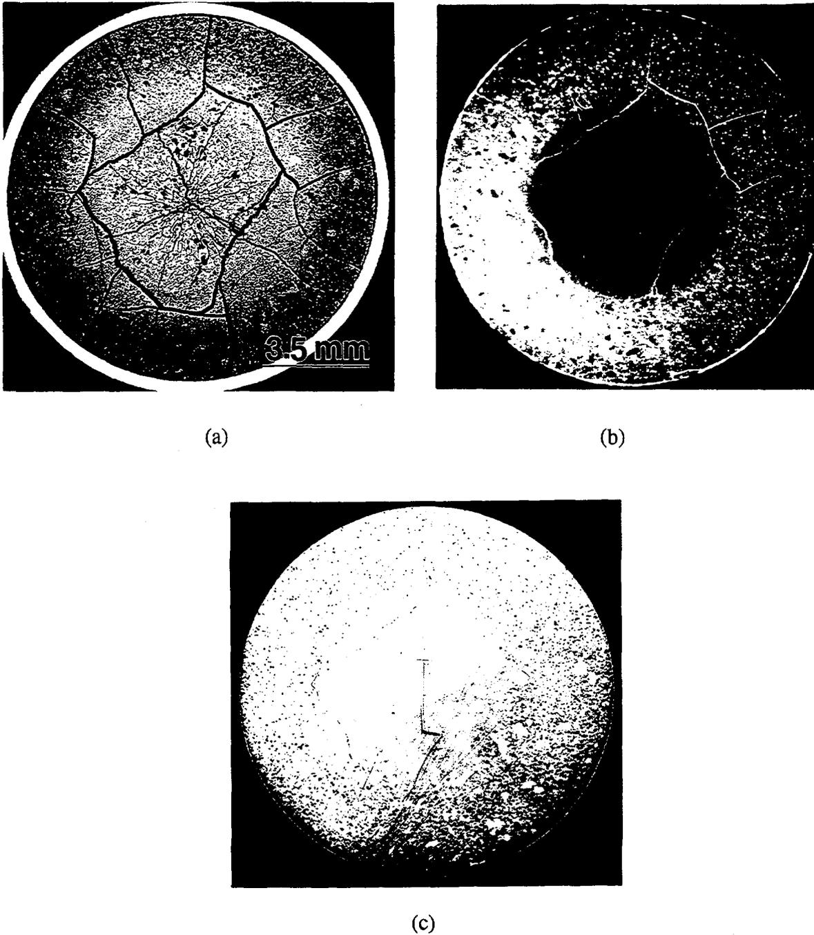
Figure 4. Outer element from bundle ABC: (a) macrograph showing fuel structure, (b)  $\beta/\gamma$  autoradiograph (white spots represent high fission-product regions and dark circle indicates fission-product depletion in the pellet centre), and (c)  $\alpha$  autoradiograph (dark spots represent Pu-rich regions; note the Pu homogenization region in the pellet centre).
