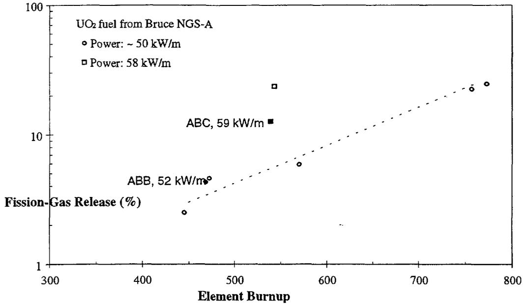
Figure 2. Fission-Gas Release versus Element Burnup for fuel experiencing declining power histories from beginning-of-life powers in the range of 50-59 kW/m (as shown).
