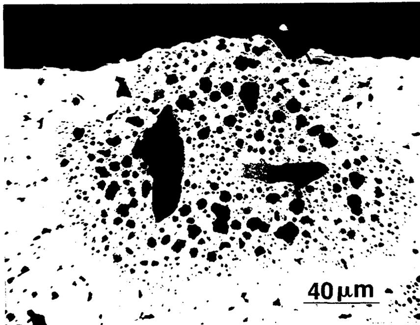
Figure 1. Microstructure of element KB-01 showing porous zone with metallic precipitates.
