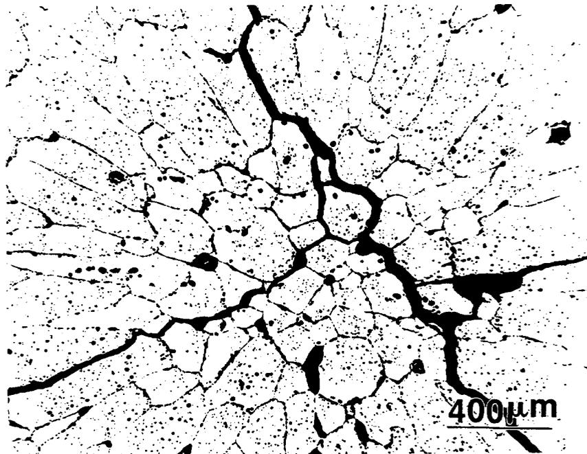
Figure 3. Micrograph showing grain morphology at pellet centre of an outer element from Bundle ABC. Note that the grains at pellet centres are larger than 100  $\mu\text{m}$ .
