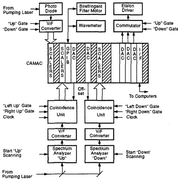
Figure 2. Laser Frequency and Power Control
