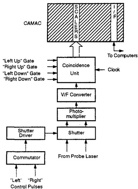
Figure 4. Laser Faraday Rotation Polarization Measurement.
