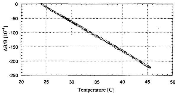
Figure 2: Magnetic field data under a slow thermal cycle for a NdFeB permanent dipole magnet. Temperature coefficient for the relative magnetic field in the air gap was  $(\Delta B/B)/\Delta T = -1.1 \times 10^{-3}/^\circ\text{C}$  in the temperature range of 25-35°C.
