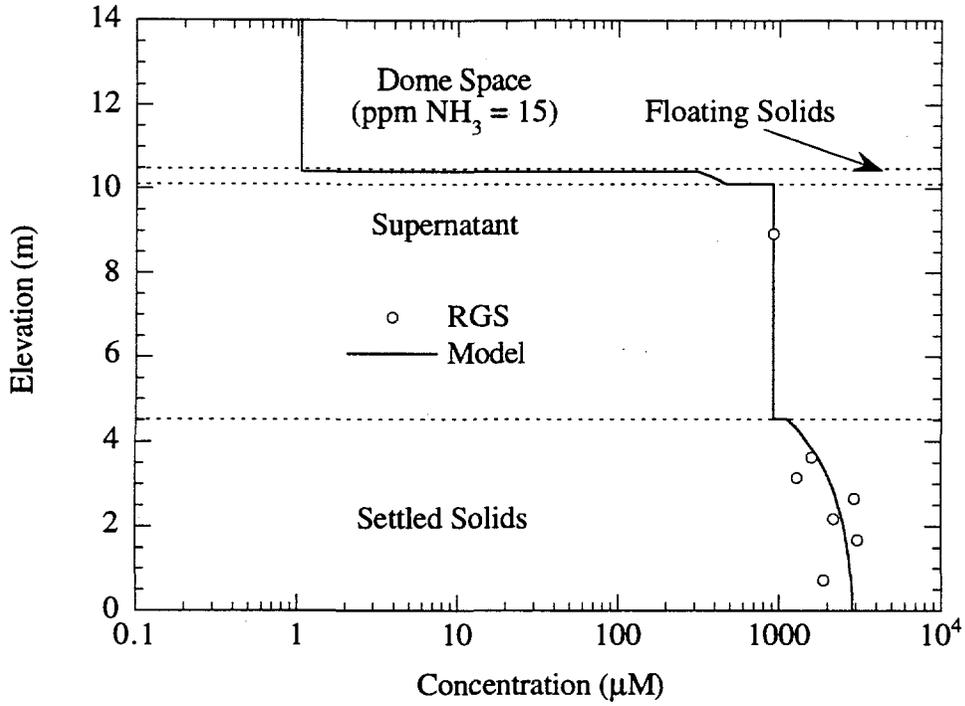
**Figure 3.6.** Ammonia Concentration Distribution in Tank AN-105 (model Eq. 2.1–2.8)
