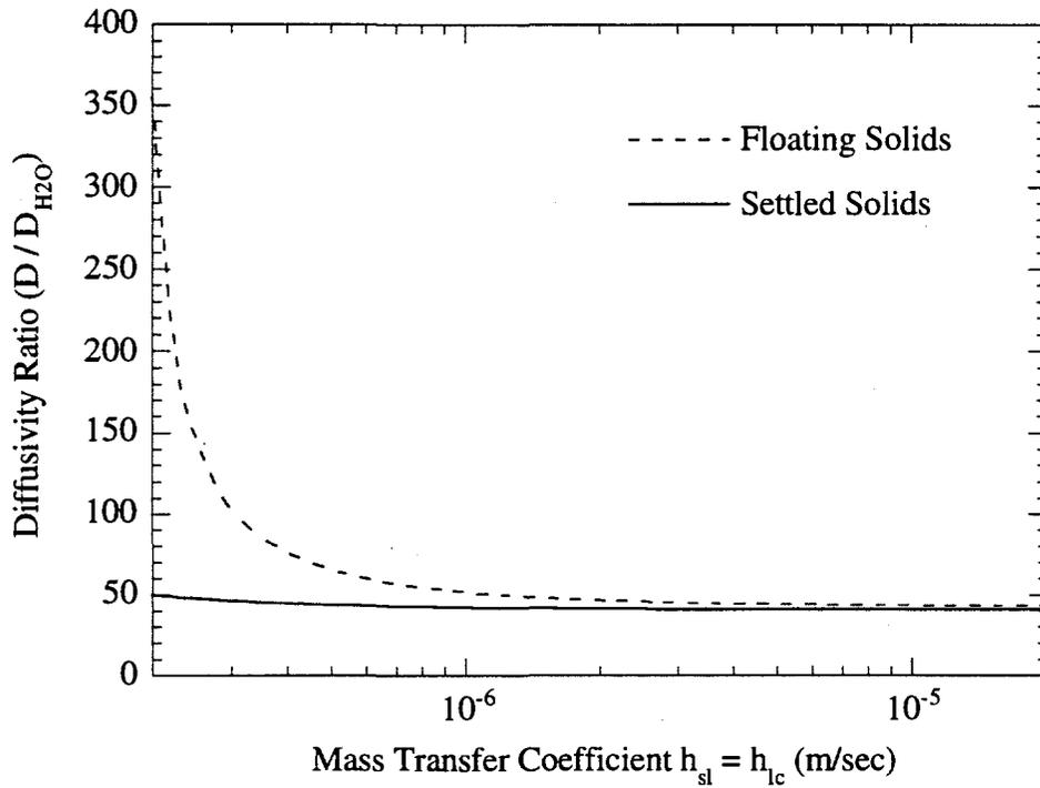
**Figure 3.7.** Diffusivity Ratios for Nonconvective Layers as a Function of the Mass Transfer Coefficient in Tank AN-105
