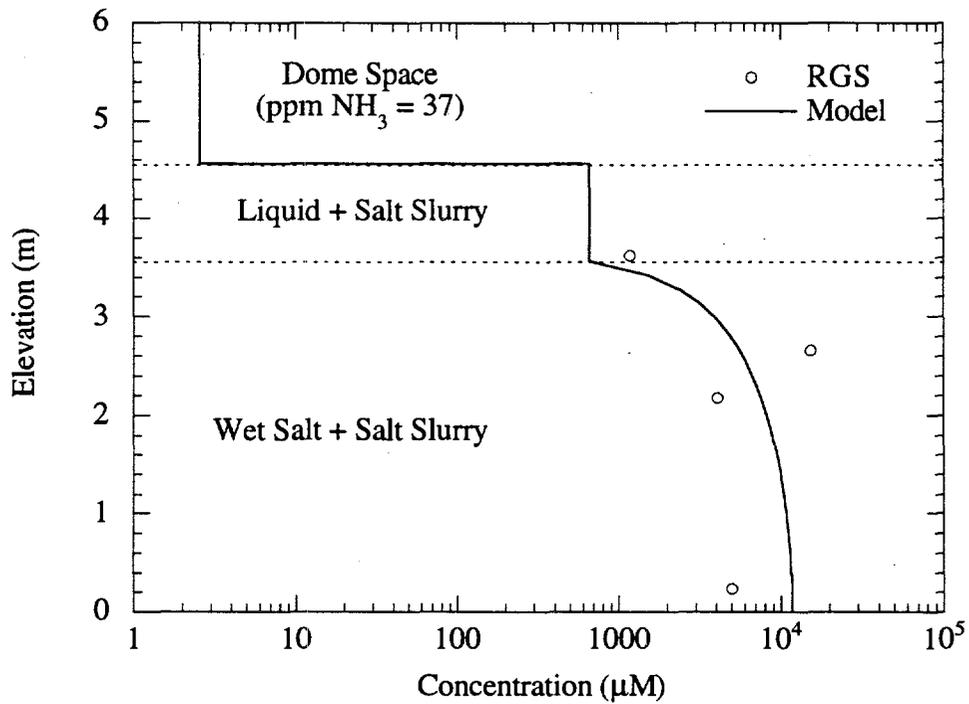
**Figure 3.11.** Ammonia Concentration Distribution in Tank S-106 (model Eq. 2.14–2.18)
