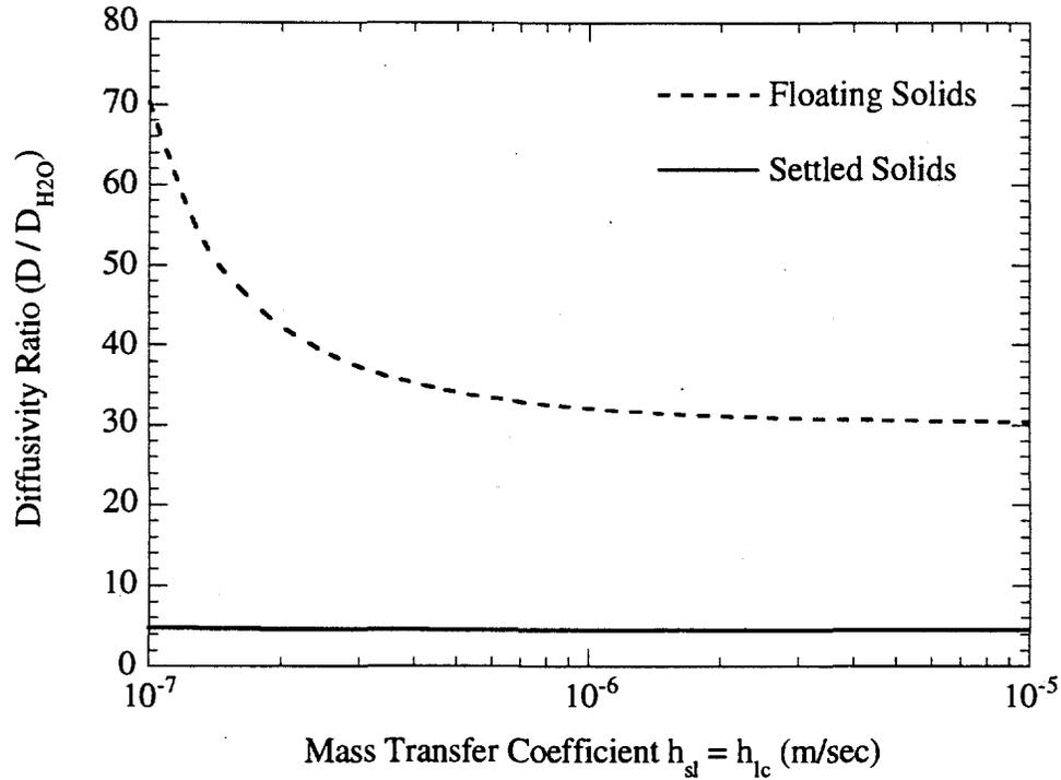
**Figure 3.3.** Diffusivity Ratios for Nonconvective Layers as a Function of the Mass Transfer Coefficient in Tank AW-101
