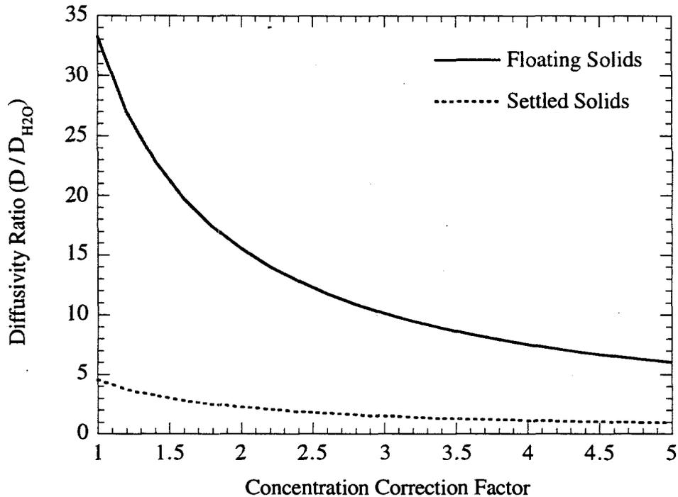
**Figure 3.2.** Diffusivity Ratios for Nonconvective Layers as a Function of the Concentration Correction Factor in Tank AW-101
