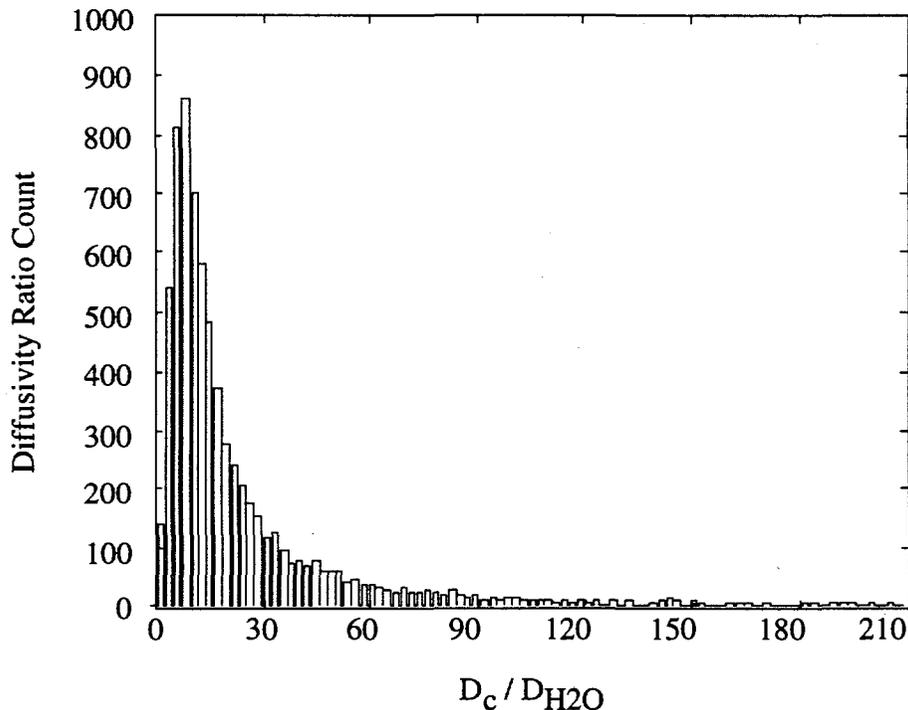
**Figure D.1.** Distribution of the Diffusivity Ratios for the Floating Solids Layer in Tank AW-101
