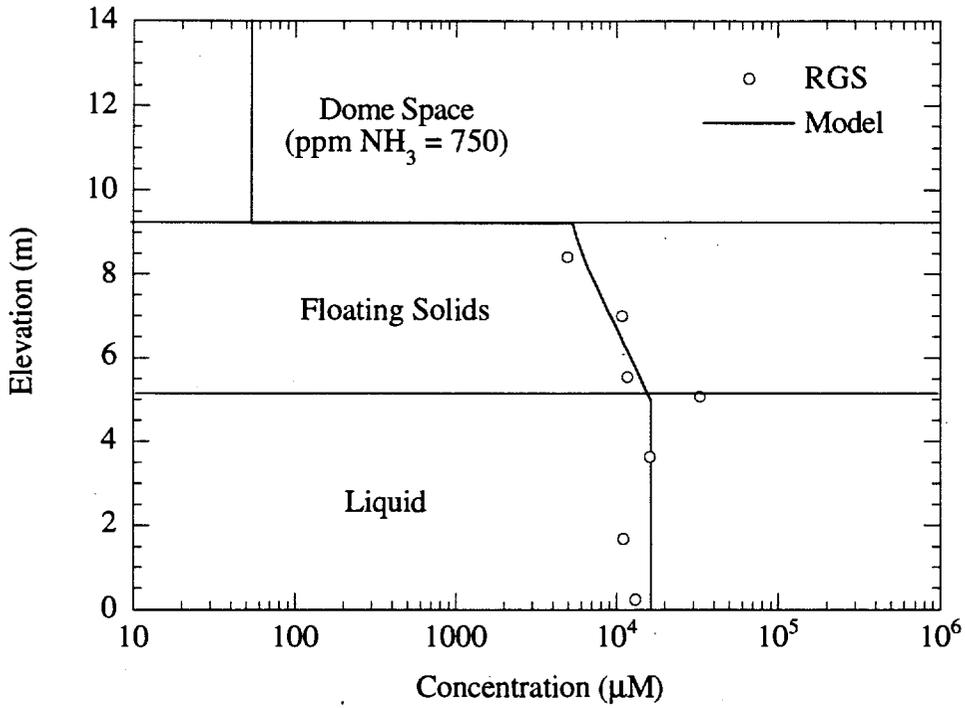
Figure 3.9. Ammonia Concentration Distribution in Tank A-101 (model Eq. 2.9–2.13)
