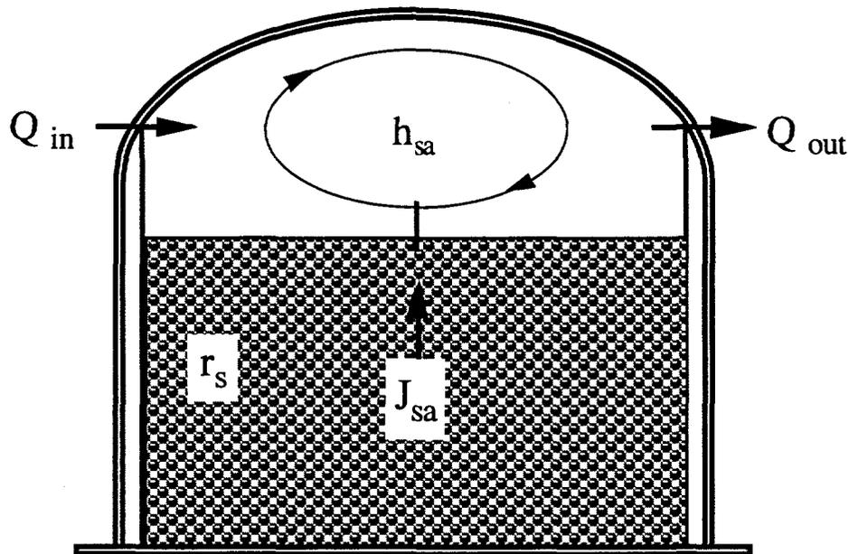
**Figure 2.4.** Schematic Diagram for the Nonconvective Liquid-Slurry Waste Configuration in Tank U-103
