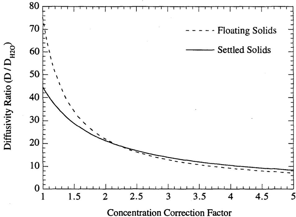
**Figure 3.8.** Diffusivity Ratios for Nonconvective Layers as a Function of the Concentration Correction Factor in Tank AN-105
