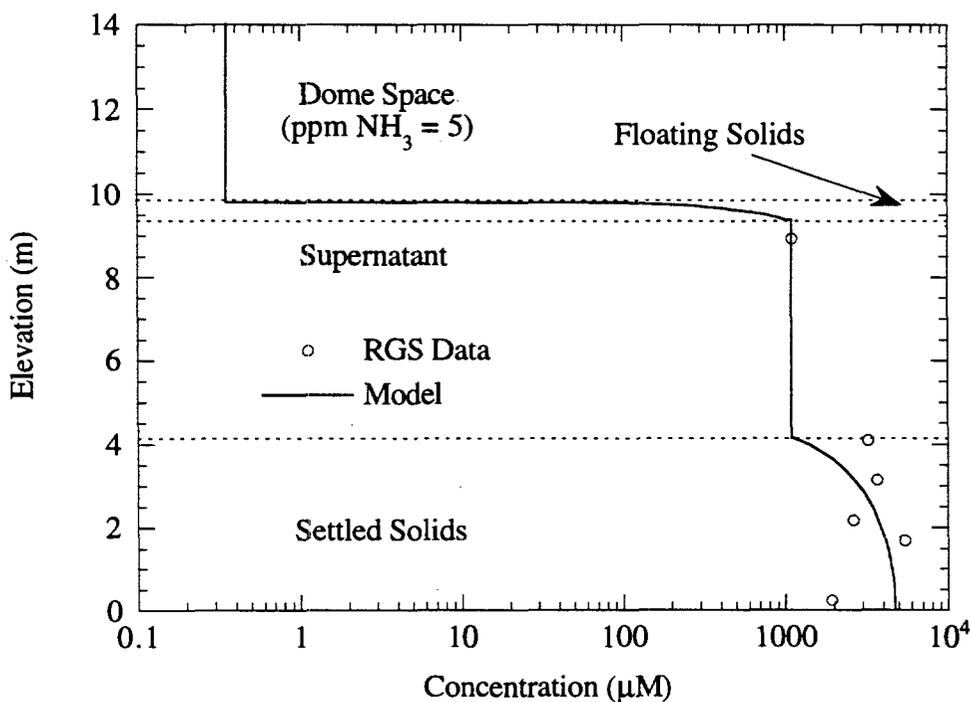
Figure 3.5. Ammonia Concentration Distribution in Tank AN-104 (model Eq. 2.1–2.8)
