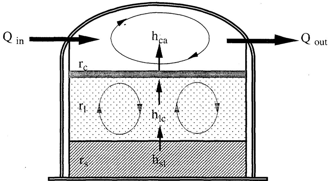
**Figure 2.1.** Schematic Diagram for the Settled Solids-Supernatant-Floating Solids Waste Configuration in Tanks AW-101, AN-103, AN-104, and AN-105
