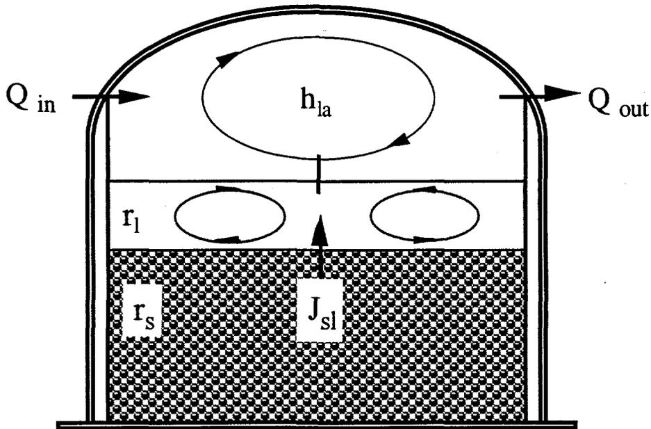
**Figure 2.3.** Schematic Diagram for the Liquid-Slurry Waste Configuration in Tank S-106
