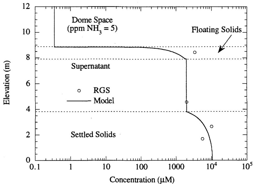
**Figure 3.4.** Ammonia Concentration Distribution in Tank AN-103 (model Eq. 2.1–2.8)
