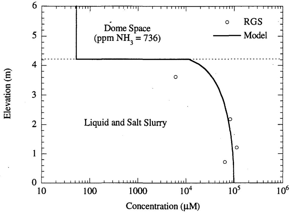
**Figure 3.12.** Ammonia Concentration Distribution in Tank U-103 (model Eq. 2.19–2.22)
