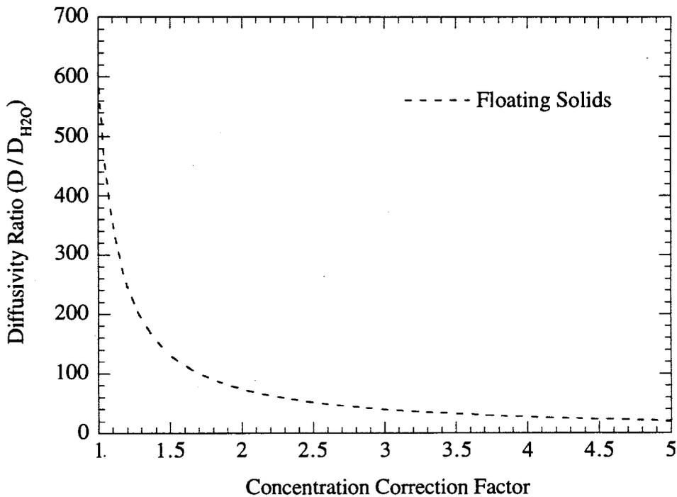
Figure 3.10. Diffusivity Ratio for the Floating Solids Layer as a Function of the Concentration Correction Factor in Tank A-101
