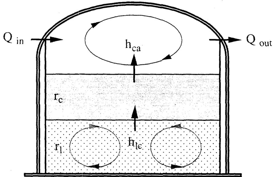
**Figure 2.2.** Schematic Diagram of the Liquid-Floating Solids Waste Configuration in Tank A-101
