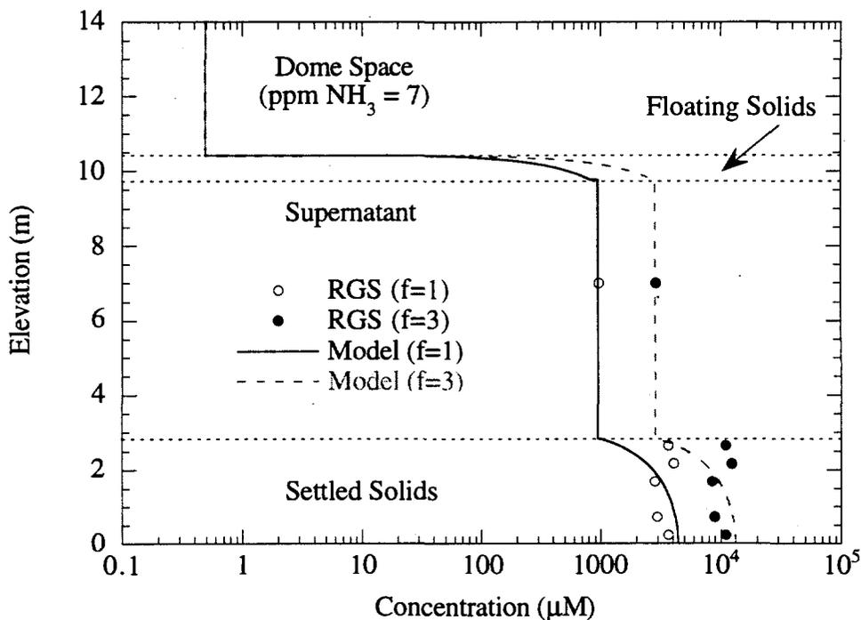
Figure 3.1. Ammonia Concentration Distribution in Tank AW-101 (model Eq. 2.1–2.8)
