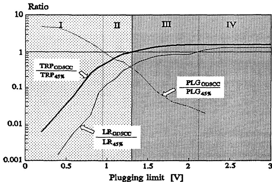
Figure 2 The efficiency of ODSCC specific maintenance (Krško NPP, SG1, 1993)
