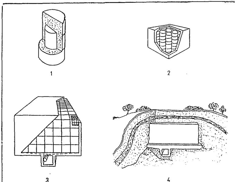
**Fig.2. Successive barriers in the surface-type final disposal system**
