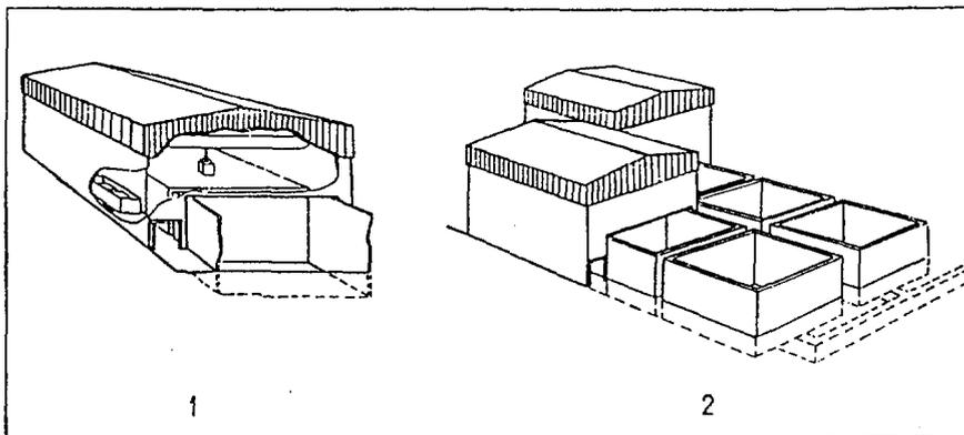
**Fig. 4. Final disposal units with sliding roof structure**
