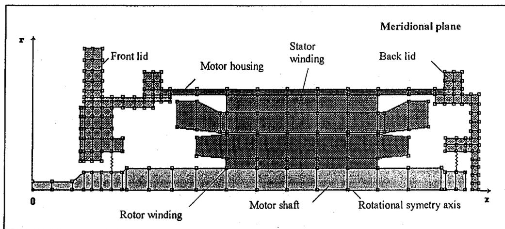
Figure 2. 3D Modeling of small low voltage electric motor
