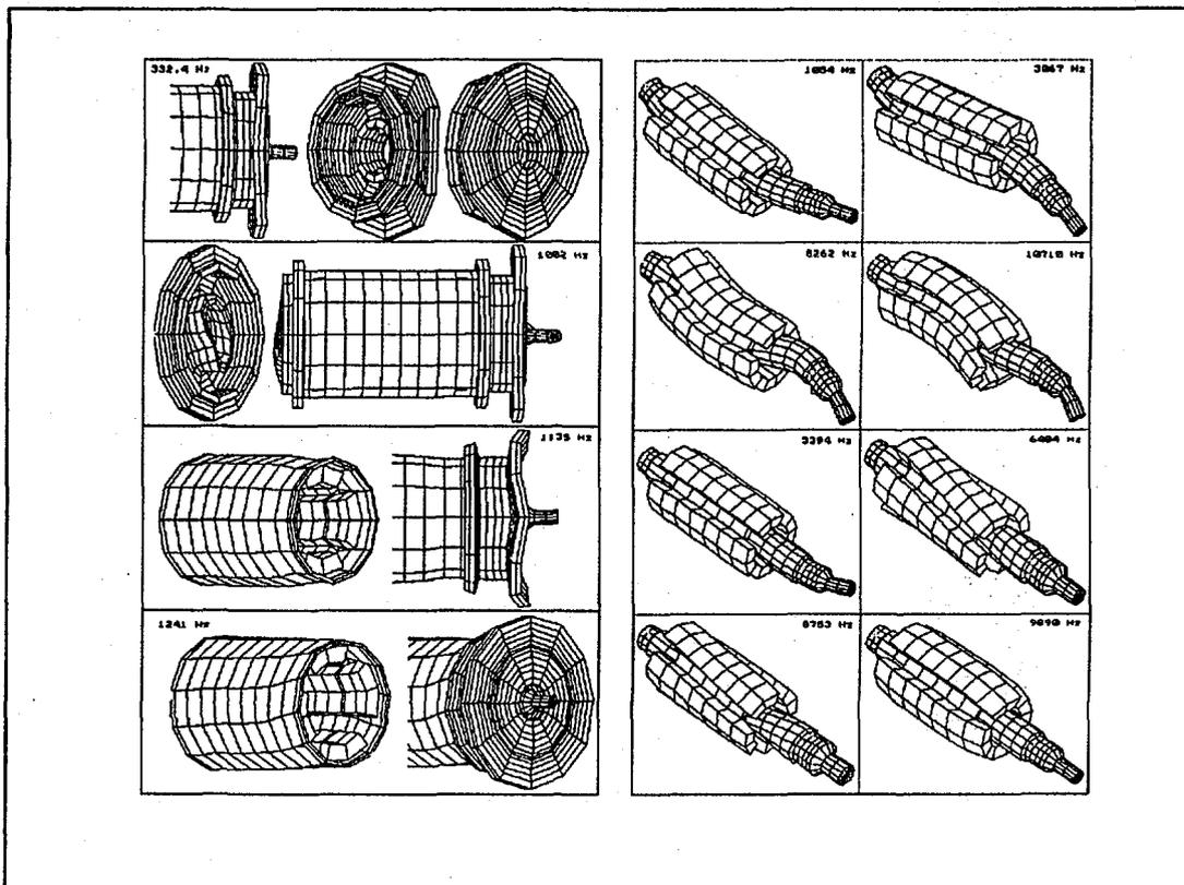
**Figure 3.** a) The first four mode shapes of the casing: 332/1002/1135/1241 Hz.
