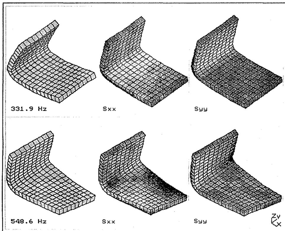
**Figure 1.** The first two resonant frequencies, mode shapes and modal  $S_{xx}$  and  $S_{yy}$  stresses of L-shaped electric motor carrier (253 3D-finite elements).
